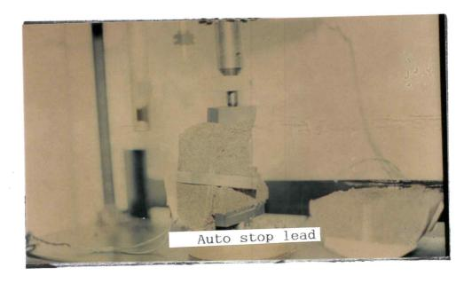
Figure 5.20. Failed specimen which results in breaking of foil tape and stopping the test.
