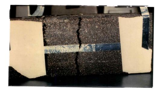
Figure 6.6. Cracked beam which broke the foil tape and stopped the test.
