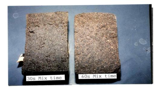
Figure 4.11. Effect of mixing time on dune sand emulsion.
