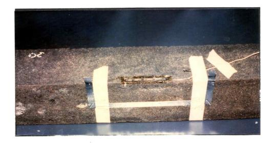
Figure 6.5. Beam ready for fatigue test with SR-4 strain gage attached to the side and foil tape attached to the bottom.
