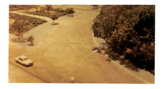
Figure 2.19. Light blue asphalt emulsion used for sidewalk treatment. "JEDDAH"
