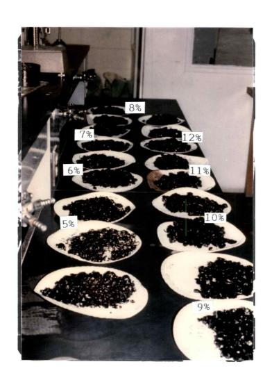
Figure 4.8. Open graded asphalt emulsion mix trials showing different emulsion contents (water content varied from 0-2%).
