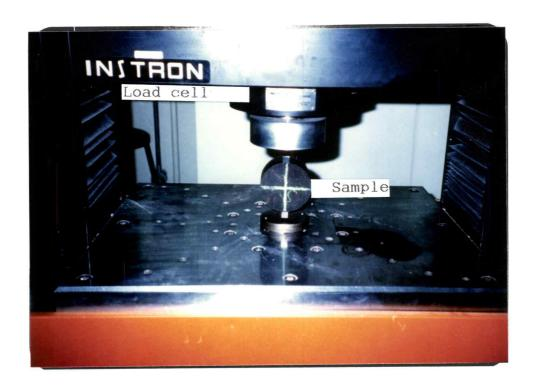
Figure 5.4. Test set up for determining tensile strength.
