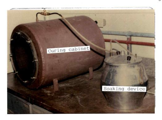
Figure 4.10. Vacuum curing cabinet and soaking device.
