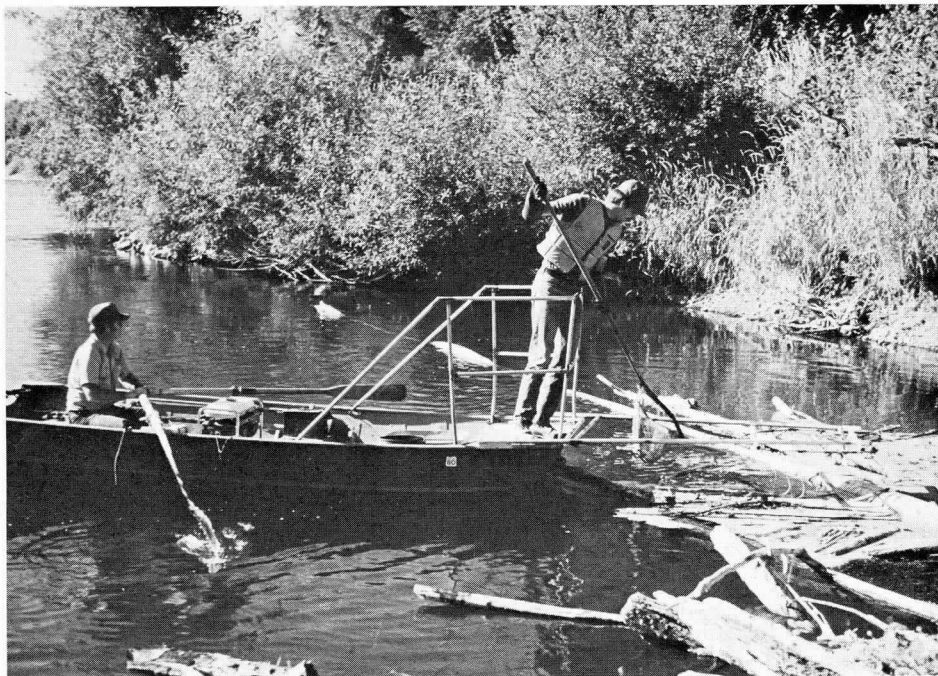
Fairly new to the warm-water fish management scene, electrofishing equipment provides an excellent method for sampling fish populations. An electric current stuns fish but causes no permanent damage.
