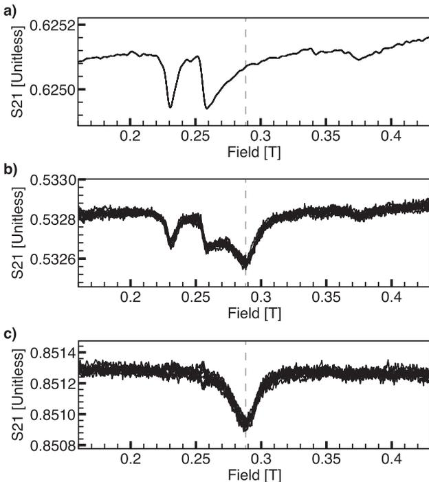
FIG. 2. A comparison of measured  $|S_{21}|$  of a bare substrate after resampling and smoothing (a), substrate with a MgO/CoFeB (0.9 nm)/Ta/CoFeB (0.9 nm)/MgO stack (b), and results after de-embedding (c). Measurements were taken with a 19 GHz excitation.
