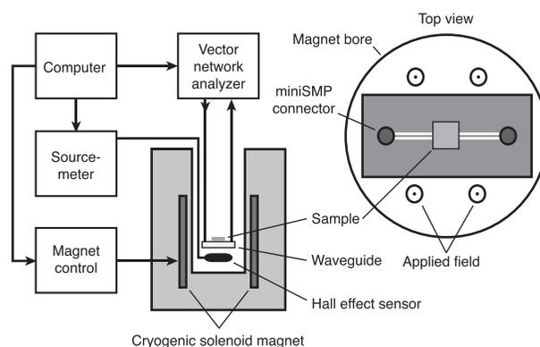
FIG. 1. Schematic of a cross section and top view of the measurement system. The waveguide and sample are placed in the bore of a Cryogenic Limited superconducting magnet, which creates a magnetic field out of the plane of the sample. The magnetic field is monitored using a Hall effect sensor and Keithley 2440 Sourcemeter. An Agilent E5224A PNA is used to measure the  $S$ -parameters of the coplanar waveguide.
