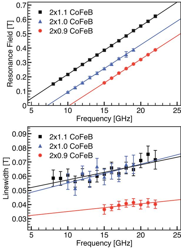
FIG. 5. Measured FMR linewidth and resonance field with 95% confidence intervals for samples presented in Table I.
