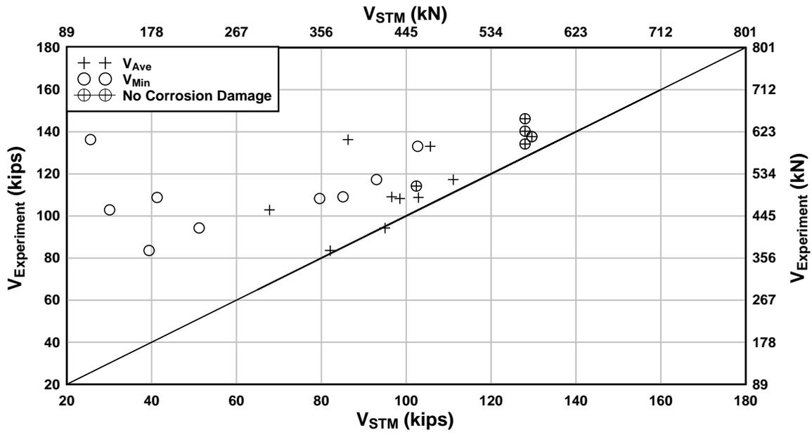
Fig. 5 – Experimental and analytical prediction of shear capacity from STM model
