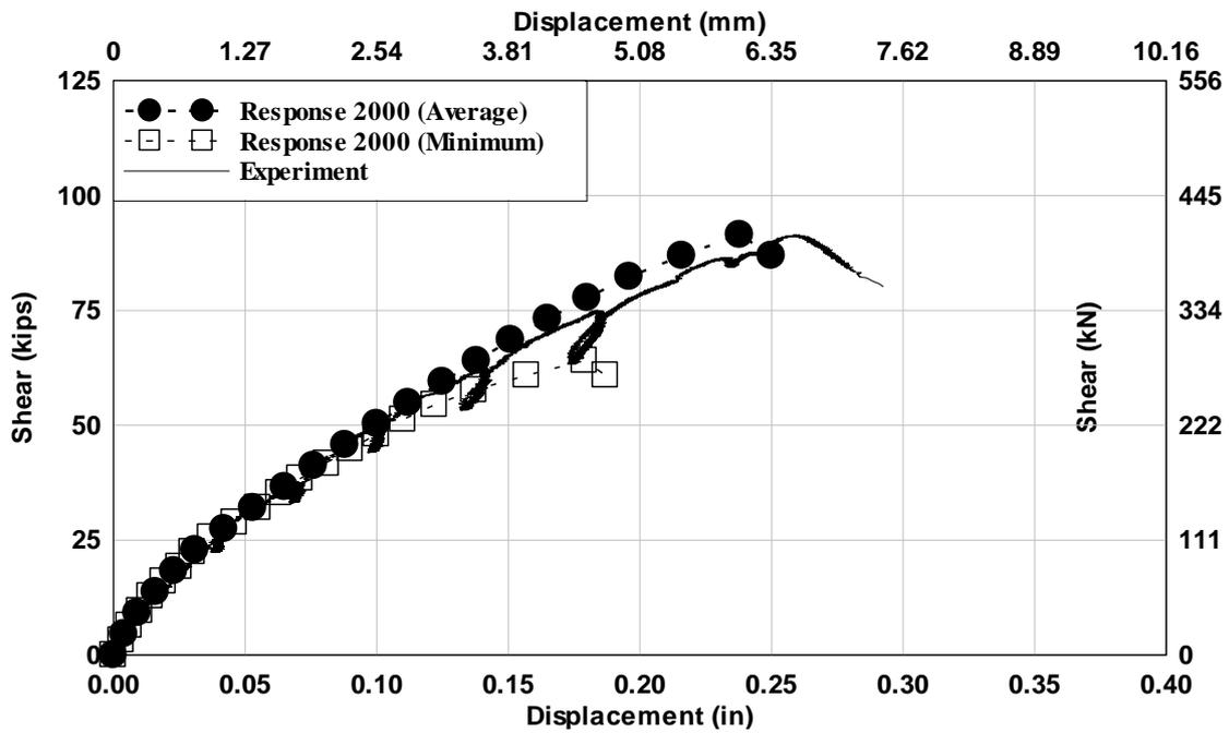
Fig. 8 – Experimental and analytical prediction of shear capacity from Response 2000, specimen 10RD.
