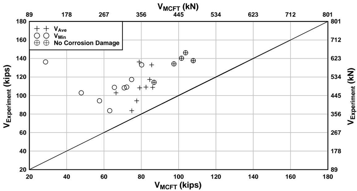
Fig. 6 – Experimental and analytical prediction of shear capacity from MCFT
