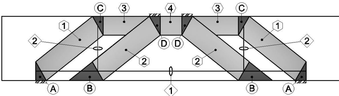
Fig. 4 – Strut-and-Tie model.
