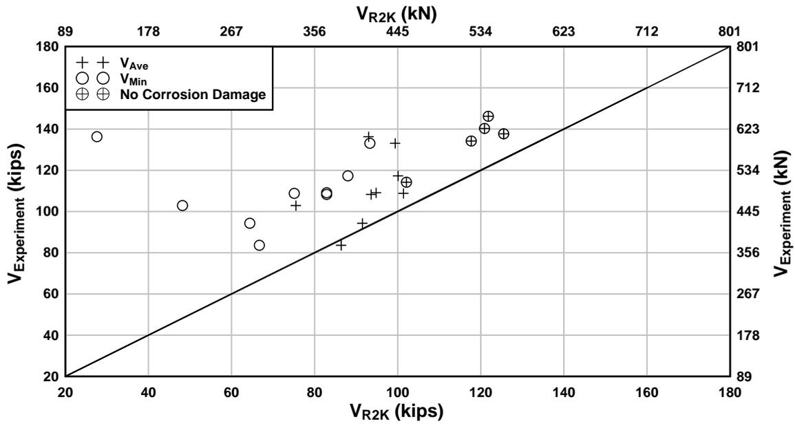
Fig. 7 – Experimental and analytical prediction of shear capacity from Response 2000.
