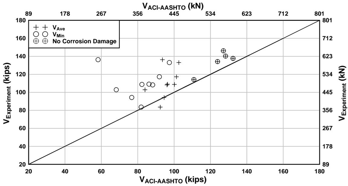
Fig. 3 – Ratio of experimental to predicted shear strengths for ACI-AASHTO approach including corrosion damage.
