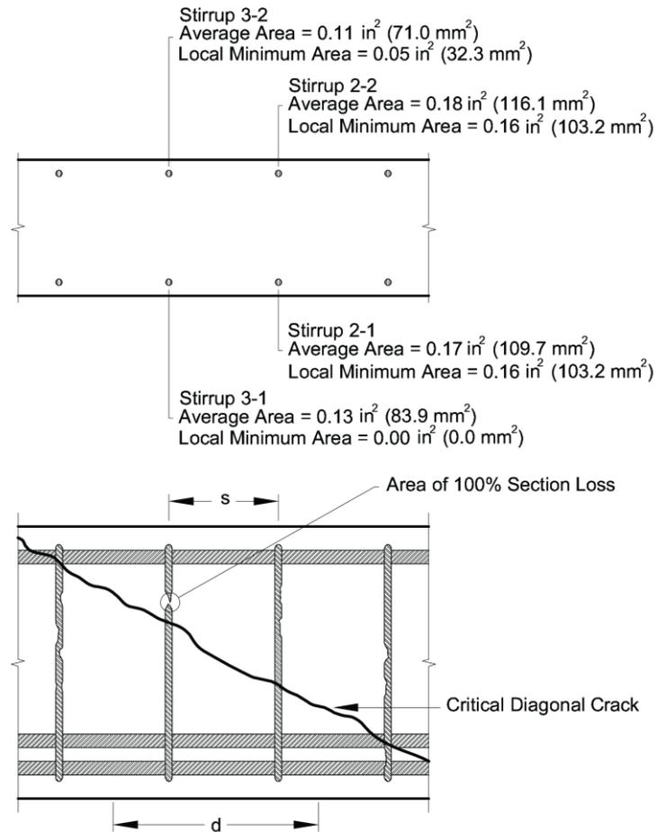
**Fig. 1 – Average and local maximum section-loss of stirrups within a length of beam.**
