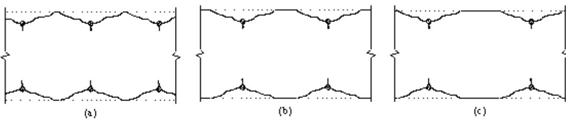
**Fig. 2 – Plan view of concrete cracking in beam web due to corrosion for three different stirrup spacing; (a) 8-in (203 mm), (b) 10-in (254 mm), and (c) 12-in (305 mm).**
