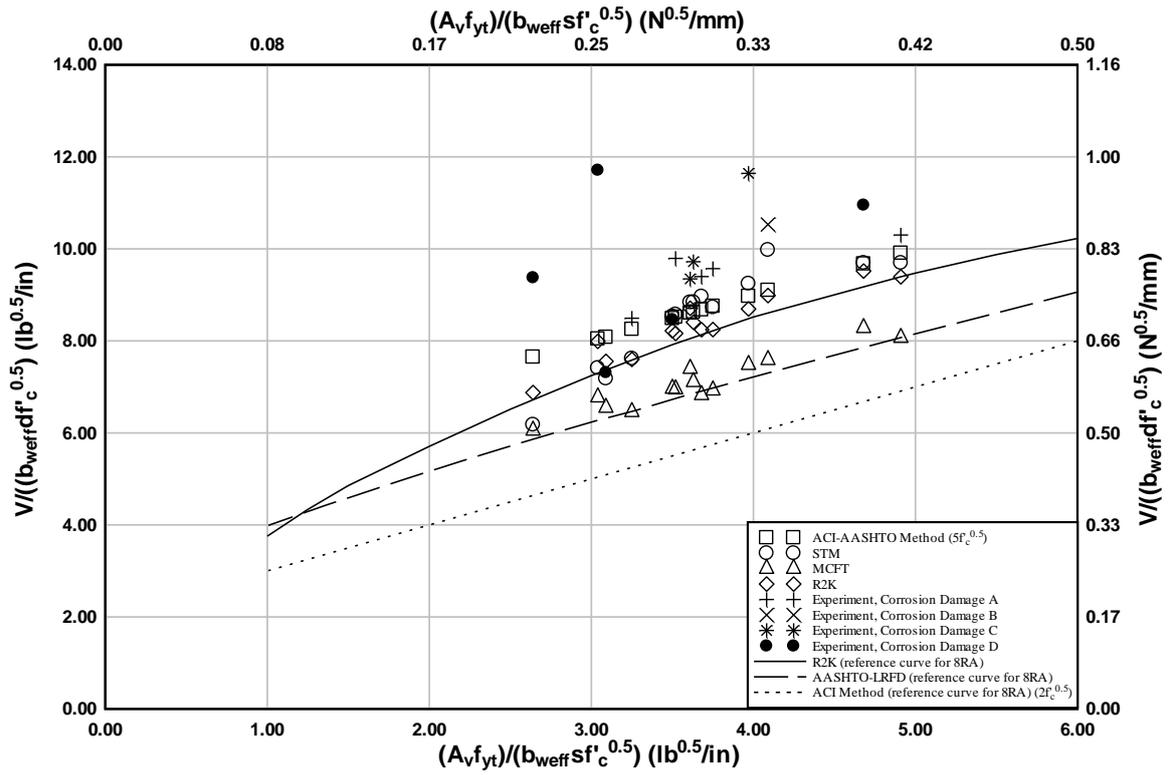
Fig. 9 – Normalized shear strength versus normalized stirrup quantity of all specimens.
