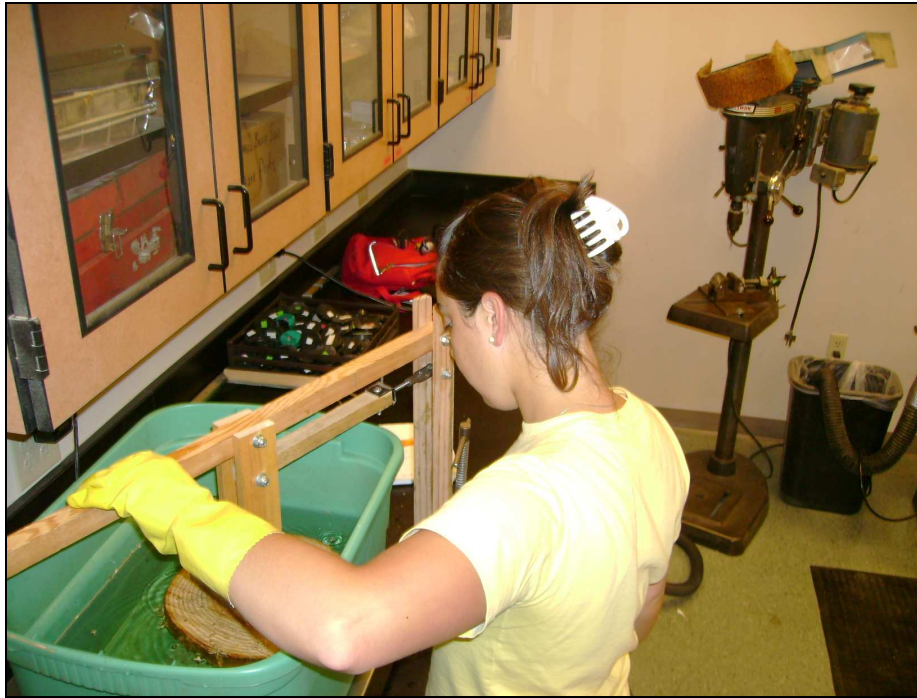
Figure 5. Dry density measurement using water displacement method.
