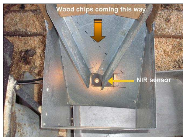
Figure 4. Top panel: wood chips path. Bottom panel: view of the collector from above.
