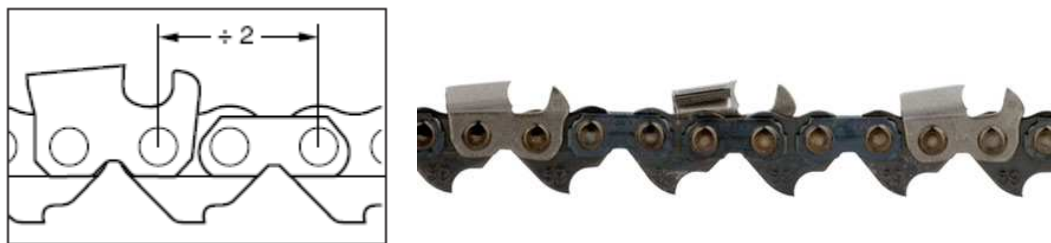
Figure 3. a) Chain pitch, b) picture of 0.404” pitch chain (Source: Mechanical Timber Harvesting Handbook, Oregon Cutting Systems Group Blount Inc.)
