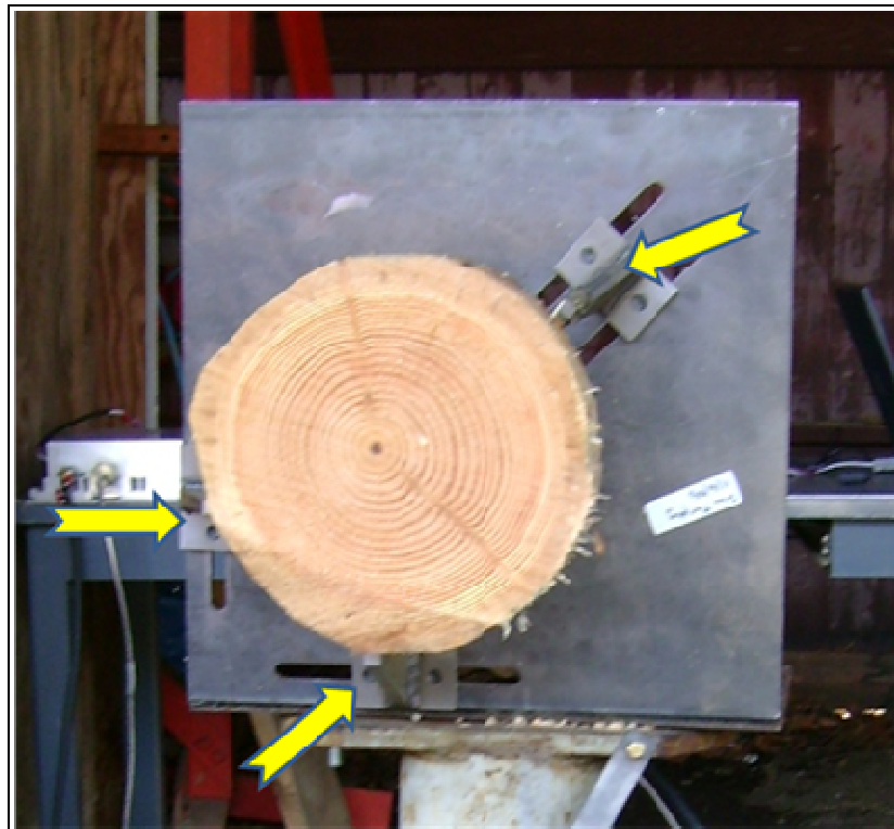
Figure 2. Wood sample holder, arrows indicate adjustable holding pins.
