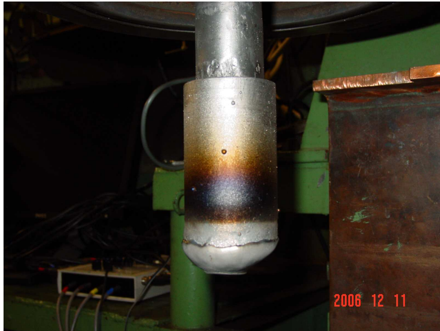
Figure 27: The leftover electrode after the 4-inch In 625 melt #2. Note more material melted off in the direction of the bus bar (and sensor 2).
