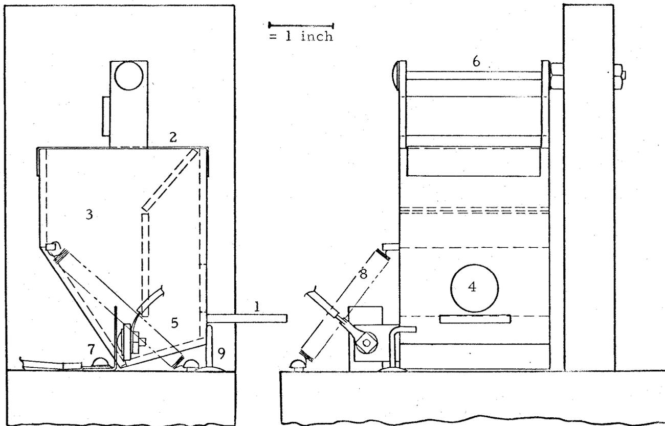
Figure 1. Mechanical electrical-recording feeder. See text for explanation.
