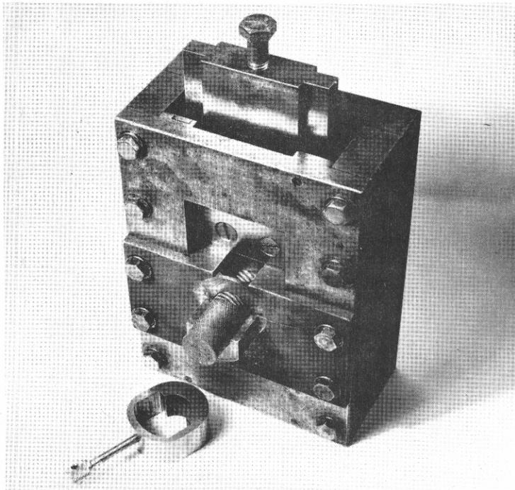
Figure 6. --Modified shear tool for testing glue joints in cylindrical plugs. A device for holding the specimen securely in place during test is shown in front of the tool.
