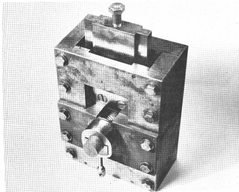
Figure 7. --Modified shear tool with plug-holding device in place and specimen ready for testing.
