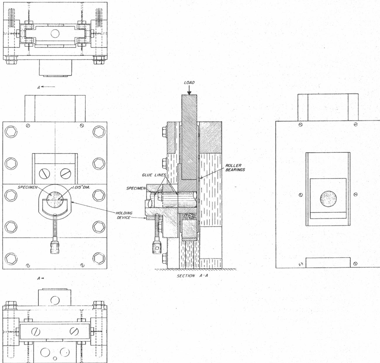
Figure 8. --Modified glue-block shear tool for shear testing glue joints in cylindrical specimens.
