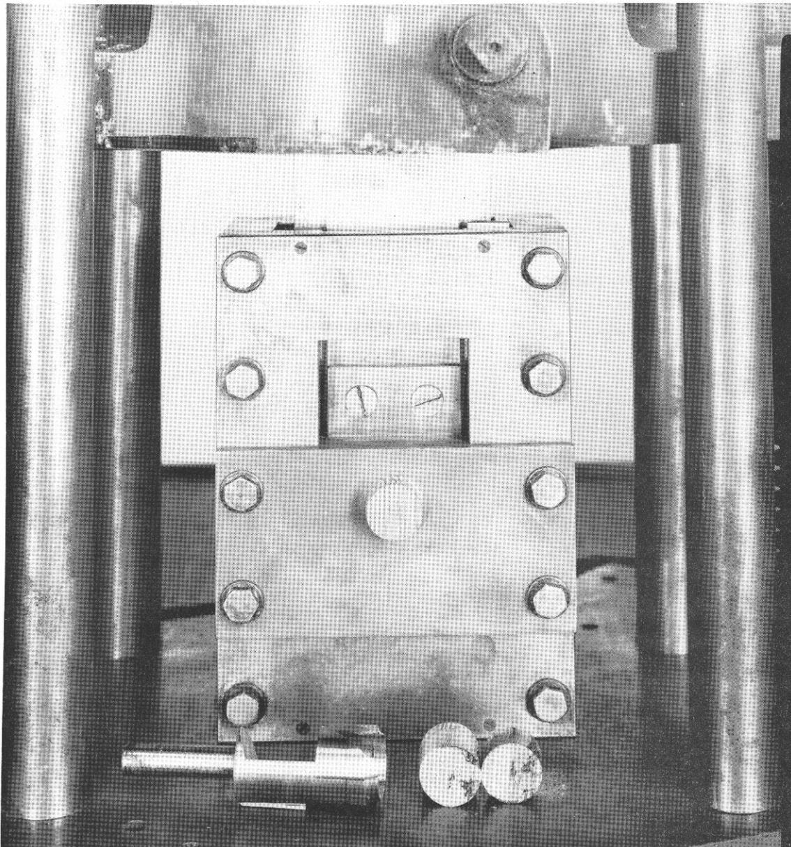
Figure 2. --Shear tool with cylindrical specimen inserted for testing.
