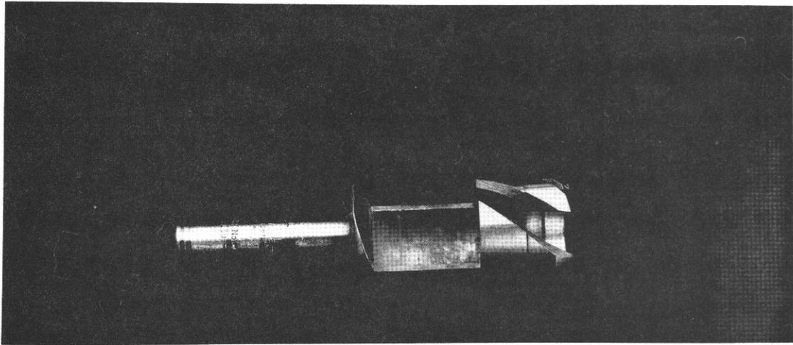
Figure 3. --Cutter for making 1-inch cylindrical plugs about 2 inches long.
