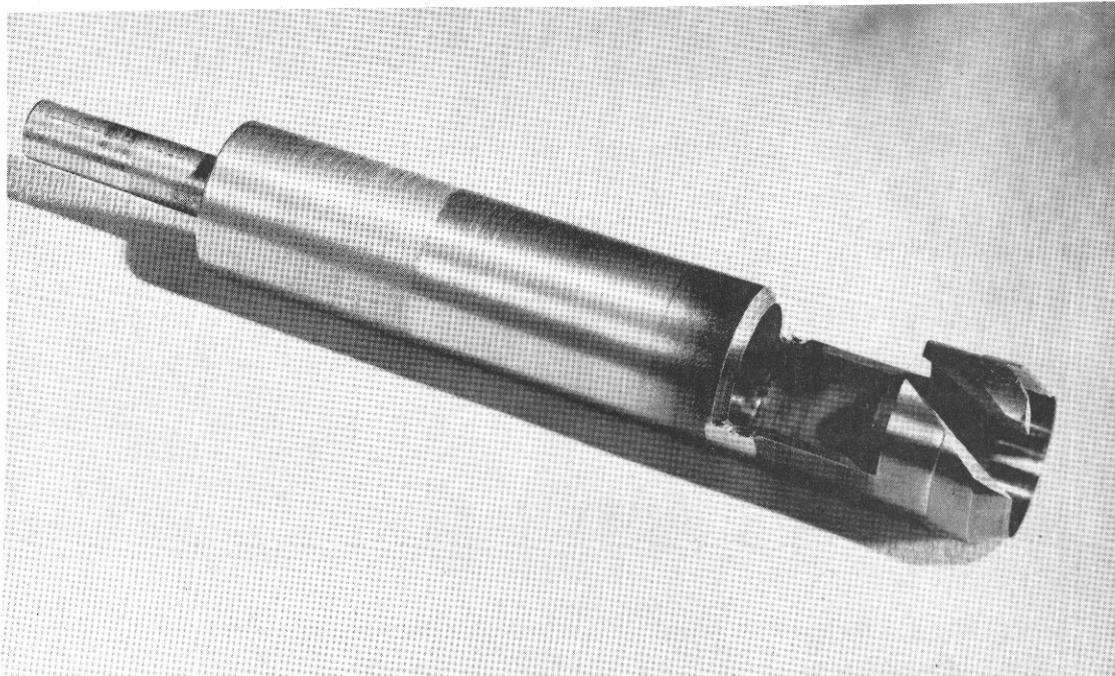
Figure 4. --Cutter after extension was added so plugs 4 to 5 inches in length could be cut.
