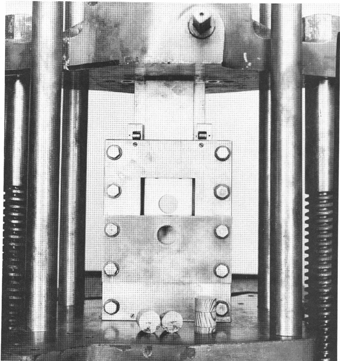
Figure 1. --Front view of shear tool for testing cylindrical specimens.
