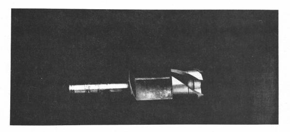
Figure 3. --Cutter for making 1-inch cylindrical plugs about 2 inches long.
