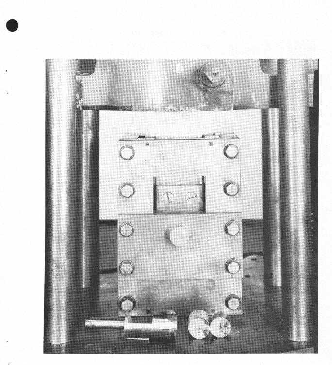
Figure 2. --Shear tool with cylindrical specimen inserted for testing. A broken specimen and a plug cutter are shown at the base of the tool.
