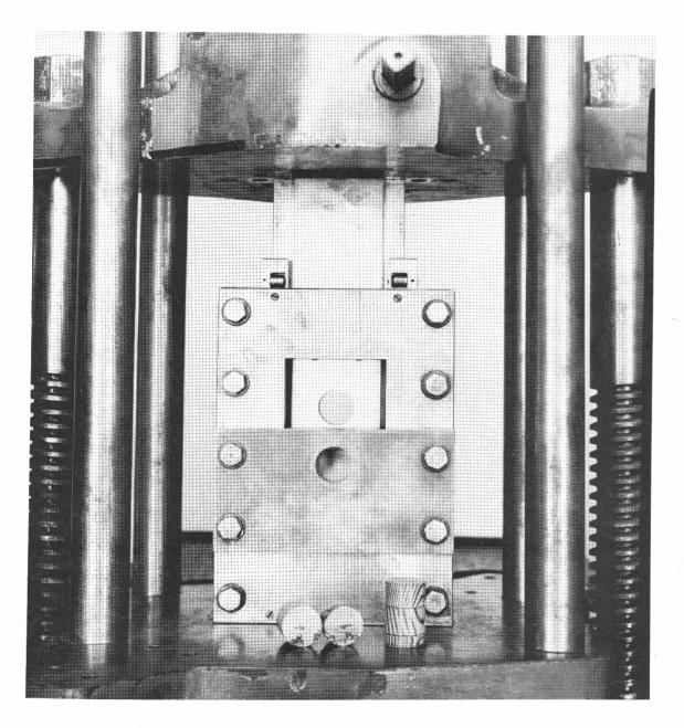
Figure 1. --Front view of shear tool for testing cylindrical specimens. The two cylindrical holes must coincide before specimen can be inserted.
