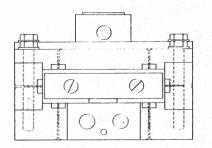
Figure 8. --Modified glue-block shear tool for shear testing glue joints in cylindrical specimens.
