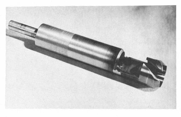
Figure 4. --Cutter after extension was added so plugs 4 to 5 inches in length could be cut.
