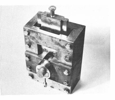
Figure 7. -- Modified shear tool with plug-holding device in place and specimen ready for testing.
