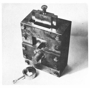
Figure 6.--Modified shear tool for testing glue joints in cylindrical plugs. A device for holding the specimen securely in place during test is shown in front of the tool.
