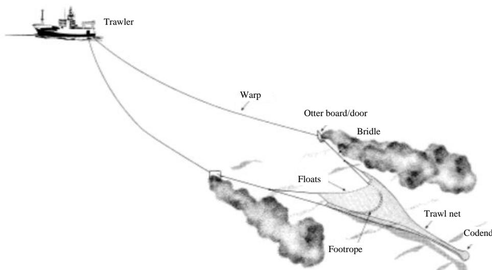
Figure 1.1: The configuration of a bottom trawl. In the context of NMFS survey sampling, the poly Nor'eastern nets had larger diameter footrope with roller bobbins when compared to the Aberdeen nets. Modified from FOOCG 2001. A Fishing Industry Guide to Offshore Operators.
