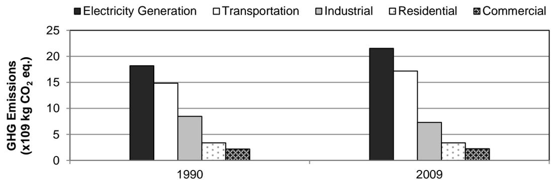
**Figure 1.2:** GHG Emissions Resulting from Fossil Fuel Combustion in the United States within Various Sectors, 1999 and 2009 (U.S. EIA, 2004)
