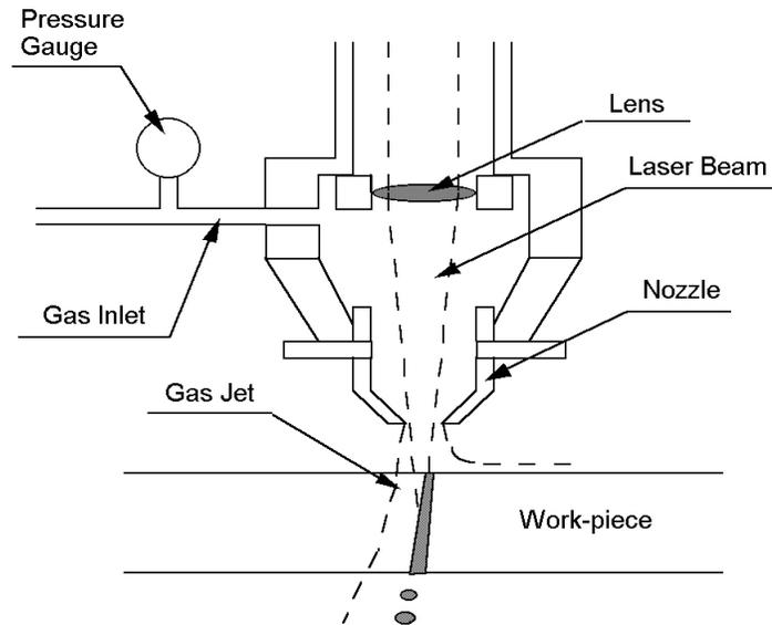
**Figure 3.10:** Gas Jet Laser Cutting (Chen et al., 2000)
