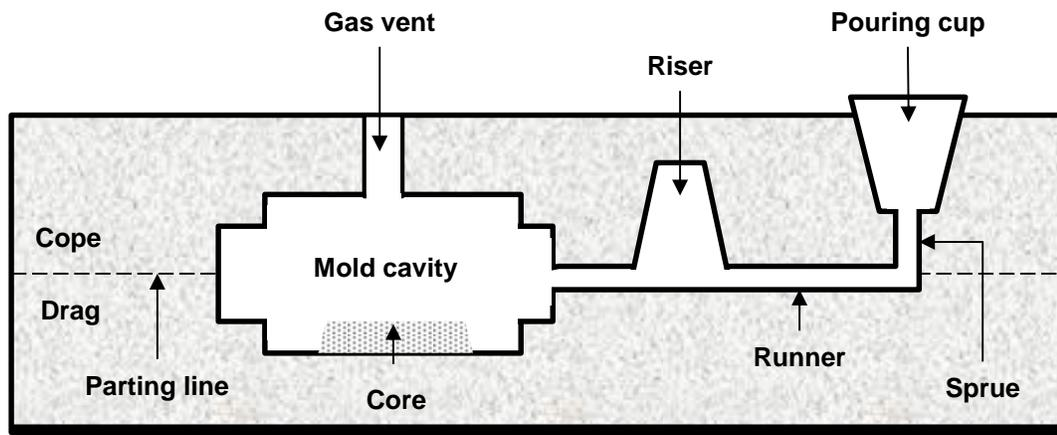
**Figure 3.4:** Mold for Sand Casting (adapted from [www.substech.com/](http://www.substech.com/))
