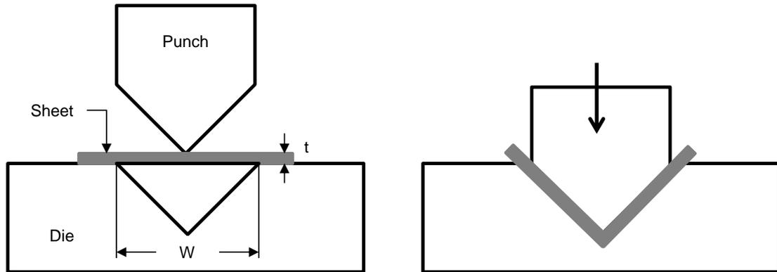
**Figure 3.7:** Illustration of Bending Process in a Sheet Metal (adapted from Lange, 1985)
