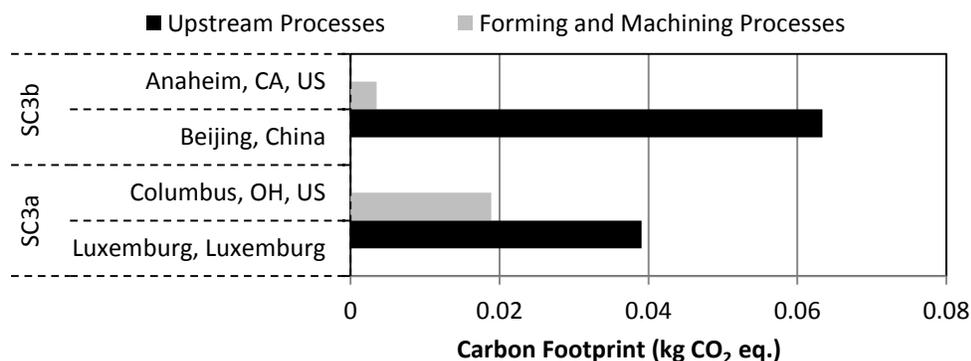
**Figure 4.9:** Resultant Carbon Footprint from Manufacturing Processes for Supply Chain Alternatives SC3a and SC3b
