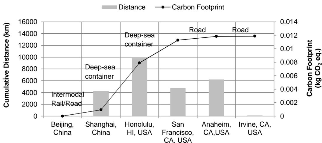
**Figure 4.8:** Transport Distance and Resultant Carbon Footprint for alternative SC3b
