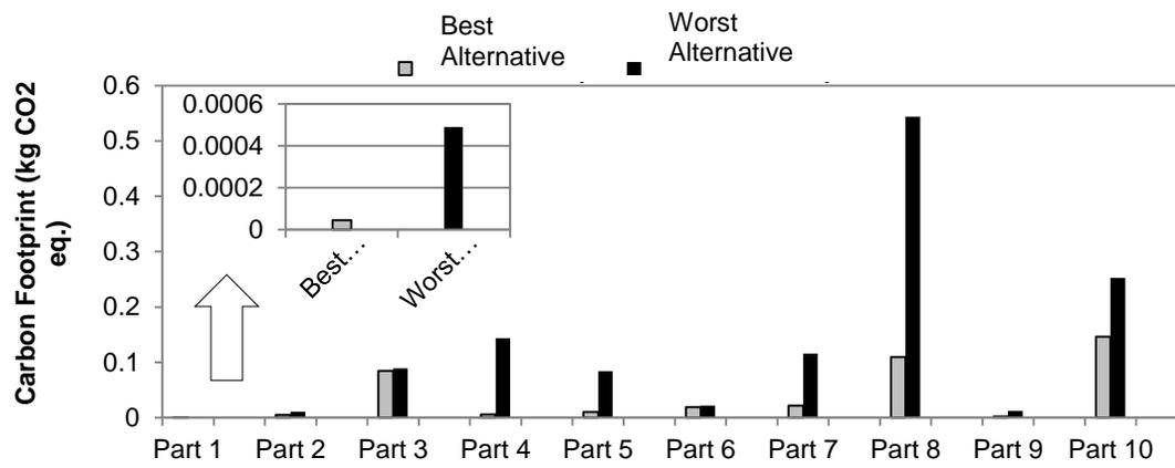
**Figure 4.15:** Best and Worst Alternatives of the Pedal Components
