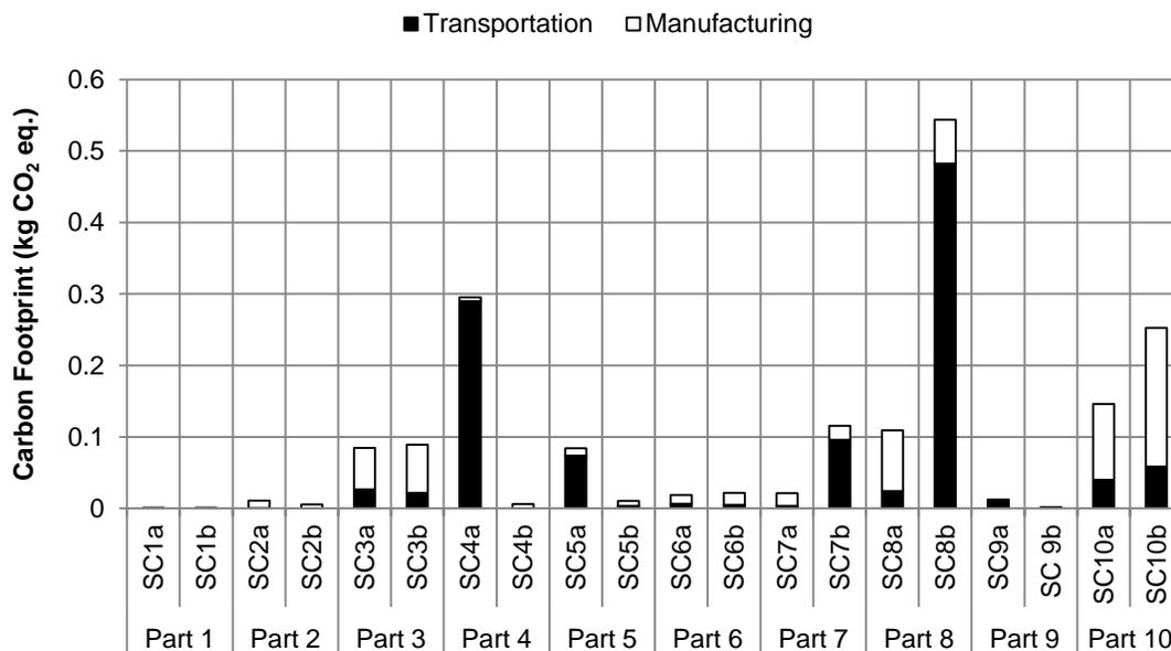
**Figure 4.14:** Carbon Footprint for Alternative Supply Chain Scenarios for Each Pedal Component
