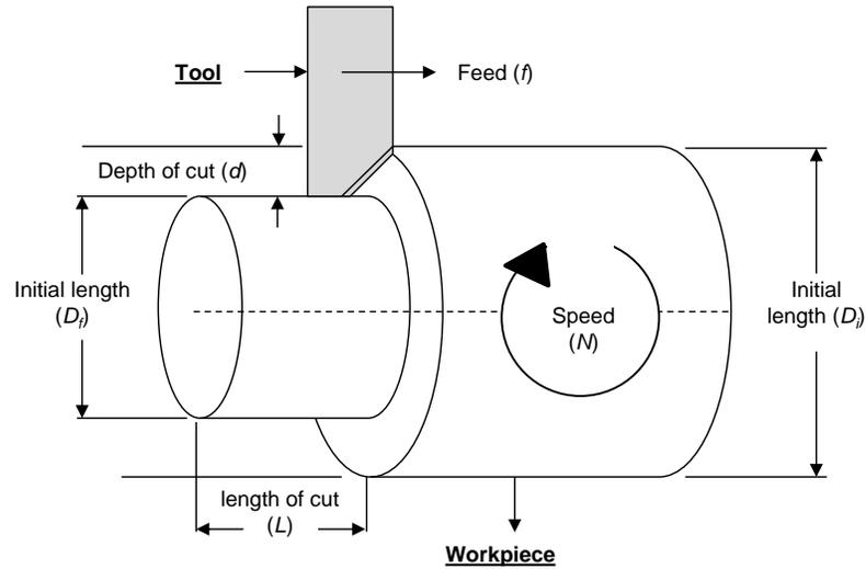
**Figure 3.8:** Schematics of Turning Operation Showing the Process Parameters
