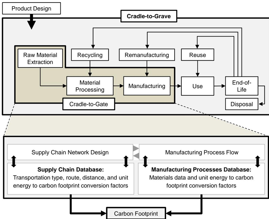
**Figure 3.1:** A Framework to Integrate Energy and Carbon Footprint Reduction into Manufacturing Process Flow and Supply Chain Network Design
