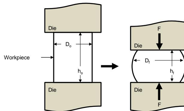
**Figure 3.6:** Basics of Open-die Forging (Kalpakjian, 2001)
