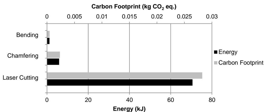
**Figure 4.10:** Process Energy Use and Carbon Footprint in Columbus, OH, USA for SC3a
