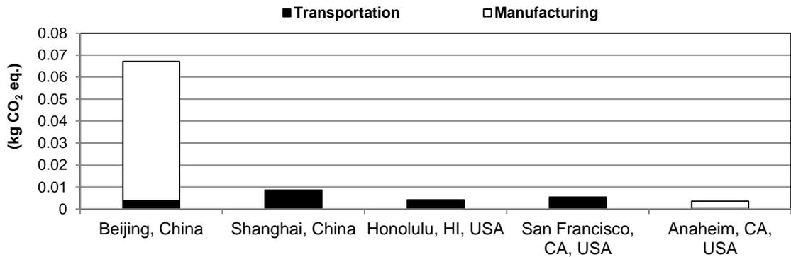
**Figure 4.6:** Carbon Footprint of Supply Chain Alternative 2 (SC3b)
