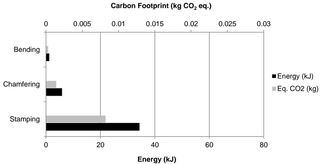
**Figure 4.11:** Process Energy Use and Carbon Footprint in Anaheim, CA, USA for SC3b
