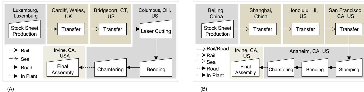
**Figure 4.4:** Supply Chain Alternatives (A) SC3a and (B) SC3b for Pedal Body Plate Production
