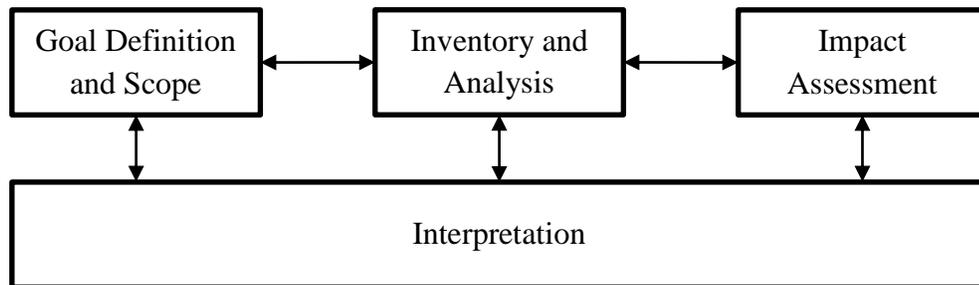
**Figure 2.2:** LCA Principles and Framework According to ISO 14040 (ISO, 2012)
