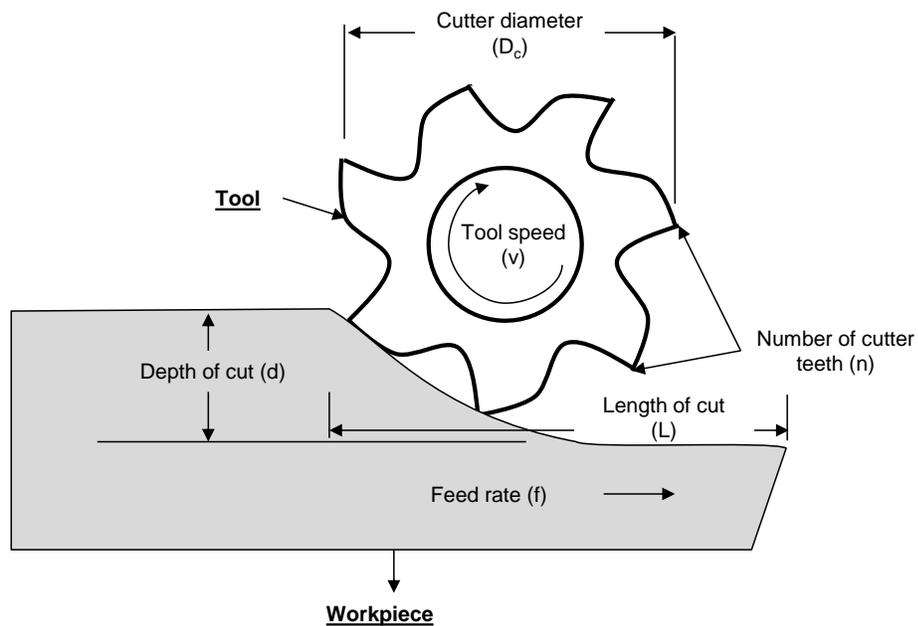
**Figure 3.9:** Milling Process Terminology Using a Slab Mill (DeGarmo et al., 1988)
