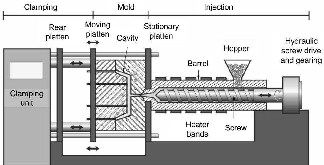
**Figure 3.5:** Illustration of Injection Molding Process (Plastic Injection Molding, 2002)
