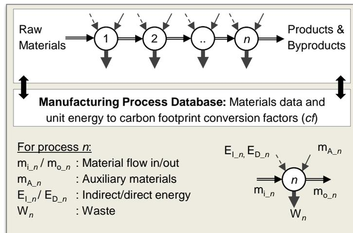
**Figure 3.3:** Input and Output Modeling for Unit Manufacturing Processes and Linking of Models for Manufacturing Process Flow
