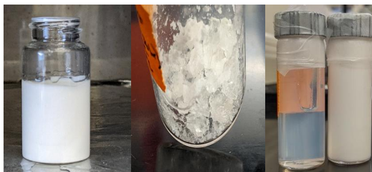
Figure 4.33: Polymer formed while curing in a solution of EtOH (right) and THF (middle) without sparging and after sparging (left) with the THF on the right of the image and ETOH on the left.
