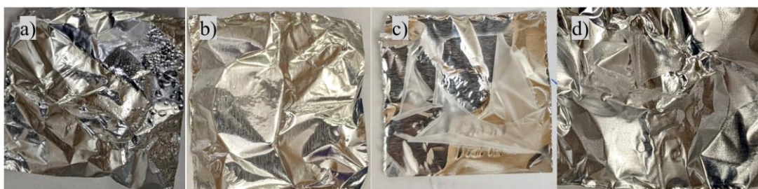
Figure 4.21: Deposition appearance of ES samples during the solvent trials. Images (a) show the typical depositions observed for EtOH samples. Image (b) shows the collector appearance on a more even coating that has been collected. Images (c + d) show the appearance of the completed cured film which often splits after a drying phase.
