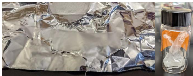
Figure 4.22: ES film from A-POSS: EB in THF solvent. Left is the deposited film onto the Al foil collector with right showing the film's appearance.
