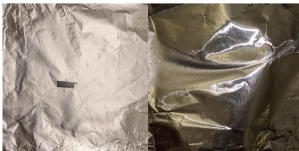
Figure 4.24: Film appearance after changing UV lamp position. (A-POSS/EB samples)
