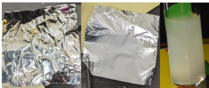
Figure 4.8: Deposition of A-POSS solution onto Al foil (left and middle) with the solution of A-POSS in ethanol post-cure (right).
