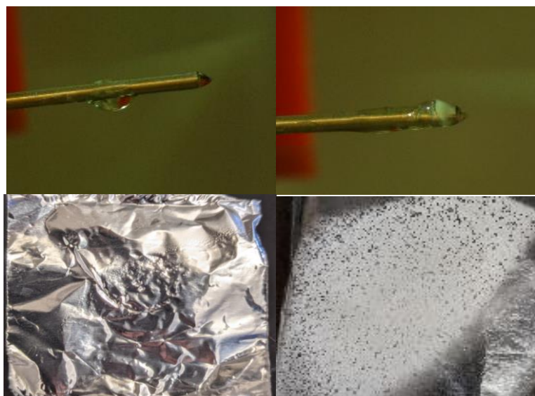
Figure 4.32: Effect of sparging the ES solution as depicted from the needle perspective. Top row – Image of the needle during electrospinning for a non-sparged (left) and sparged (right). Bottom row – two of the samples collected for the non-sparged (left) and sparged (right) ethanol solution
