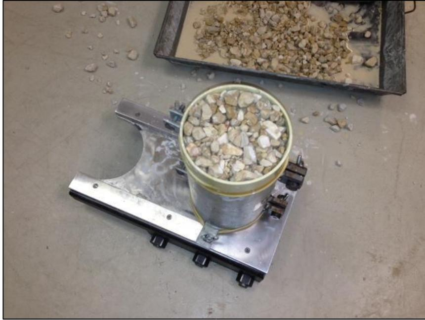
**Figure 4.3 Compacted specimen on custom compaction base**
