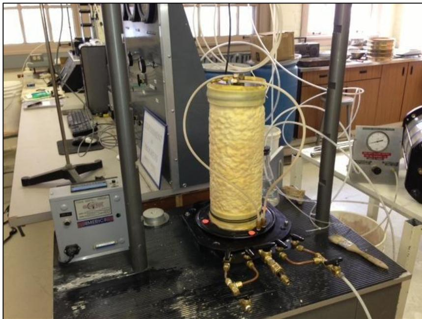
**Figure 4.5 Specimen with top platen, drainage lines and under vacuum**
