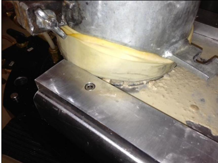
**Figure 4.4 Transfer of specimen from compaction base to triaxial base**
