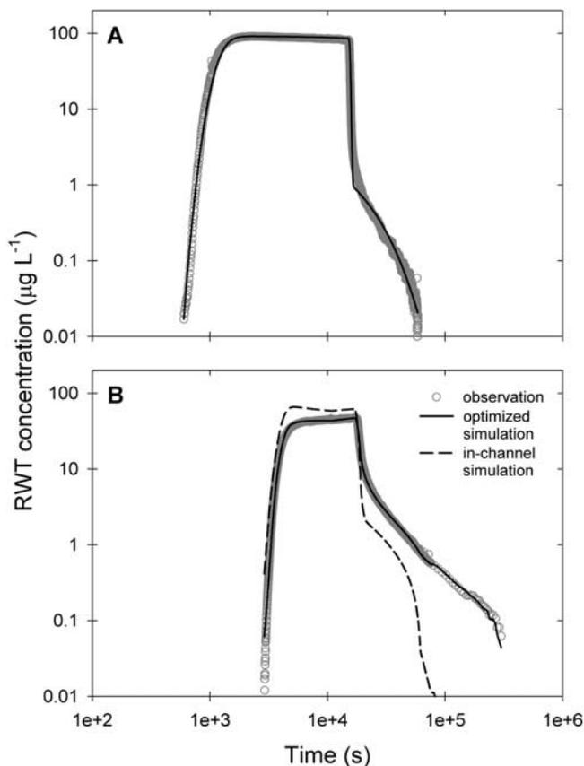
**Figure 3.** Observations and simulations of WS03 RWT tracer experiment, 6 April 2002 in (a) the 304 m bedrock reach (simulation 1) and (b) the downstream 367 m alluvial reach (simulations 2 and 3). All times are relative to the start of the drip (time 0 s).
