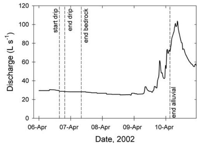
**Figure 2.** Watershed 3 hydrograph for 6–10 April 2002, recorded at the WS03 gauge house, 667 m downstream of the RWT drip location. The bedrock reach ends 304 m downstream from the drip location. Start and end of continuous drip of tracer is noted, as well as the end times of sampling at the end of the bedrock reach and end of the alluvial reach.
