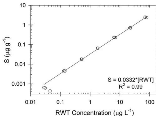
**Figure 4.** Rhodamine WT (RWT) sorption isotherm for WS03 streambed sediments (<2 mm size fraction), where  $S$  is the sorbed mass of RWT per mass of sediment. Three replicates were run for each RWT concentration value. Resulting  $K_d$  value is  $0.0332 \text{ L g}^{-1}$ .
