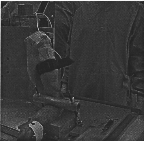
Figure 2.2: Custom shoulder-testing apparatus with specimen mounted and positioned to replicate previously established in vivo force-displacement protocol.
