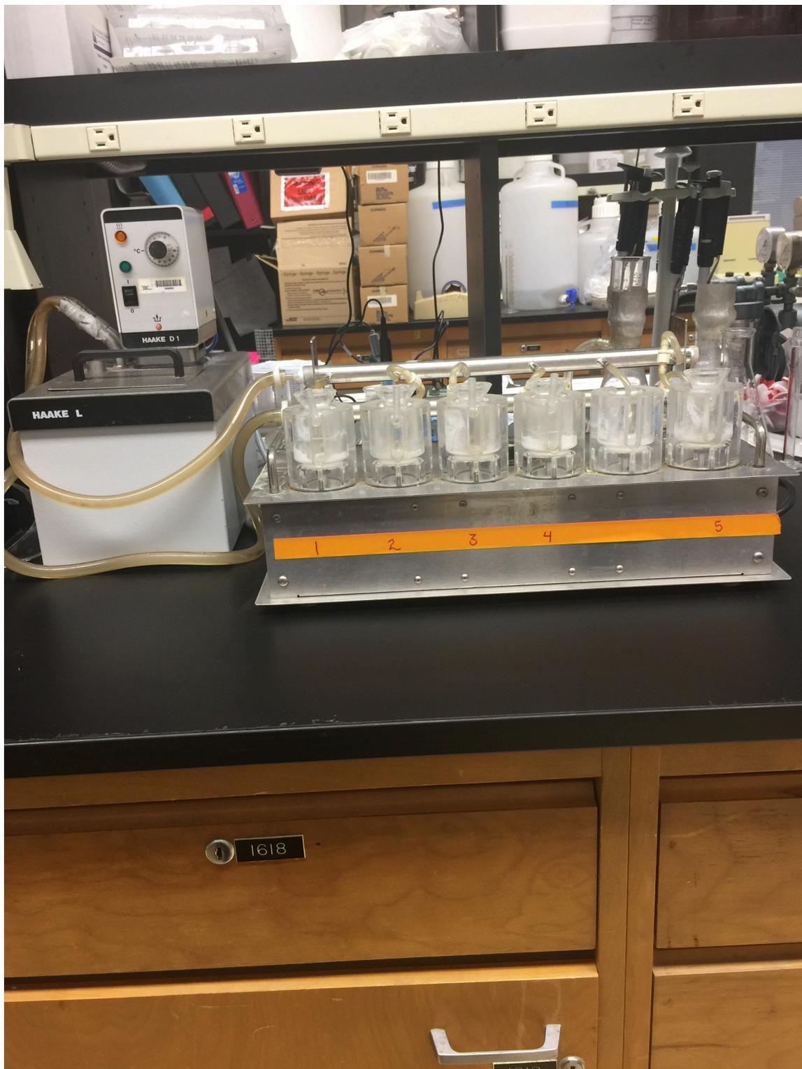
Figure (1.3) Waake Franz upright diffusion cells set system used in testing atenolol formulations.
