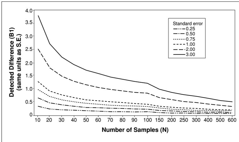
Figure 12. Required cycles for a time study.
