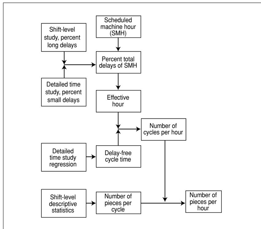
Figure D-1. Flow chart of information for production calculation.
