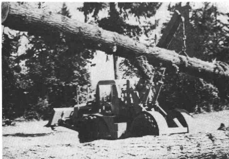
Figure 3. --Skidder-loader with boom extended and raised for loading logs.
