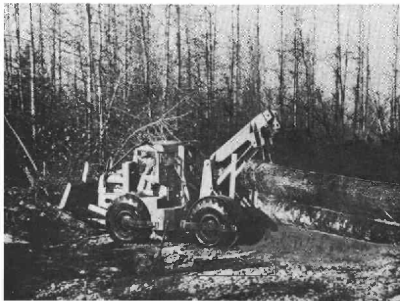
Figure 2. --Skidder-loader skidding tree-length logs.
