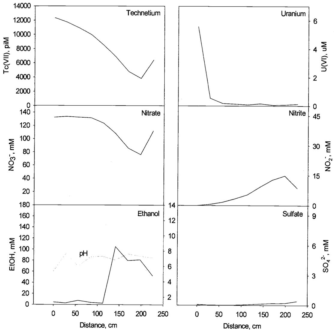
**Figure 30.** Area 1 model concentration profiles (Upper flow path). Data measured 29 Oct. 2003 during eleventh week of flowing conditions.
