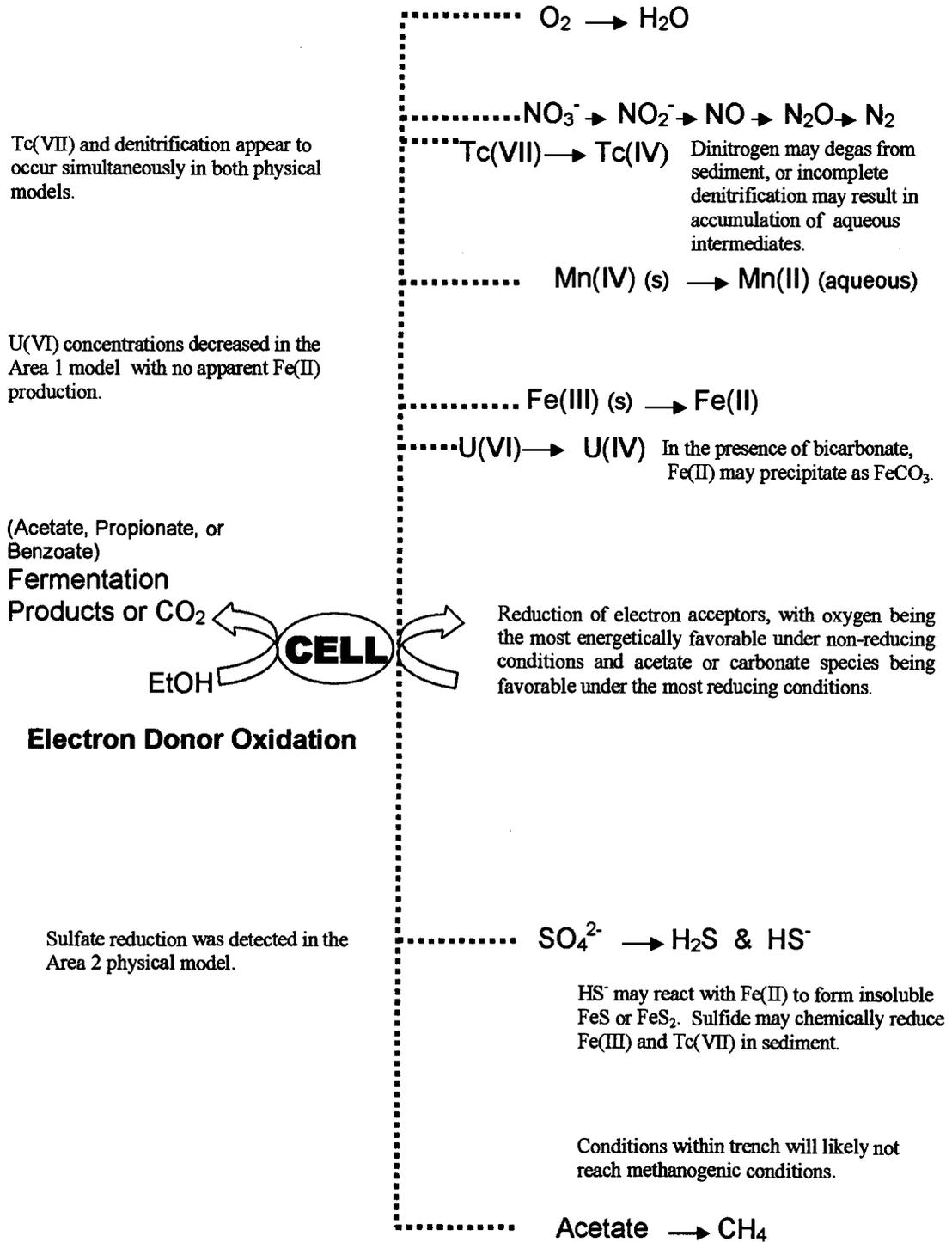
**Figure 33.** Conceptual diagram for principal redox reactions in the physical models.
