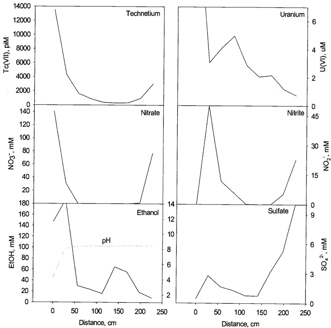
**Figure 27.** Area 1 model concentration profiles (Lower flow path). Data measured 16 Sept. 2003 during seventh week of flowing conditions.
