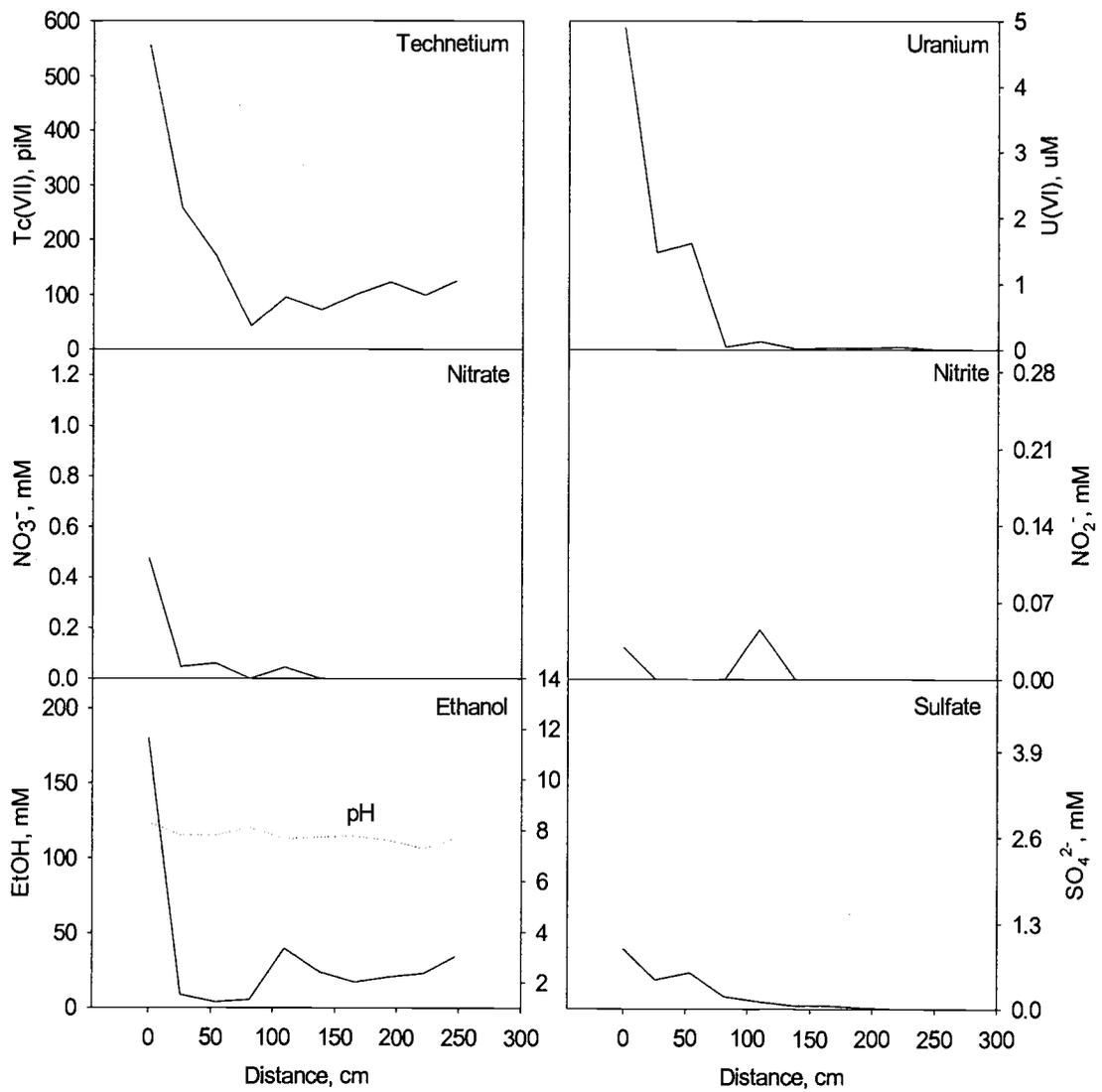
**Figure 22.** Area 2 column concentration profiles. Data measured 24 Oct. 2003 during fifth week of flowing conditions.
