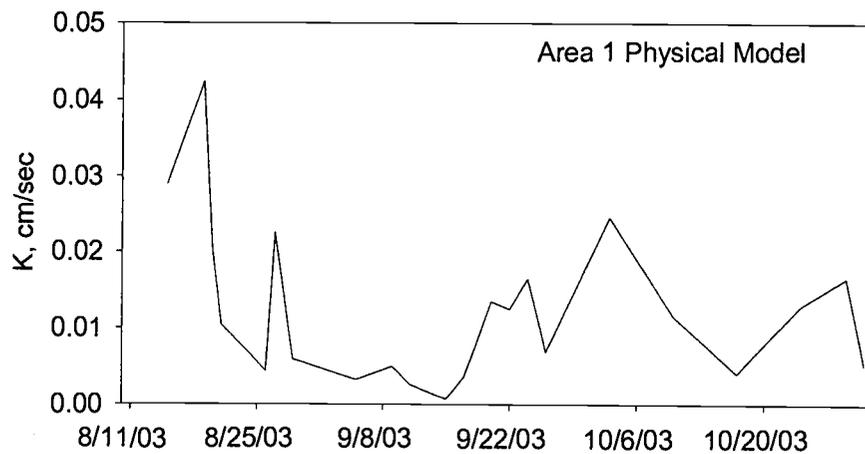
Figure 32. Hydraulic conductivity of the Area 1 column.
