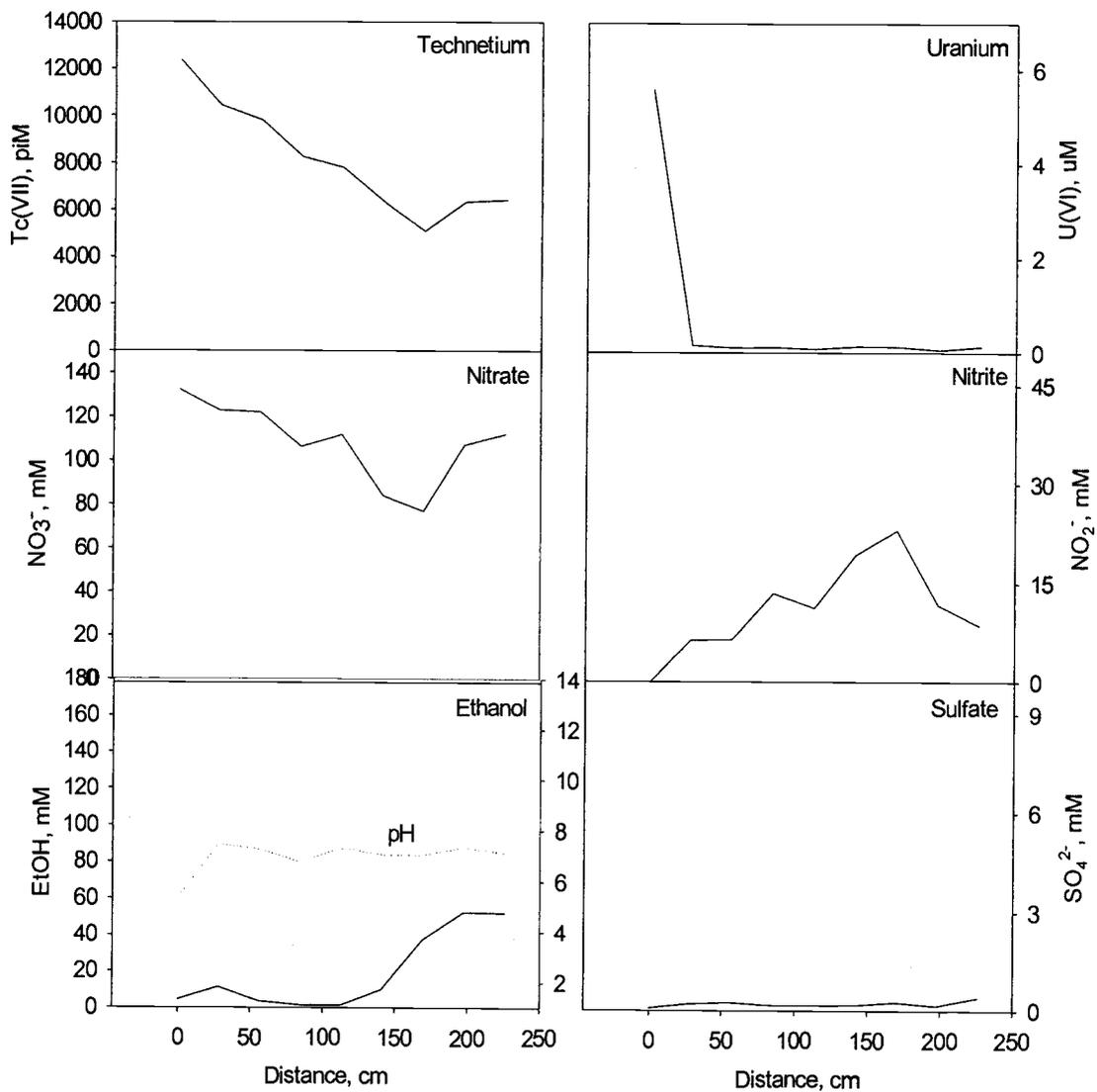
**Figure 31.** Area 1 model concentration profiles (Lower flow path). Data measured 29 Oct. 2003 during eleventh week of flowing conditions.
