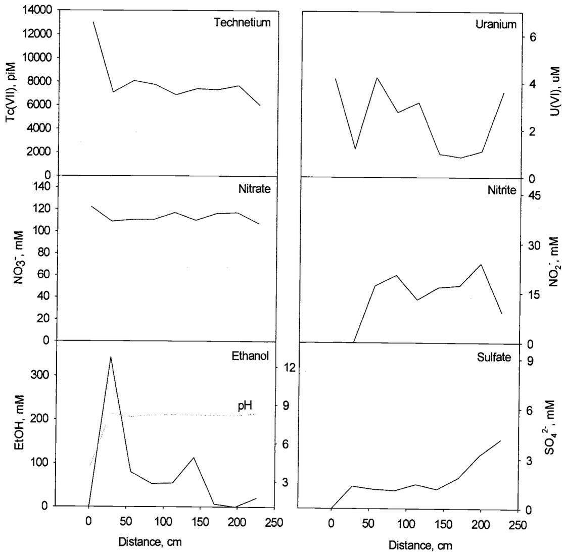
**Figure 24.** Area 1 model concentration profiles (Upper flow path). Data measured 19 Aug. 2002 during first week of flowing conditions.
