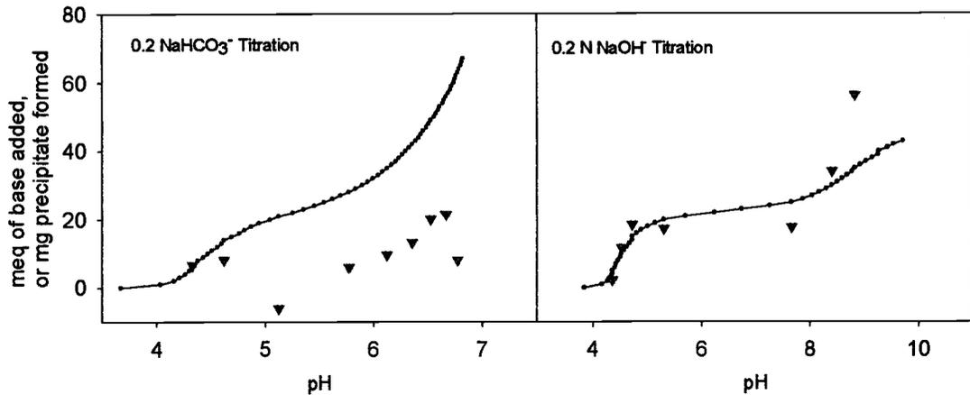
**Figure 13.** Mass of precipitate formed per 10 mL of titrant, either NaHCO<sub>3</sub> (left) or NaOH (right), added to FW21 groundwater, where ▼ represents mg of precipitate formed.
