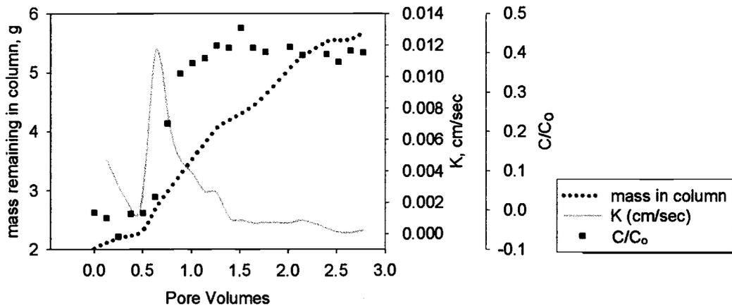
**Figure 14.** Relative precipitate concentration in column effluent ( $C/C_0$ ), precipitate mass remaining in the column, and corresponding hydraulic conductivity during precipitate transport experiment.
