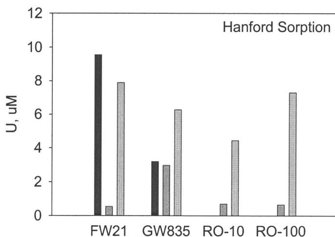
**Figure 16.** Aqueous uranium concentrations in batch experiments prior to contacting with sediment (—), after contacting with sediment (.....), and after bicarbonate addition (▨). RO-10 and RO-100 represent reverse osmosis treated water with 10 mM and 100 mM bicarbonate additions, respectively.
