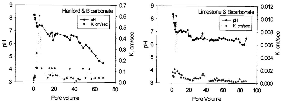
Figure 15. Change in hydraulic conductivity and pH observed during two pH adjustment experiments.
