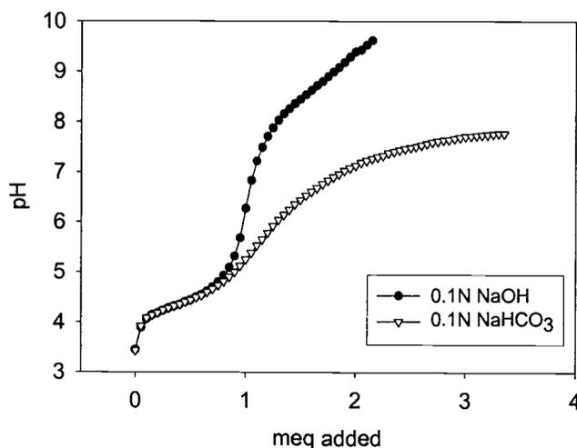
Figure 12. Titration of FW21 with 0.1N NaOH and 0.1N HCO<sub>3</sub>
