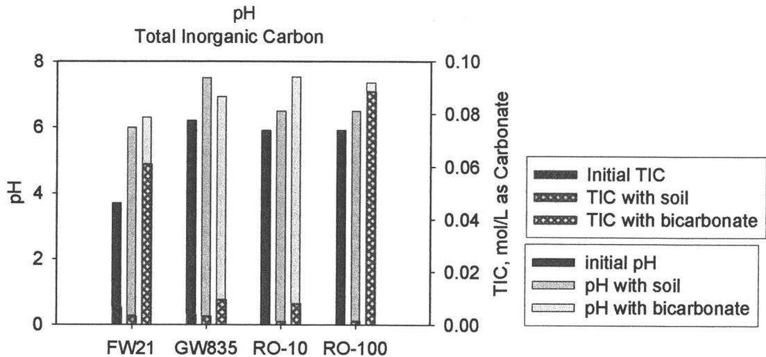
**Figure 17.** pH and TIC concentrations prior to contacting four solutions with sediment, after contacting with sediment, and after bicarbonate addition.
