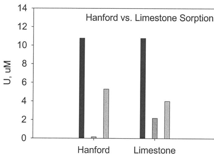
**Figure 18.** Uranium concentrations in the water prior to contacting with sediment (—), after contacting with sediment (—), and after bicarbonate addition (—).
