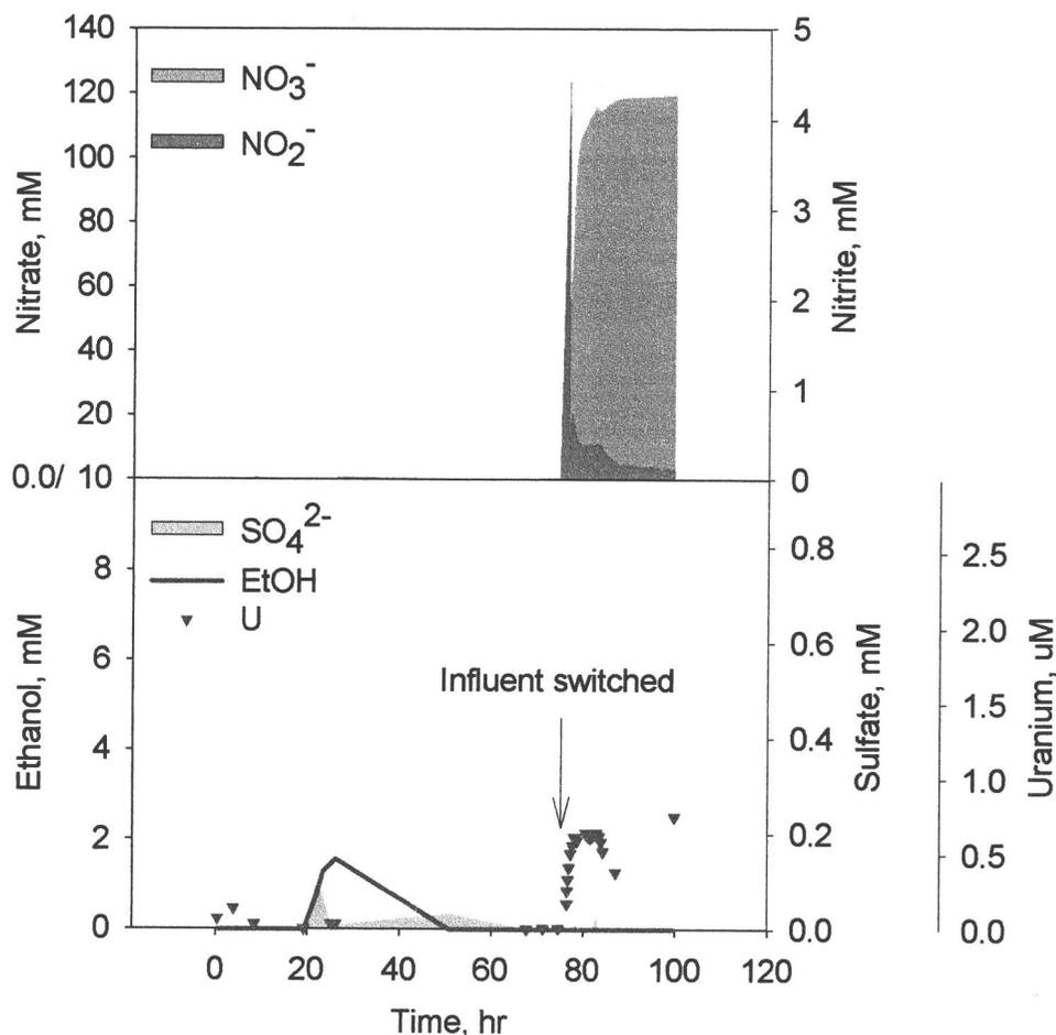
**Figure 19.** Concentrations in the column effluent measured over time. The arrow indicates the time when the influent was switched from the feed solution to 120 mM nitrate tap water.
