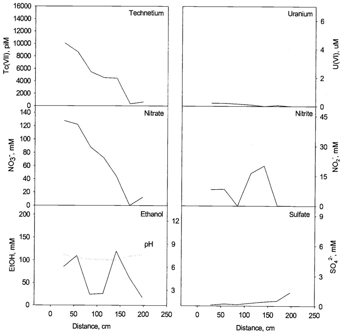
**Figure 28.** Area 1 column concentration profiles (Upper flow path). Data measured 23 Oct. 2003 during tenth week of flowing conditions.
