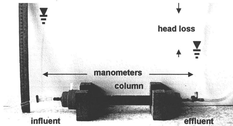
Figure 6. Column used for pH adjustment experiments.
