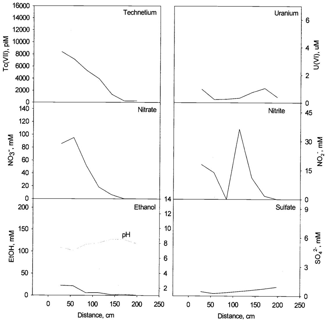
**Figure 29.** Area 1 column concentration profiles (Lower flow path). Data measured 23 Oct. 2003 during tenth week of flowing conditions.
