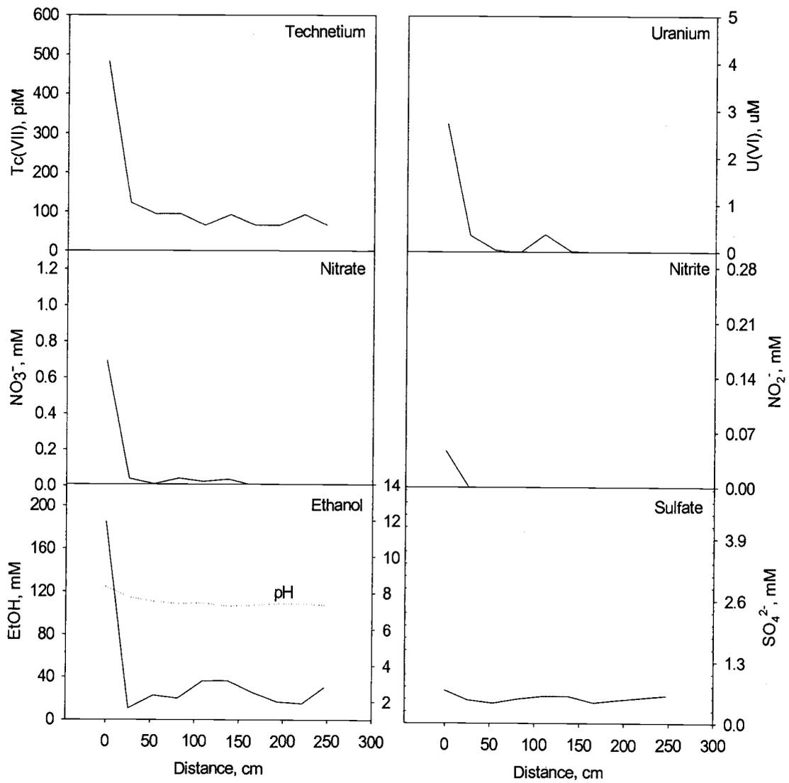
**Figure 21.** Area 2 column concentration profiles. Data measured 8 Oct. 2003 during third week of flowing conditions.
