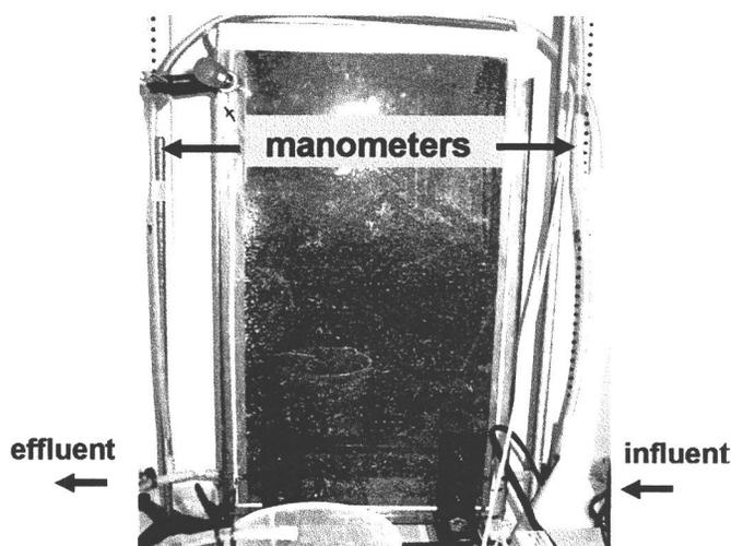
**Figure 7.** Laboratory chamber used for bio-immobilization experiments with FW21 groundwater.
