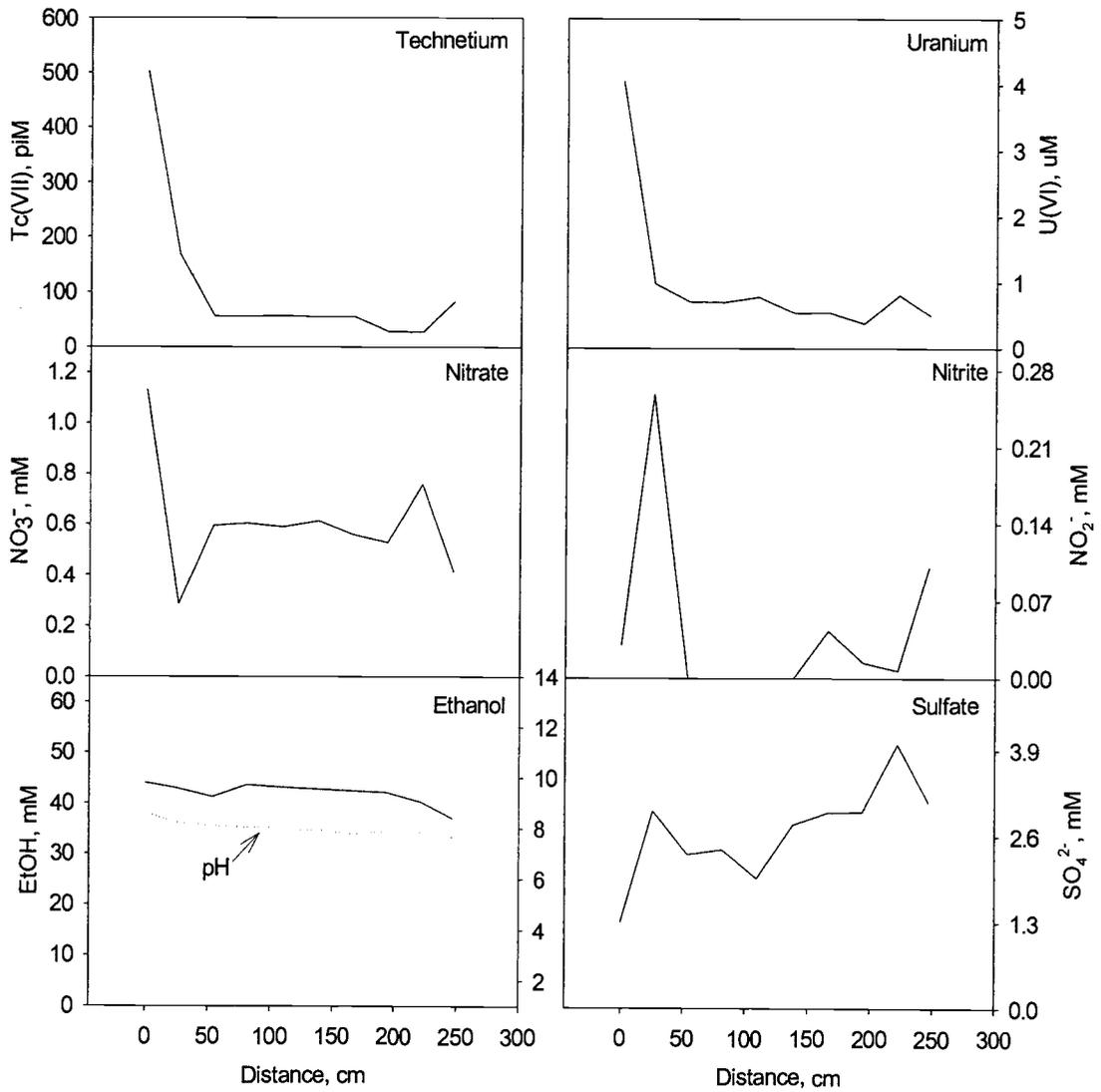
**Figure 20.** Area 2 column concentration profiles. Data measured 20 Sept. 2003 during first week of flowing conditions.
