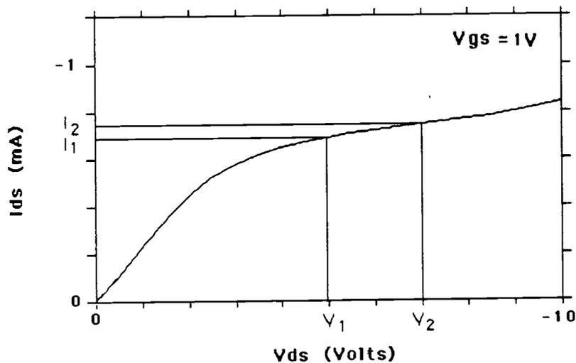
Fig. 2-2-3 I-V curve of a p-channel GaAs MESFET.  $I_1$  and  $I_2$  are drain currents at drain biases  $V_1$  and  $V_2$ , respectively.
