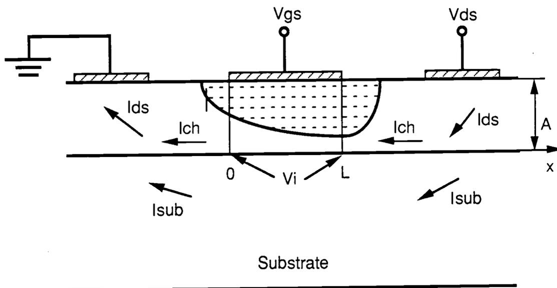
Fig. 2-1-1 Cross section of GaAs MESFET
