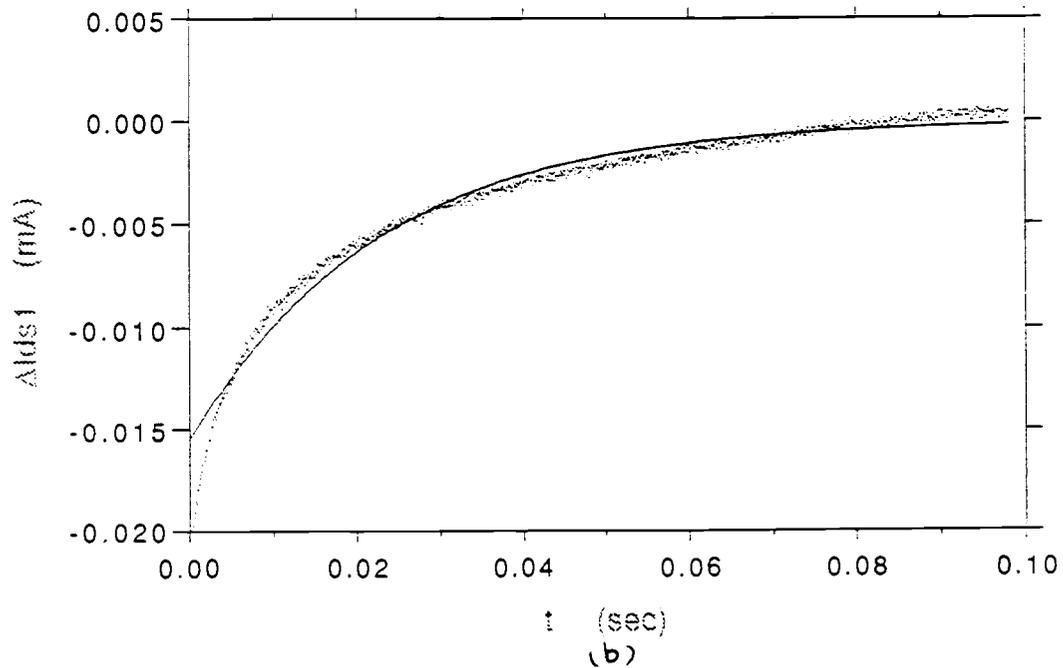
Fig. 5-2-1 The fitting of drain current transients by one-level model. The dots are measured data and the solid lines are the fitted curves. (a) response to drain voltage change from -7V to -6V; (b) response to drain voltage change from -6V to -7V
