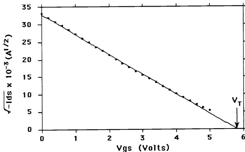
Fig. 3-2-3 Threshold voltage  $V_T$  extracted from  $\sqrt{\text{abs}(I_{ds})} - V_{gs}$  curve according to "square law" model
