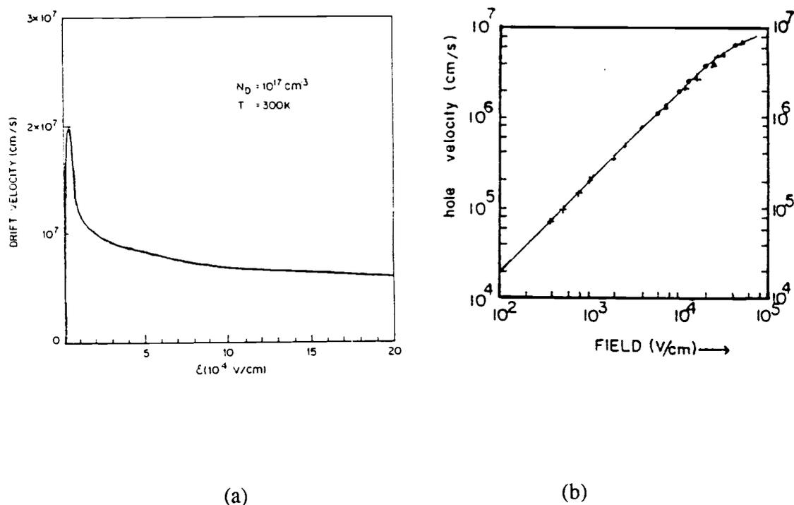
Fig. 2-1-3 (a) Electron velocity vs. electric field in GaAs (after P. Smith, M. Inoue, and J. Frey in Ref: 21 ) and (b) Hole velocity vs. electric field in GaAs ( after V. L. Dalal in Ref: 22 )
