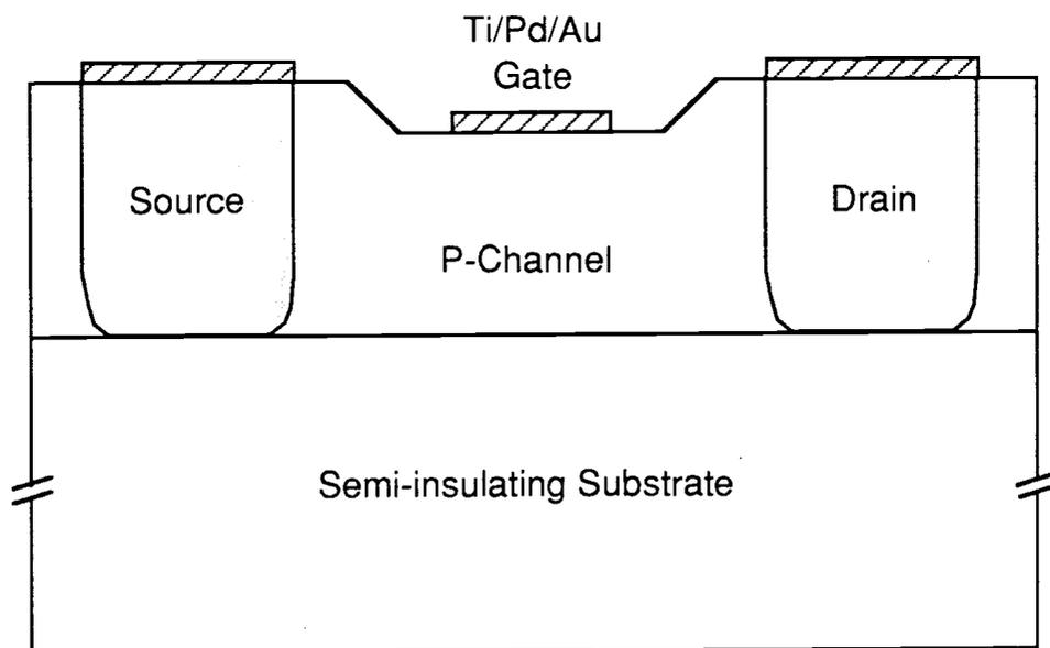
Fig. 3-1-1b Cross section view of the p-channel MESFET
