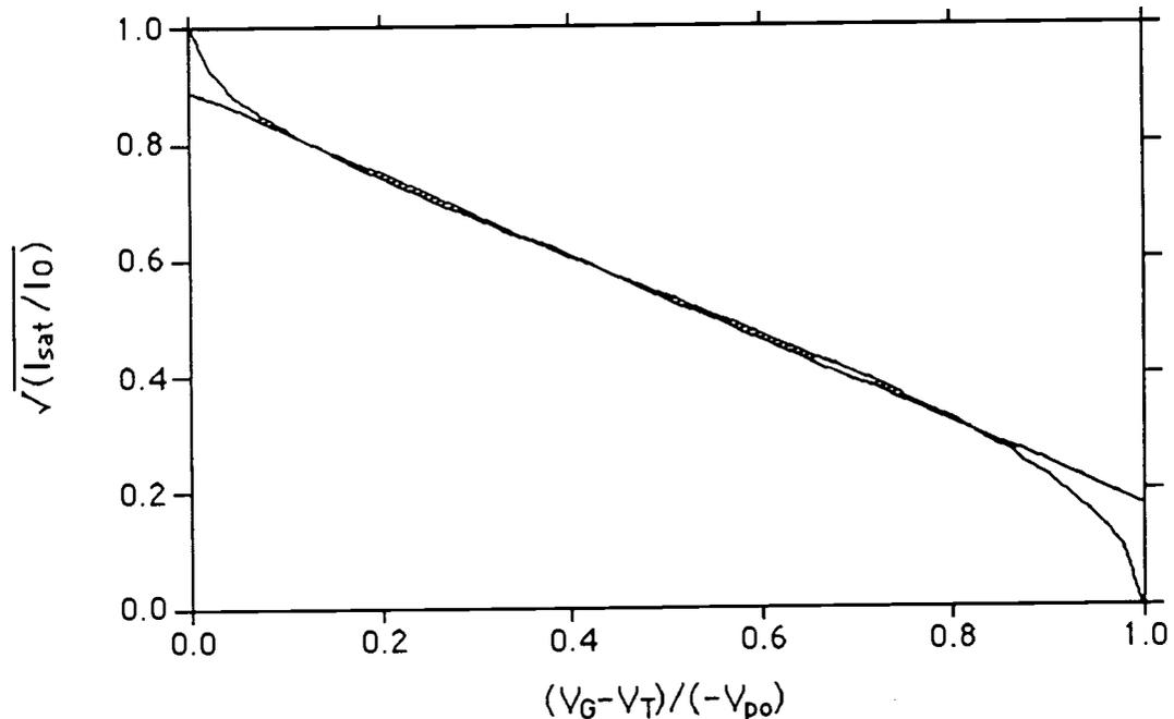
Fig. 2-1-5 Values of  $\sqrt{I_{\text{sat}}/I_0}$  as a function of gate bias voltage for MESFETs obeying Eq.(2-1-20a). The straight line has expression as Eq.(2-1-23)
