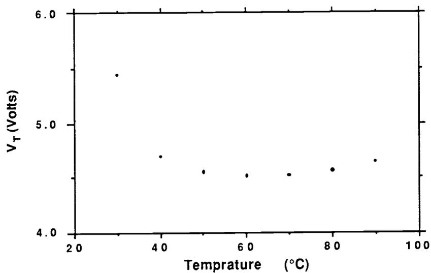
Fig. 4-1-3 Temperature dependency of threshold voltage at bias  $V_{ds} = -7V$
