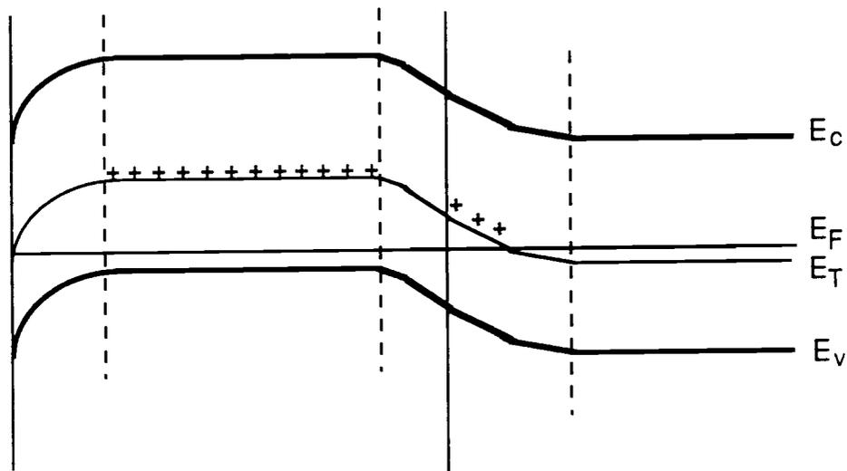
Fig. 2-2-5 Band diagram of a p-channel GaAs MESFET.  $E_C$  and  $E_V$  are the conduction band and valence band respectively.  $E_F$  is the Fermi level and  $E_T$  is the deep trap level, i.e. EL2.
