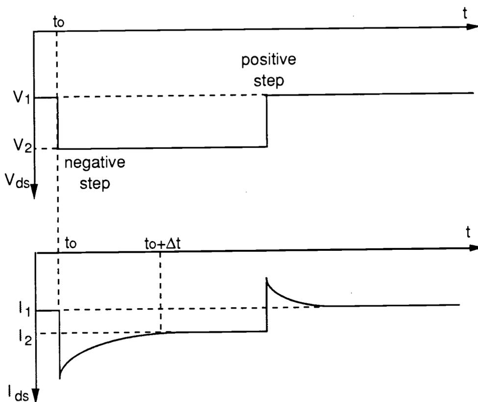
Fig. 2-2-4 Drain current response to step drain bias change
