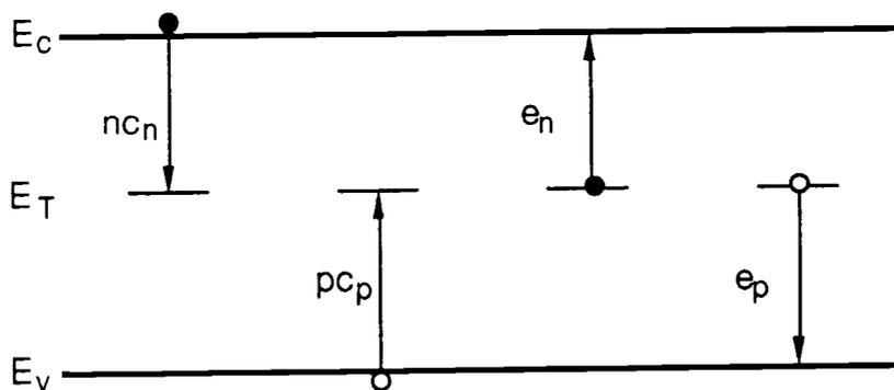
Fig. 2-2-1 Emission and capture processes at a deep level of energy  $E_T$ . The quantities near the arrows are the rates (in  $\text{s}^{-1}$ ) of the processes.
