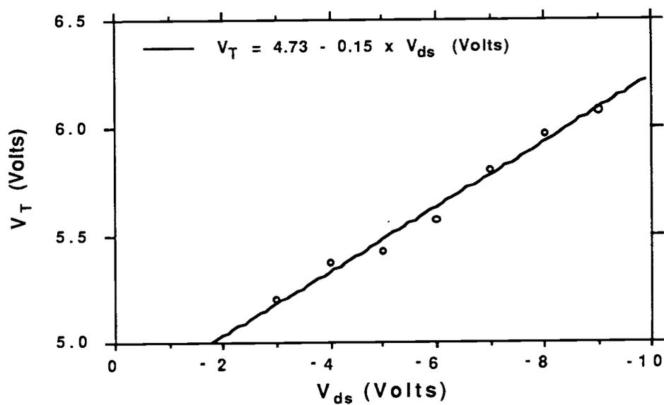
Fig. 4-1-4 Threshold voltage at different drain biases and at room temperature
