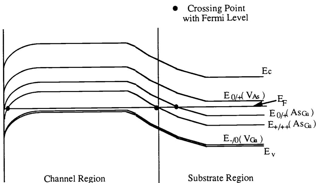
Fig.5-2-4 Band diagram for p-channel GaAs MESFET with defect levels
