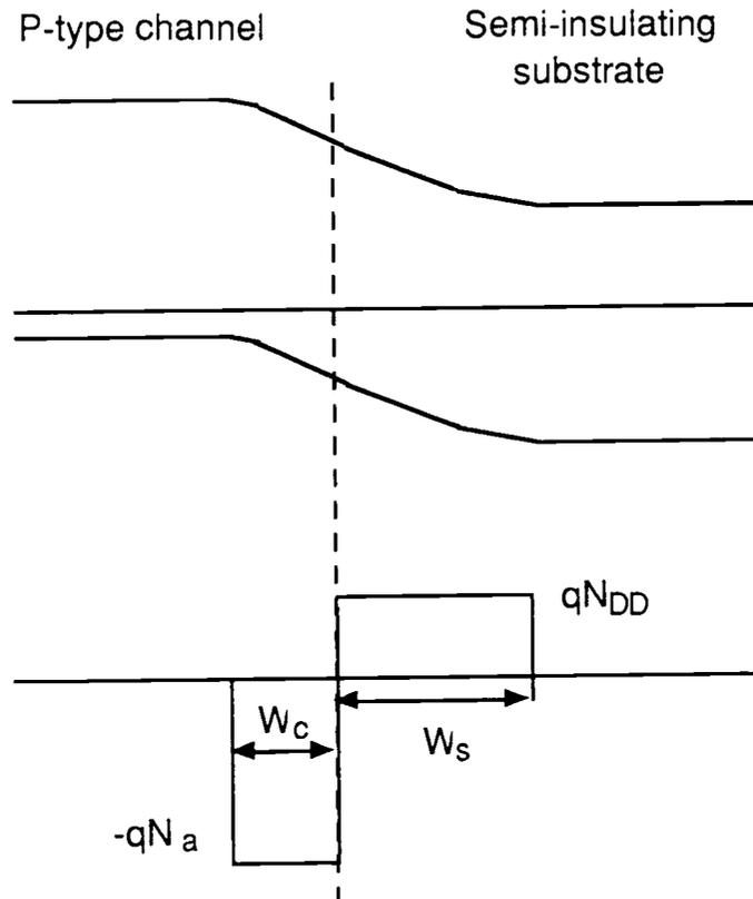
Fig. 2-2-2 The band diagram and charge distribution for channel-substrate interface
