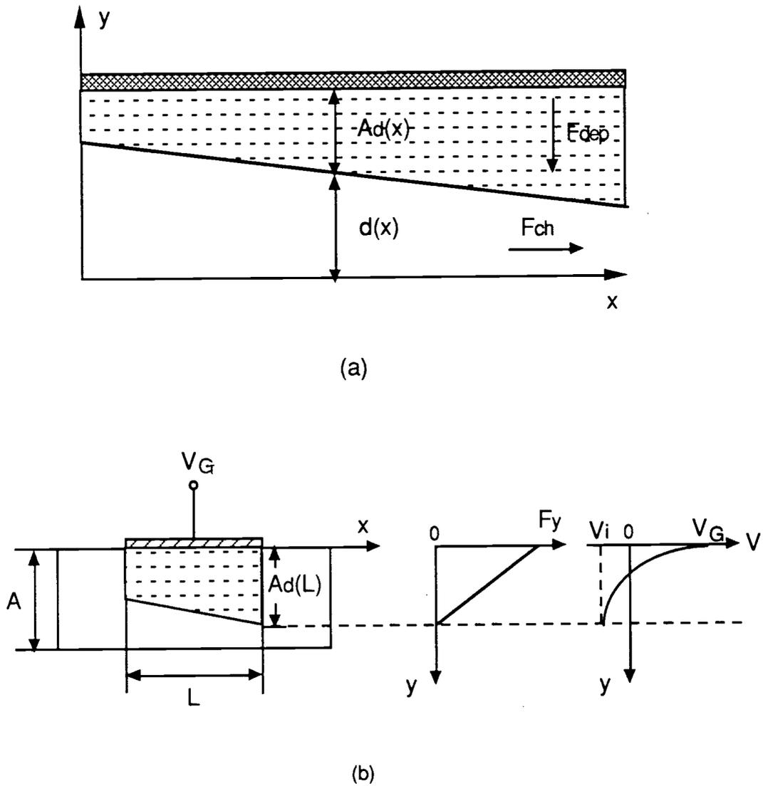
Fig. 2-1-2 Depletion region and conducting channel under gate. (a) Section of a gradually varying channel under gate; (b) charge, electric field and potential distributions in the depletion region.
