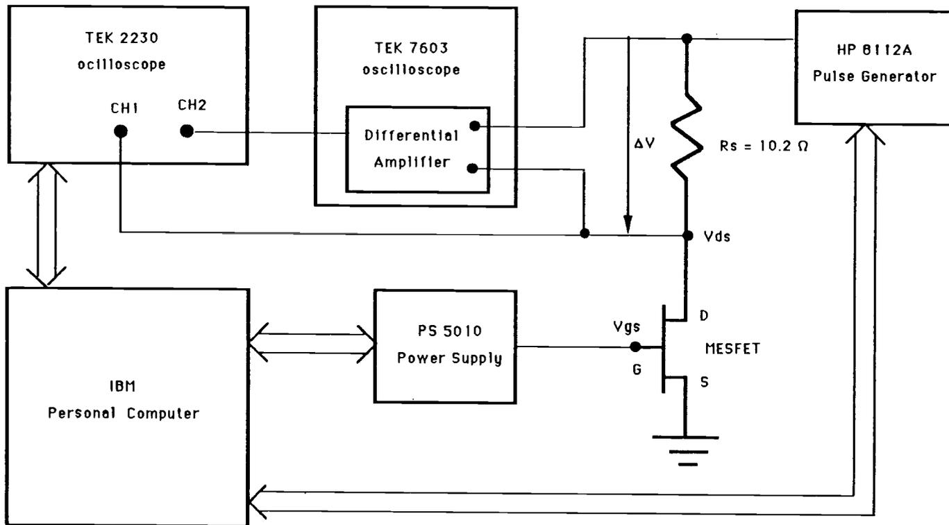
Fig. 3-3-1 Experimental Setup for Drain Current transient Measurement
