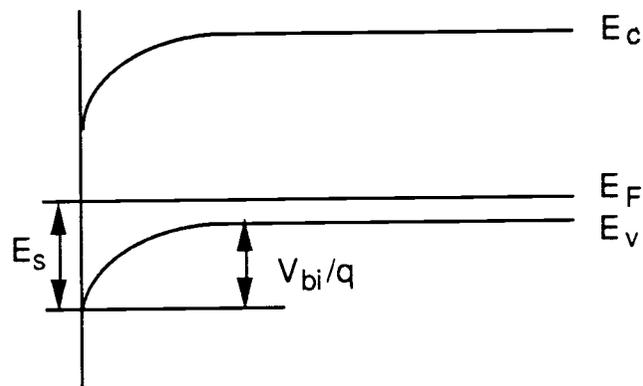
Fig. 5-1-1 The definition of built-in voltage  $V_{bi}$ .  $E_s$  is the Fermi level pinning energy on surface.
