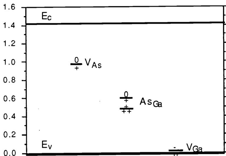
Fig. 5-2-3 Literature values for the level positions of vacancies and antisite defect of EL2 complex in GaAs at  $T = 300$  K.
