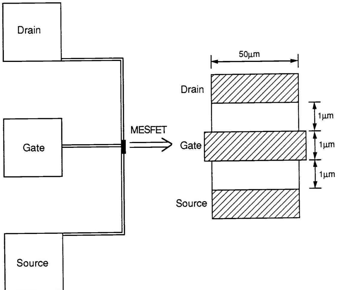
Fig. 3-1-1a Over looking view of the p-channel MESFET
