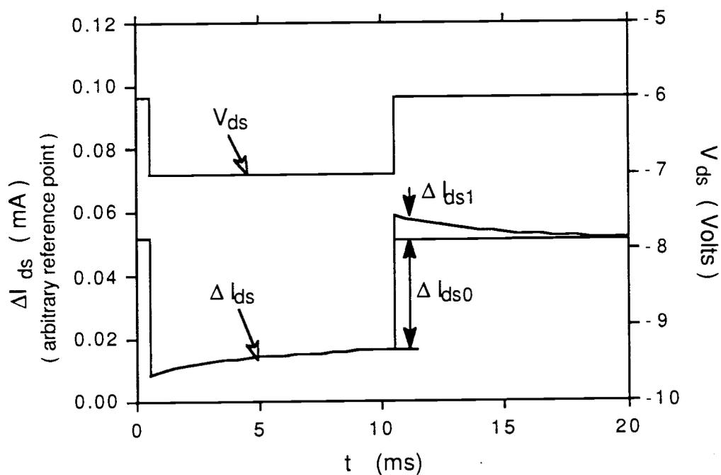
Fig. 4-2-1 Drain current response at room temperature and gate biased at 1V
