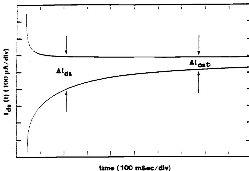
Fig. 6-2-2 Superposition of positive and negative step transients to determine  $\Delta I_{ds}$ . (n-channel GaAs MESFET data, Ref: 12)
