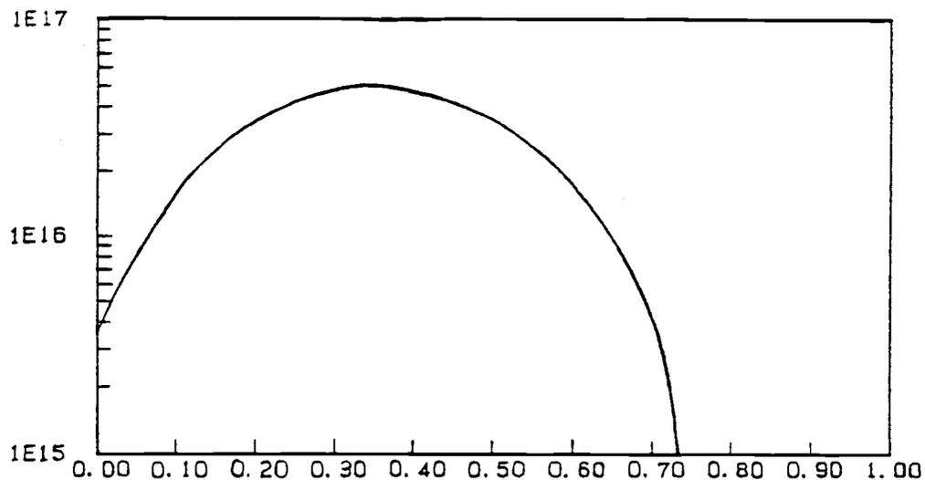
Fig. 3-1-2 Channel doping profile. Be implantation at energy 140 keV with a dose of  $2.3 \times 10^{12} \text{ cm}^{-2}$
