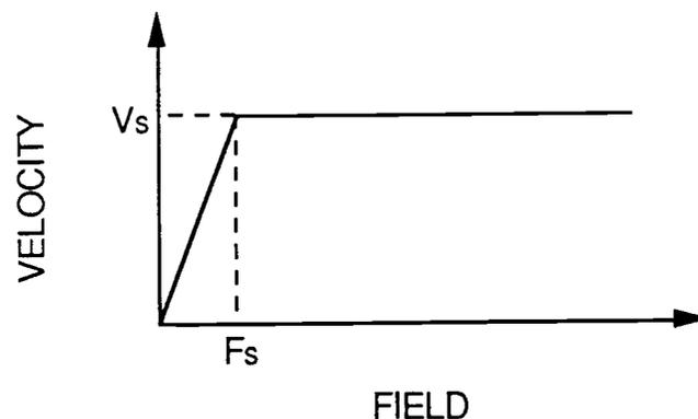
Fig. 2-1-4 Simplified velocity-electric field dependence
