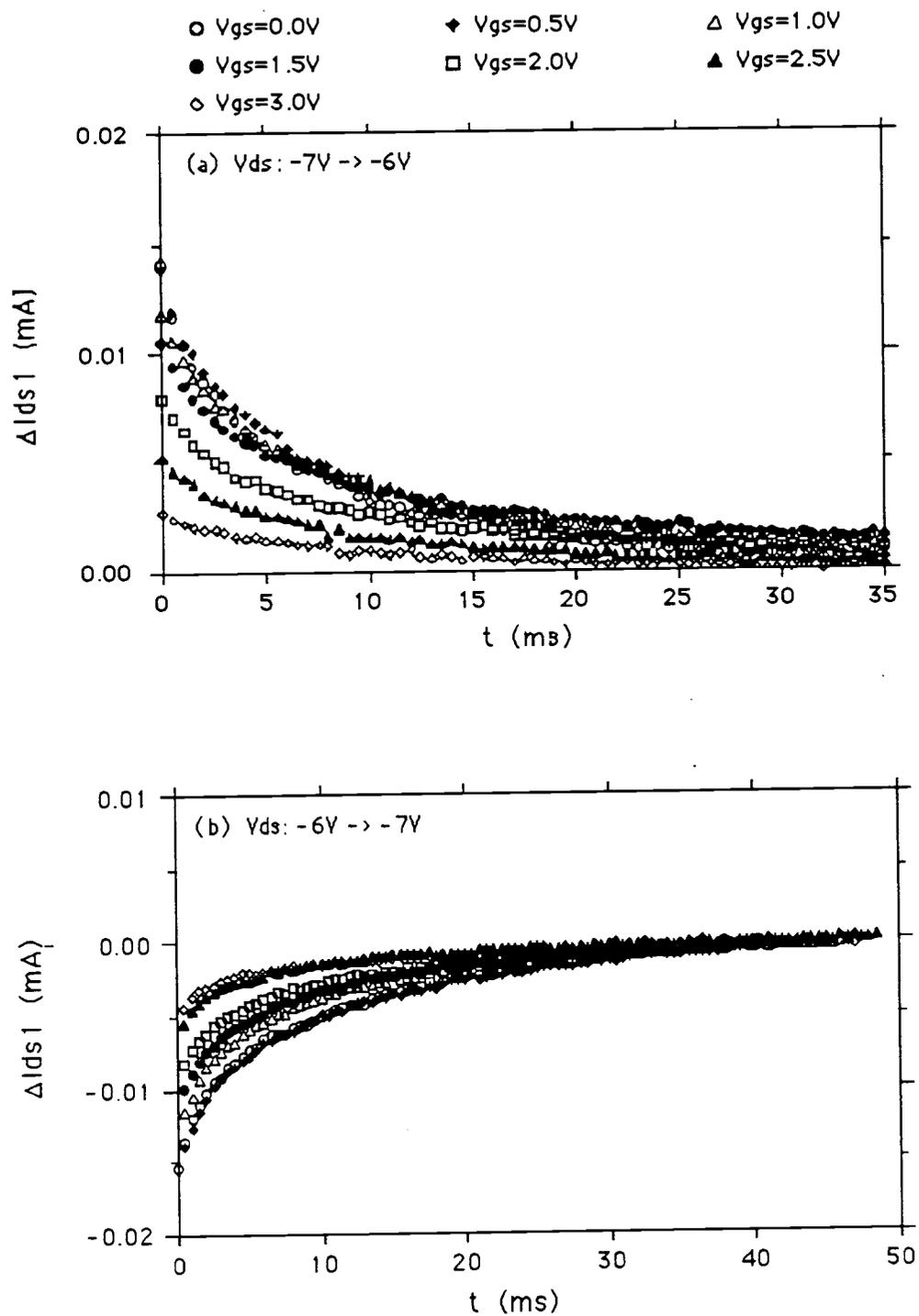
Fig. 4-2-3  $\Delta I_{DS1}$  for different gate biases at room temperature. (a) response to positive step  $V_{DS}$ ; (b) response to negative step  $V_{DS}$
