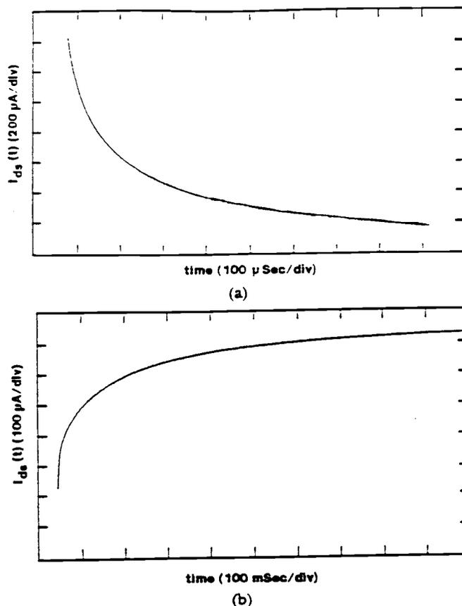
Fig. 6-2-1 Drain current transient of a  $1\mu\text{m}$  gate-length GaAs MESFET with a  $300\mu\text{m}$  gate width. (a) a drain voltage step from 1 to 2 V and (b) a step from 2 to 1V. (Results after P.C. Canfield, S. C.F. Lam, and D. J. Allstot, Ref: 12)
