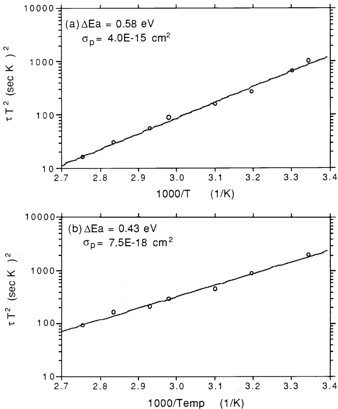
Fig. 5-2-2 ( $\tau T^2$ ) vs. ( $1000/T$ ) curves. Open circles are the experimental data. The straight lines are fitted curves of Eq.(5-2-2). (a) Data from positive transient; (b) Data from negative transient
