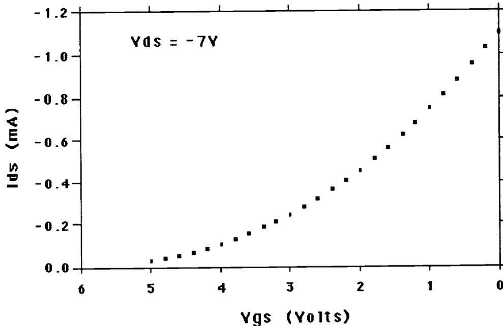
Fig. 4-1-2 Measured  $I - V_{gs}$  curve for p-channel GaAs MESFET at  $V_{ds} = -7V$
