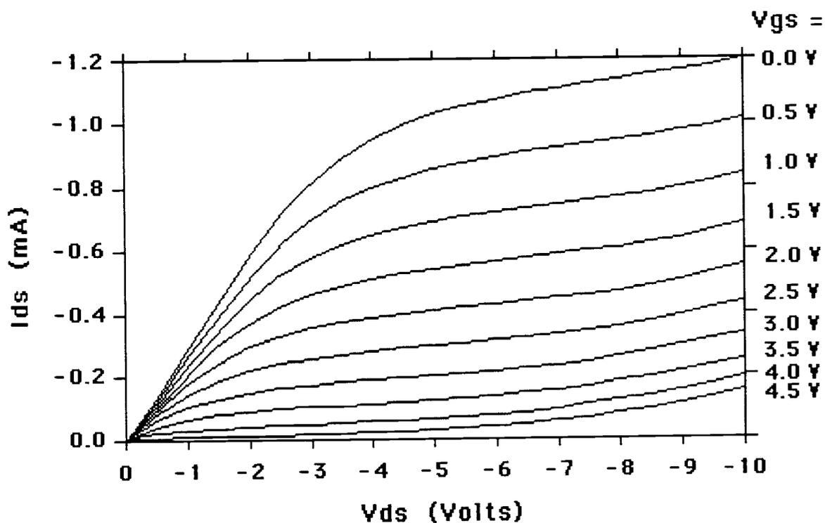
Fig. 4-1-1 Measured I - V curve for p-channel GaAs MESFET
