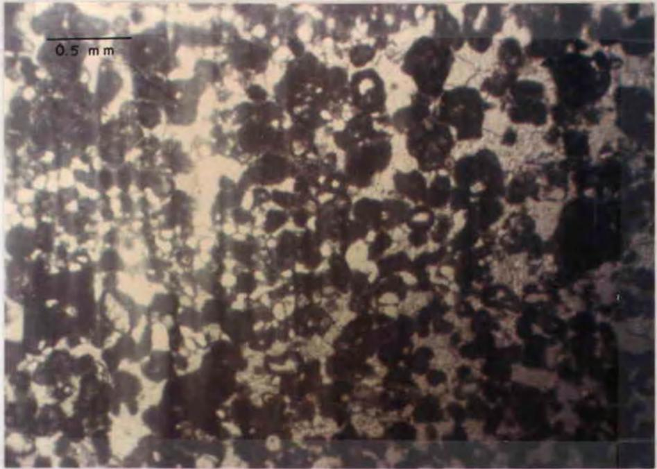
Figure 32. Photomicrograph of silty packed pelsparite (Bed #11, Figure 31), Gypsum Spring Tongue of the Twin Creek Formation. Plane light.
