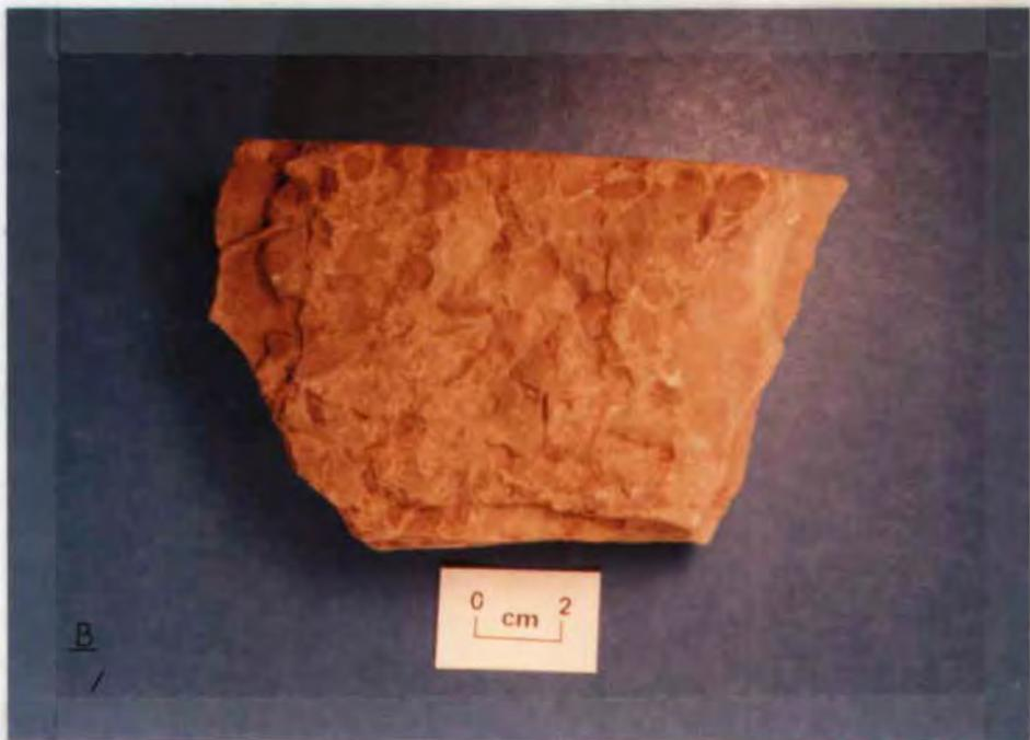
Figure 33. a) Very fine-grained sandstone of the Gypsum Spring Tongue, Twin Creek Formation showing edgewise siltstone intraclasts, symmetrical and migrating asymmetrical ripple laminations. b) underside of sample showing layer of concentrated siltstone intraclasts. Bed #7 (Figure 31). Gypsum Spring Tongue, Twin Creek Formation.
