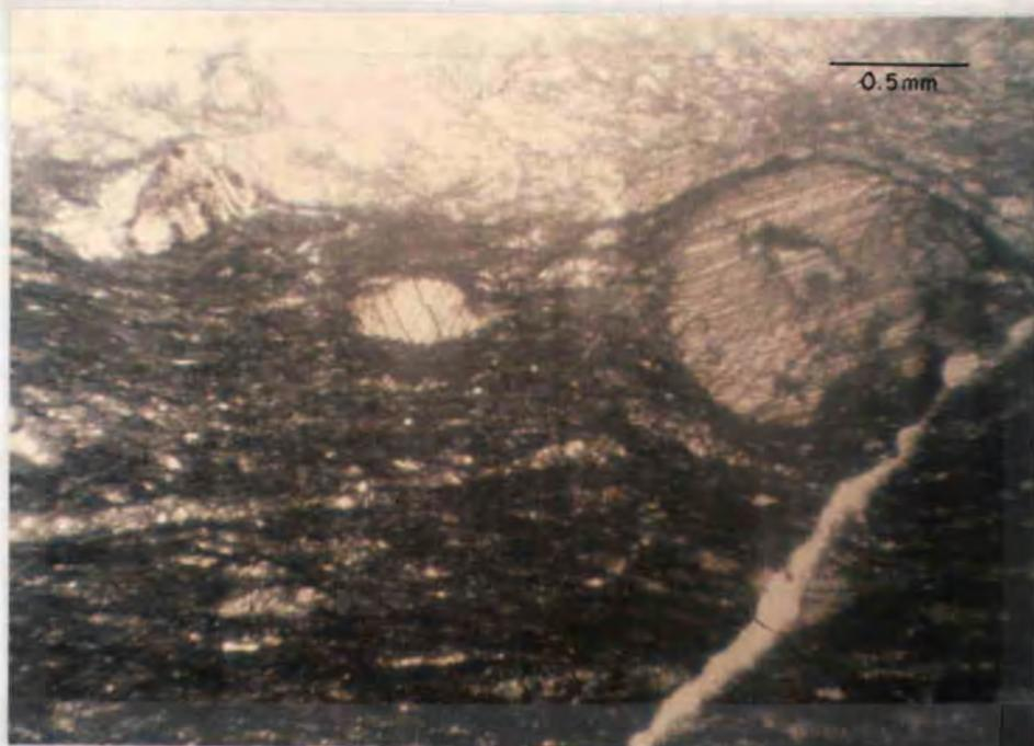
Figure 5. Photomicrograph, sheared limestone of the Scott Peak Formation from the Medicine Lodge thrust. Note flow lines of micrite (M) around calcite crystals (C). Circular crinoid columnal right center; calcite vein at filling top. Sample Kmb 79-269, SW $\frac{1}{4}$ , Section 30, T. 15 S., R. 9 W. Plane light.
