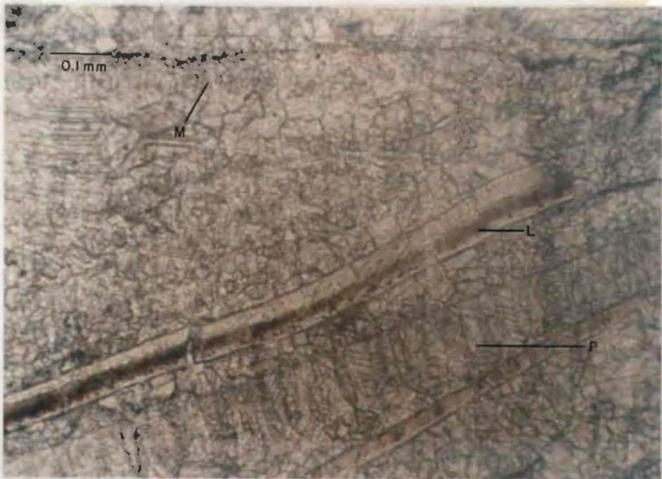
Figure 12. Photomicrograph, sparse biotranssparite. L, *Lingula* shell fragments; P, recrystallized pelecypod shell fragment showing internal structure; M, recrystallized pelecypod shell with a micrite rim. Sample Kmb 79-51, Dinwoody Formation, NE $\frac{1}{4}$ , NE $\frac{1}{4}$ , Section 30, T. 15 S., R. 9 W. Plane light.
