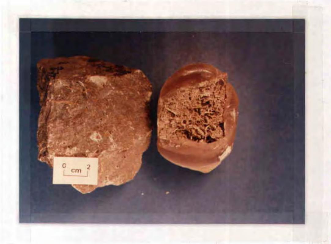
Figure 47. Cast of a matted and tangled mass of grass (?) roots. Sample of rock on left prior to impregnation with plastic and dissolution of the calcite matrix, Round Timber limestone.
