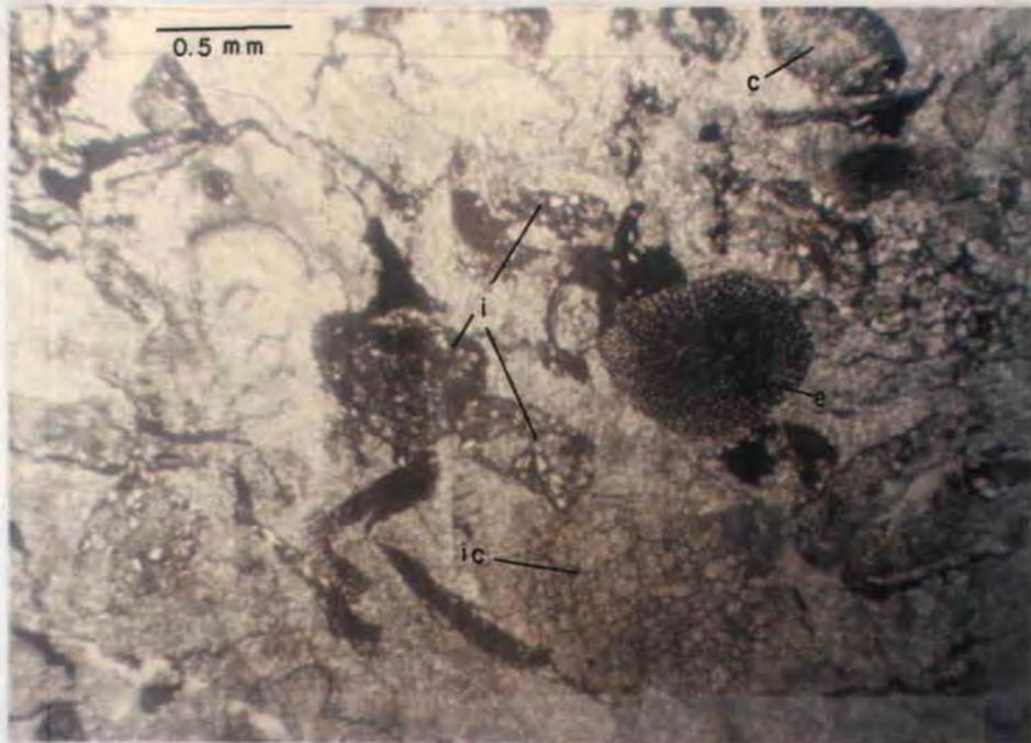
Figure 25. Photomicrograph of limestone in the Woodside Formation near the Woodside-Thaynes contact showing red hematite cement concentrated in intraparticle pores of echinoid plates (e), siltstone intraclasts (i), in calcite lithoclasts (c), and as local zones of interparticle cement in calcite spar (ic). Sample Kmb 79-106, NE $\frac{1}{4}$ , Section 8, T. 15 S., R. 9 W. Plane light.
