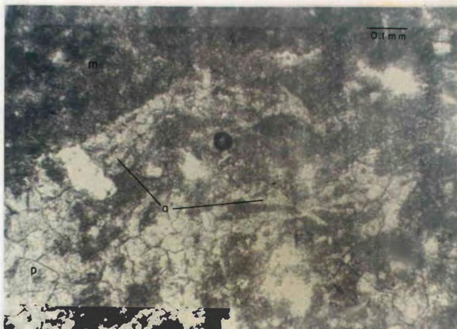
Figure 16. Aggrading neomorphism in limestone, Woodside Formation. Photomicrograph showing clotted appearance of microspar (m), pseudospar (p), and acicular neomorphic spar (a) as single crystals and in a radiating pattern. Sample Kmb 79-141, NW $\frac{1}{4}$ , NE $\frac{1}{4}$ , Section 30, T. 15 S., R. 9 W. Plane light.
