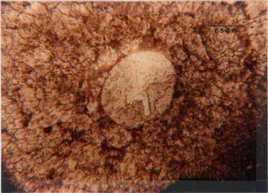
Figure 40. Photomicrograph. Equant spar filling Chara axis. Sample Kmb 79-71; center, NE $\frac{1}{4}$ , NE $\frac{1}{4}$ , Section 19, T. 15 S., R. 9 W. Plane light.
