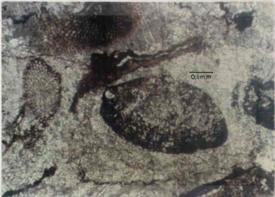
Figure 26. Greater magnification of calcite clast (c) in Figure 25 showing algal borings. Plane light.
