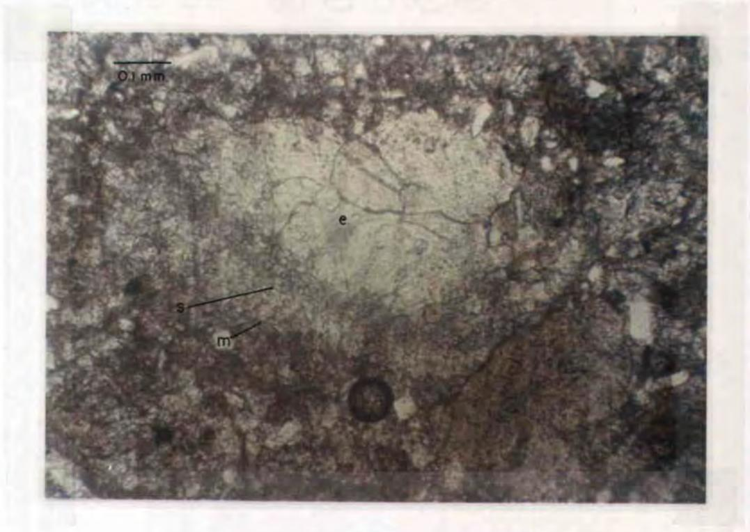
Figure 15. Cementation in calcareous siltstone, Woodside Formation. Photomicrograph showing a layer of micrite (m) lining bottom of pore, scalenohedral spar (s) normal to lower pore wall, equant spar (e) filling the pore. Sample Kmb 79-12a, NE $\frac{1}{4}$ , NW $\frac{1}{4}$ , SW $\frac{1}{4}$ , Section 17, T. 15 S., R. 9 W. Plane light.
