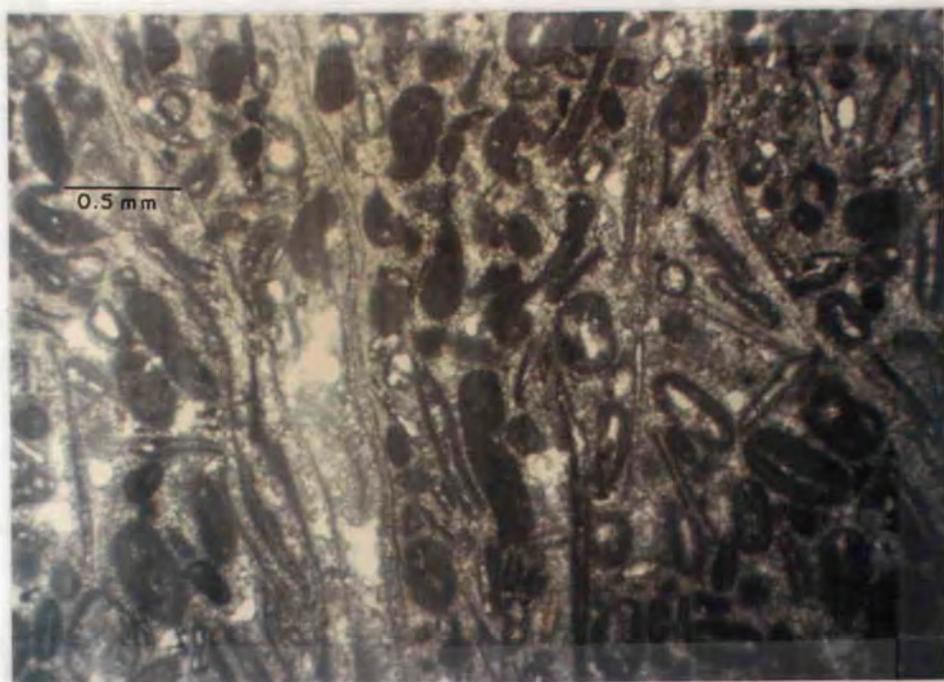
Figure 18. Photomicrograph, mixed oolitic biosparite of the Woodside Formation. Sample 79-114, NE $\frac{1}{4}$ , Section 5, T. 15 S., R. 9 W. Plane light.
