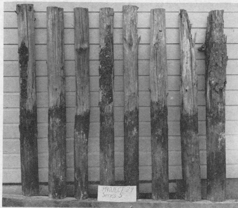
Figure 4. Condition of Douglas fir posts ( left ) and cross sections ( right ) taken at different distances above and below the ground line after 27 years of service. These posts were treated by backfilling with Anaconda Copper Mining Company treater dust.
