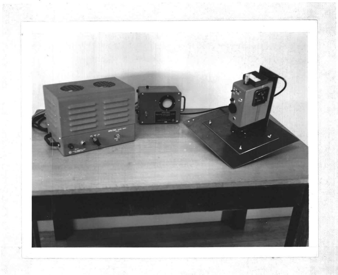
Figure 11. Spectra "Brightness Spot Meter" showing power supply, regulated brightness source and detector mounted on adapter.
