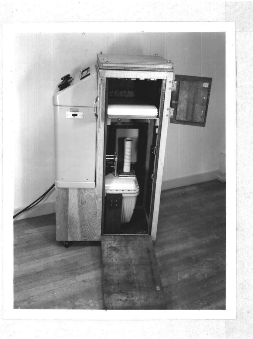
Figure 6. Special X-ray unit with front panels open and screen exposure holder intercepting the beam.
