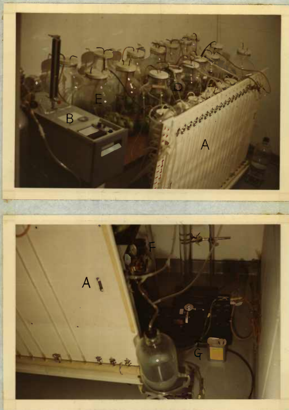
Figure 1. Apparatus used to measure fruit respiration. (A) flow board, (B) Beckman CO 2 infrared analyzer, (C) flow meter, (D) respiration chamber, (E) Jars containing fruits for chemical analyses, (F) Ethylene cylinder, (G) Sigma flexible tubing pump.
