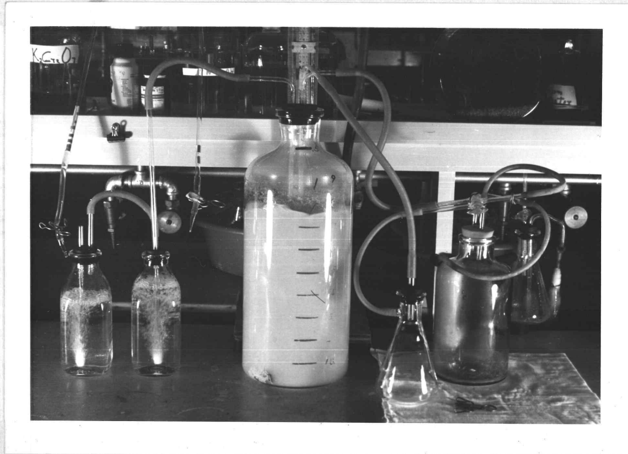
Activated sludge apparatus
