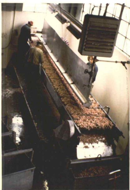
Figure 26. Sorting of trash fish and unwanted objects from shrimp.
