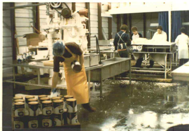
Figure 43. Cans are sealed by a can seamer.
