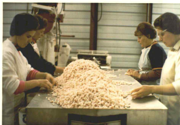
Figure 42. Shrimp meat is inspected and packed in five-pound cans.
