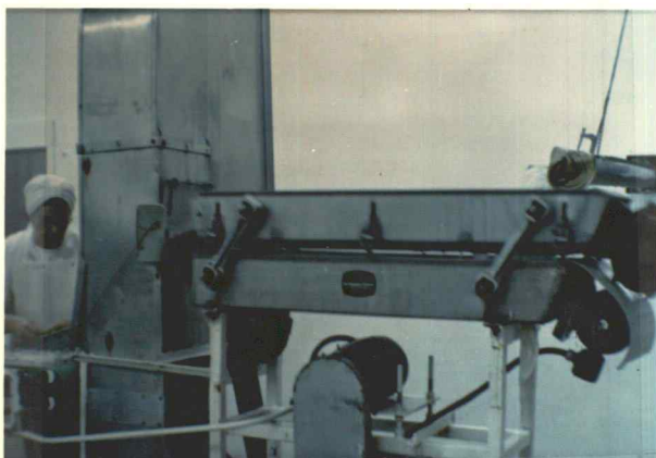
Figure 52. Shrimp meat is flumed into a de-water shaker.
