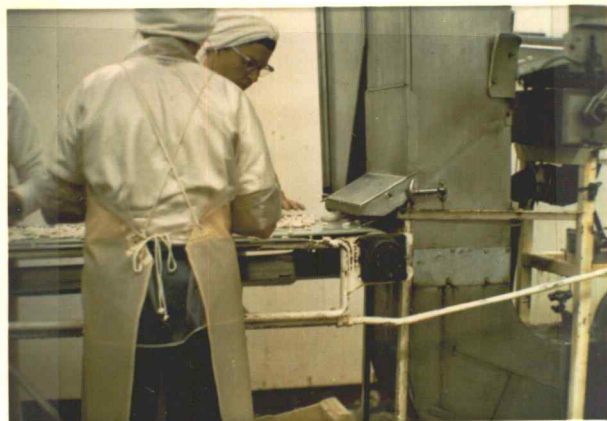
Figure 53. Shrimp meat is cleaned by an air-blower.
