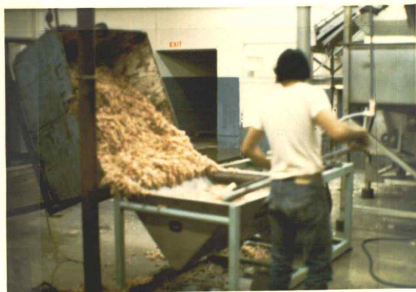
Figure 47. Shrimp are dumped into a food pump.
