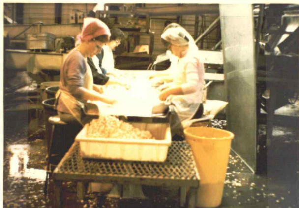
Figure 41. Shrimp meat is inspected on a shaker table.
