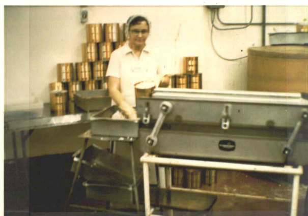
Figure 55. Shrimp meat is brined, de-watered and packed.
