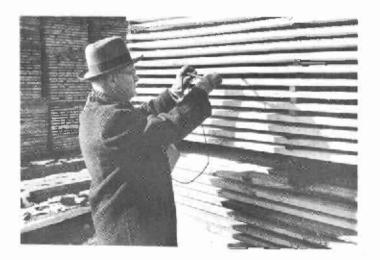
2. The electrode is slipped into the space between the layers of lumber, the Thandle is then twisted to drive the electrode pins into the bottom of the board.
