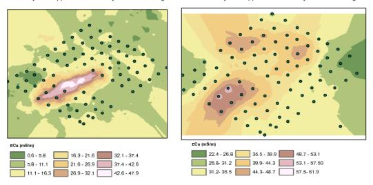
Figure 10. Apparent conductivity (EC<sub>a</sub>) readings in milliSiemens per meter (mS/m) from EMI on playa # 295 in the year 2008, before rehabilitation activities and in 2009 after rehabilitation activities. In each year, EC<sub>a</sub> readings were taken at a shallow depth of 50cm and a deep level of 1 meter. The dots represent sampling points from 2009 and are displayed in all images for reference purposes.
