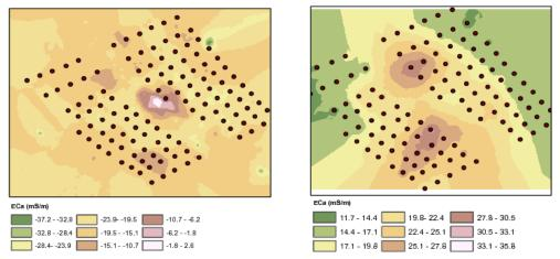
Figure 11. Apparent conductivity ( $EC_a$ ) readings in milliSiemens per meter (mS/m) from EMI on Ram Lake NE playa in the year 2008, before rehabilitation activities and in 2009 after rehabilitation activities. In each year,  $EC_a$  readings were taken at a shallow depth of 50cm and a deep level of 1 meter. The dots represent sampling points from 2009 and are displayed in all images for reference purposes.
