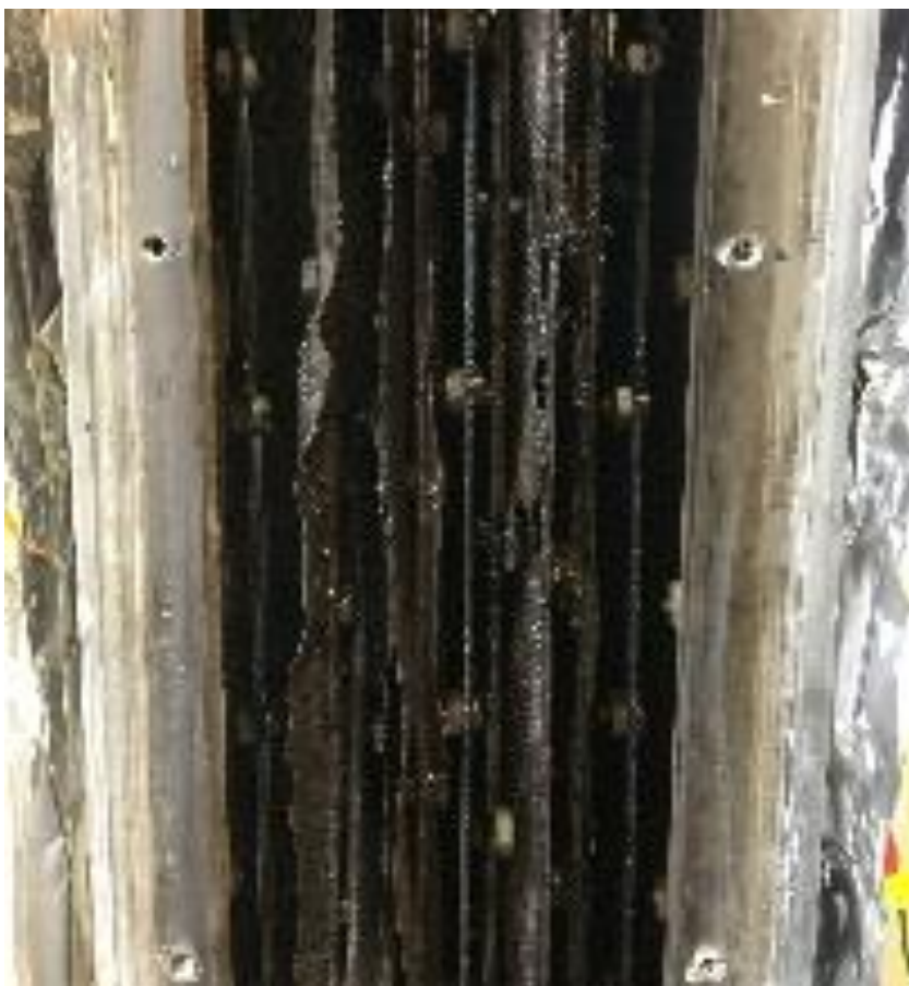
Figure 3.8: Front view of 5C configuration, showing electrode spacing, separator cloth, fasteners
