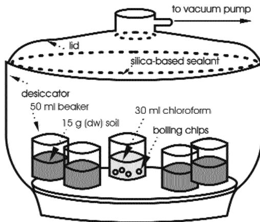
**Fig. 7.** A general set up for the chloroform fumigation extraction (Okalebo et al., 1993).
