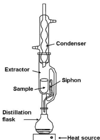
**Fig. 8.** Schematic diagram of a Soxhlet extractor (Arisa and Morada, 2006).
