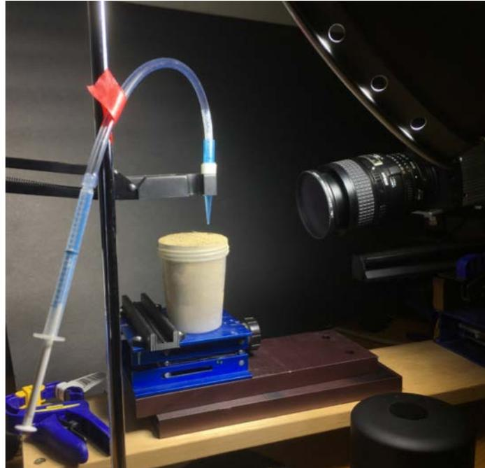
**Fig. 4.** WDPT, and contact angle set up with the high-speed camera.
