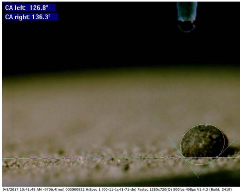
**Fig. 6.** Screenshot of the SCA20\_U program (DataPhysics Instruments GmbH, Filderstadt, Germany) used for contact angle measurements.
