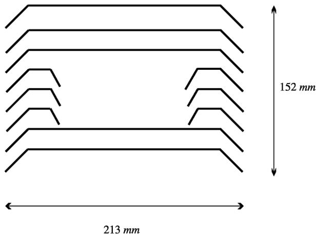
FIG. 3. Cross section of Davis Instruments multiplate shield model 7714 (Onset Computer Radiation Shield RS1). Dimension of the shield is 213 mm (length)  $\times$  188 mm (depth)  $\times$  152 mm (height). Individual plates are 3 mm thick. All of the plates are separated by 15 mm, except for the top two, which are separated by 20 mm. The vertical overlap between a plate and the one underneath is 4 mm.
