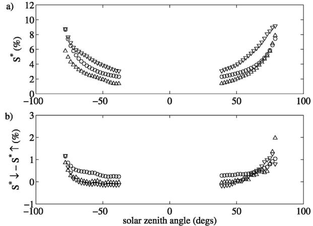
FIG. 4. (a) Mean shortwave radiation ratio  $\bar{S}^*$  (%), and (b) difference between the downward shortwave radiation ratio and the upward shortwave radiation ratio  $S^{*\downarrow} - S^{*\uparrow}$  (%) for grass-covered (o), black ( $\Delta$ ), and white ( $\nabla$ ) surfaces. Negative (positive) sign in the solar zenith angle indicates before (after) solar noon.
