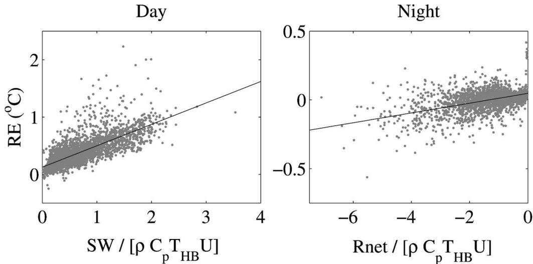
FIG. 7. HOBO radiative error as a function of nondimensional radiation forcing  $X$ . For display, the radiation forcing in the horizontal axes has been multiplied by  $10^3$  and  $10^4$  for day and night, respectively. SW and Rnet stand for shortwave and net radiation, respectively. Lines indicate regression lines based on the coefficients in Table 3.
