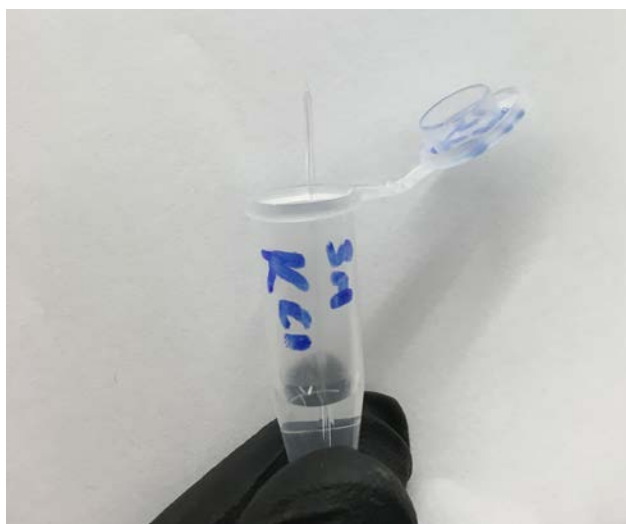
Figure 9 We backfill pipettes in our lab by putting the wide base in a 1.5 mL Eppendorf tube that's been filled with about 1 mL of 3 M KCl. This is an important step for ensuring the electrolyte fills the entire interior of the glass. If this step is skipped, there will be air in the tip and we cannot make recordings. After the glass is backfilled, the researcher can directly fill the rest of the glass (details in the "Methods" section)
