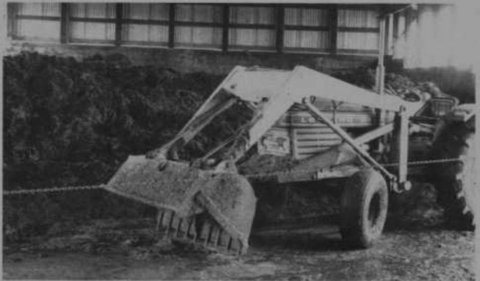
Figure 2. Heavily bedded manure is collected and handled as a solid with the tractor-mounted front-end loader. The solid manure is stored in a bunker-type covered building.
