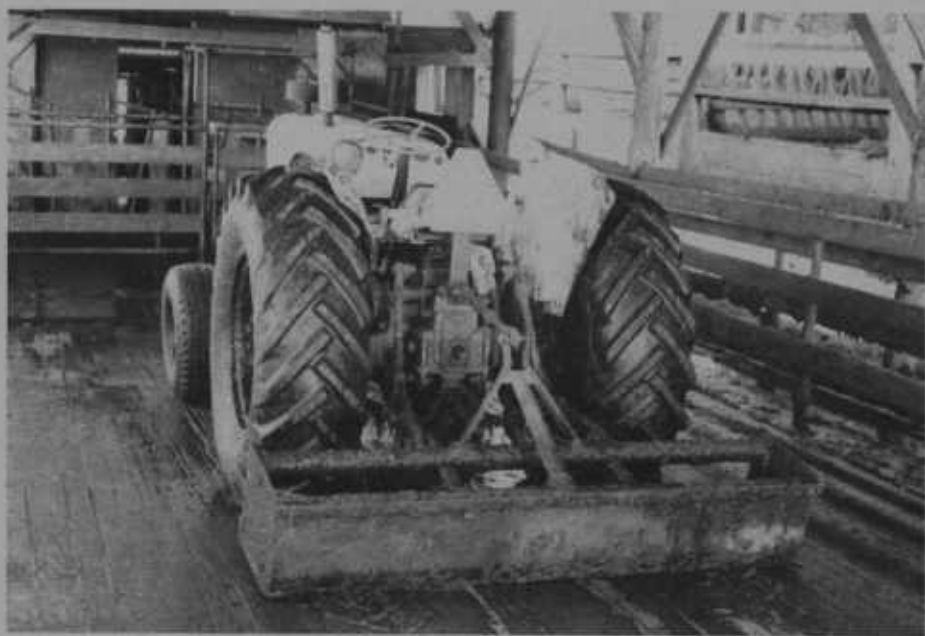
Figure 1. A rear-mounted tractor-scraper is commonly used to collect manure on dairy operations.
