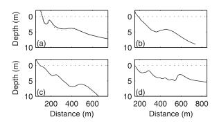
**Figure 1.** Depth versus cross-shore distance at (a) Duck (28 August 1998), (b) Miyazaki (1999), (c) the Gold Coast (6 September 1973), and (d) Noordwijk (29 July 2002). Note that the profiles in Figures 1b and 1d were surveyed well before the periods analyzed here and that the bars may thus be positioned at a different location than estimated from the Argus images. The solid (dotted) line in Figure 1a was measured north (south) of the FRF pier.
