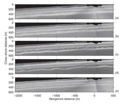
**Figure 8.** Plan view images on (a) 25 February 2003 2300 UT, (b) 27 February 2003 0600 UT, (c) 1 March 2003 0400 UT, (d) 19 March 2003 0300 UT, and (e) 21 April 2003 2200 UT at the Gold Coast, showing the temporal development of alongshore nonuniformities in the inner bar; see text for further explanation.
