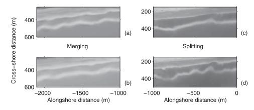
**Figure 12.** Example of the (left) merging and (right) splitting of individual crescents in the outer bar at the Gold Coast. In the merging event the crescent with its bay near y = -1650 m vanished, whereas in the splitting event a new crescent developed between y = -500 and -650 m. Images were collected on (a) 11 March 2003 0700 UT, (b) 12 March 2003 0700 UT, (c) 19 March 2003 0500 UT, and (d) 26 March 2003 0000 UT.
