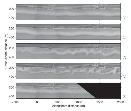
**Figure 7.** Plan view images on (a) 22 September 2001 0700 UT, (b) 23 September 2001 0700 UT, (c) 25 September 2001 0100 UT, (d) 1 October 2001 0200 UT, and (e) 19 October 2001 0600 UT at Miyazaki, showing the temporal development of crescentic bars; see text for further explanation.
