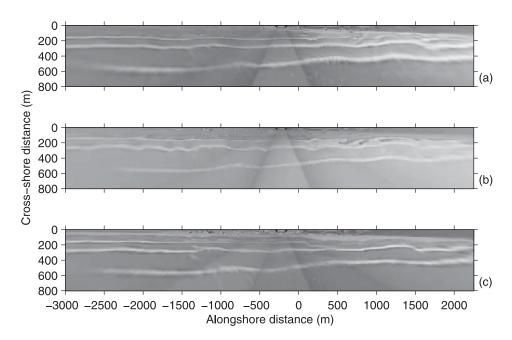
**Figure 9.** Plan view images on (a) 28 February 2002 1200 UT, (b) 20 March 2002 1300 UT, and (c) 14 May 2002 1000 UT at Noordwijk, showing the temporal development of crescentic shapes in the inner bar ( $x \approx 250$  m); see text for further explanation. In Figure 9b, secondary features are particularly obvious around y = -2750, -1500, and -750 m. Notice the similarity in inner-bar crescents in Figures 9a and 9c.
