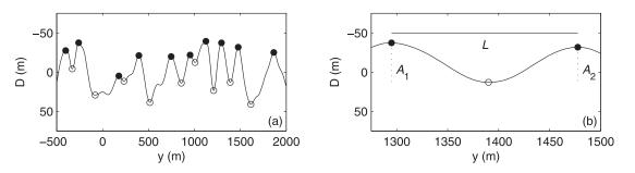
**Figure 2.** (a) Example of a bar crest line with detected (filled circles) horns and (open circles) bays. (b) A single crescent from Figure 2a with length L and amplitude  $A = 0.5 \times (A_1 + A_2)/2$ .
