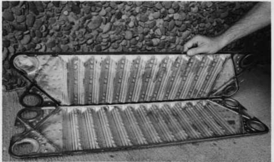
Figure 5b. —A neoprene gasket seals the edges of these heat exchanger plates.
