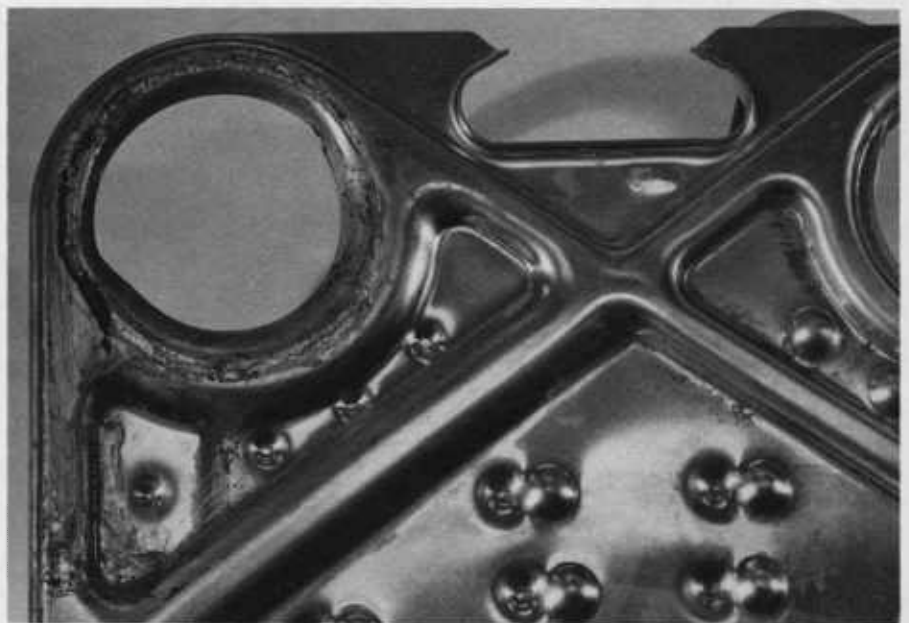
Figure 5c. —Crevice corrosion in several areas under the gasket of these 316 stainless heat exchanger plates has penetrated the thickness.
