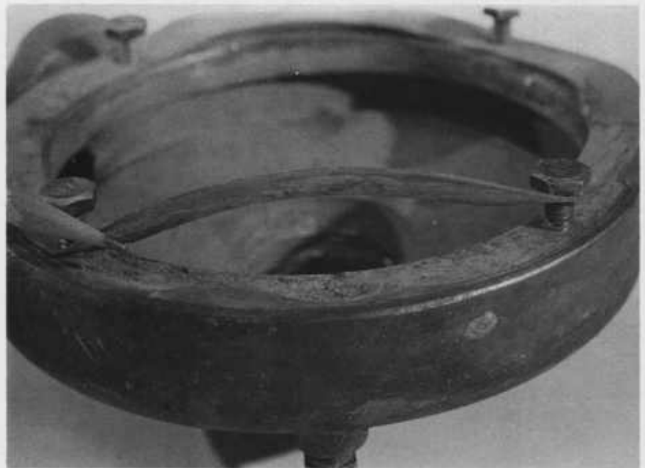
Figure 2.—Pitting has appeared under the gasket on this 316 stainless pump housing.
