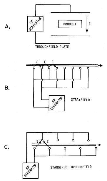
Figure 5. Various arrangements of radiofrequency electrodes used in industry.
