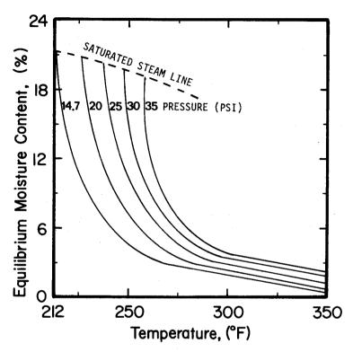
Figure 3. Equilibrium moisture content of wood versus temperature at various pressures (Rosen, 1983).
