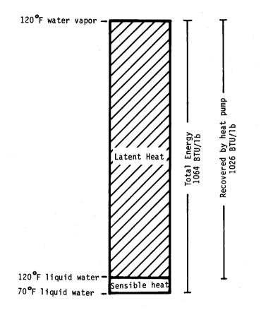
Figure 2. Energy in liquid and vapor water leaving the kiln at  $120^{\circ}F$ . A heat pump recovers the shade portion.
