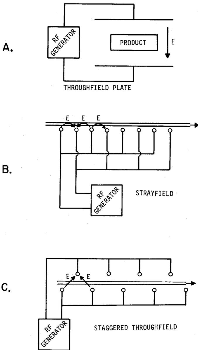
Figure 5. Various arrangements of radiofrequency electrodes used in industry.
