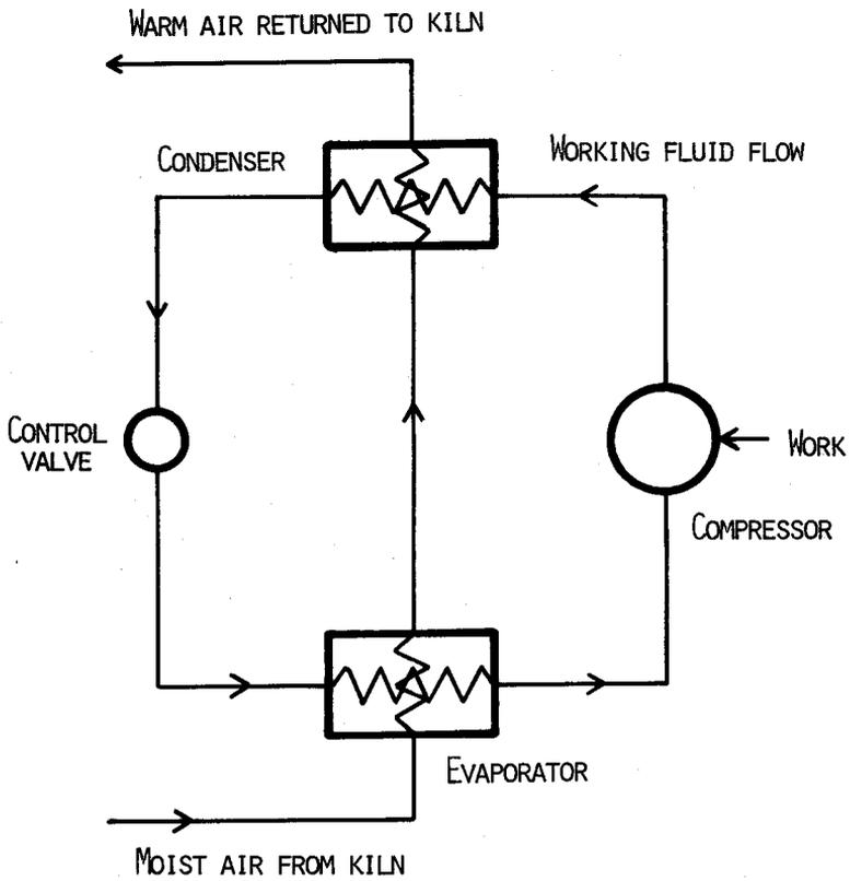
Figure 1. Schematic of kiln vapors and working fluid flows in a dehumidification dryer.
