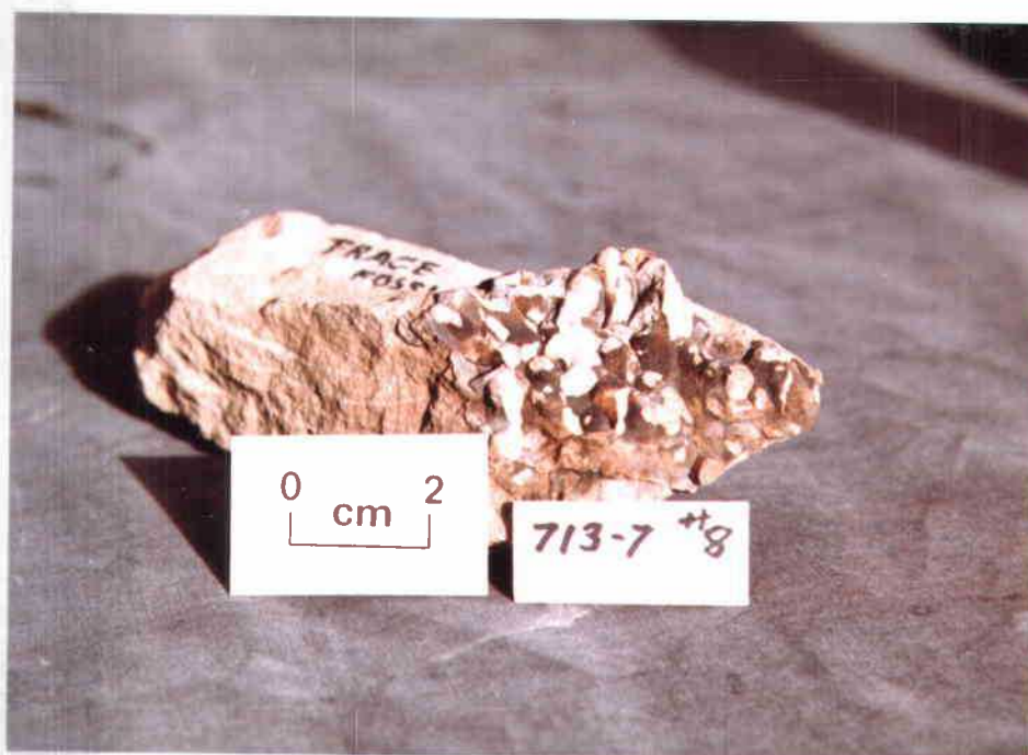
Figure 33: Sand filled Teredo borings within darker carbonized wood in Pittsburgh Bluff sandstone. (OC 713-7, sec. 13-T6N-R7W).
