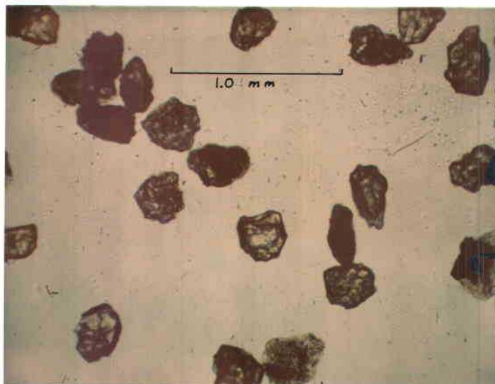
Figure 19: Photomicrograph of heavy mineral assemblage from "epidote-rich" upper Cowlitz sandstone member (Tc 5 ). Note typical "broken-glass" appearance of pistachio green epidote grains which comprises 90% of the grains in the slide. Plane polarized light. Sample 825-7 #3.
