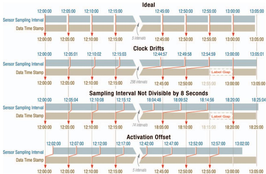
**Figure 1.** Sources of timing error (Clock Drifts, Sampling Interval Not Divisible by 8 Seconds, and Activation Offset) result in sensor sampling intervals time stamped with incorrect start times for remotely sensed behavior data collected using dual-axis accelerometer activity sensors mounted on Lotek GPS\_4400 collars. Accumulation of many small errors can result in a gap in the data time stamps (label gap) which starts the cycle of error accumulation anew.
