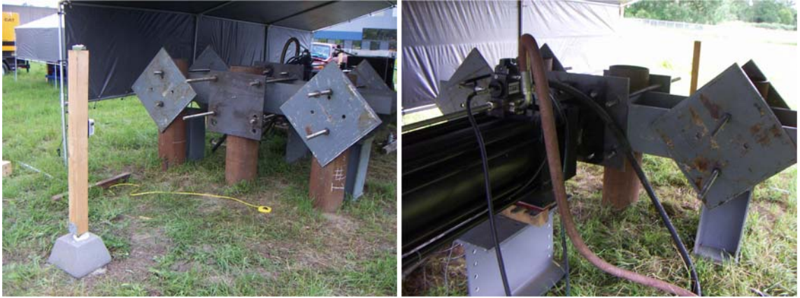
Figure 3-11 Actual Test Set-up – Three-in-a-row Reaction Pile Arrangement
