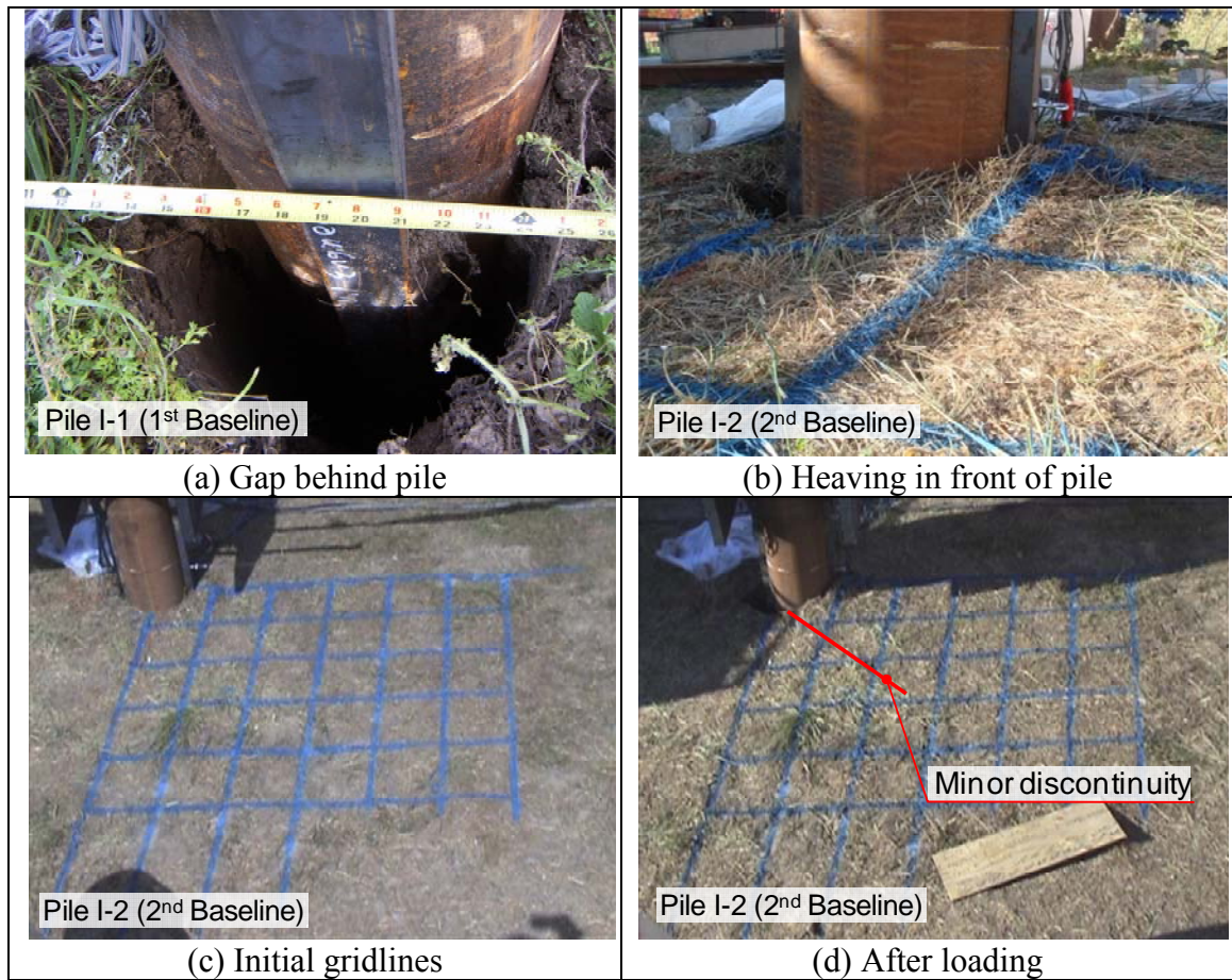
Figure 4-1 Observations during the Lateral Loading Tests for the 1 st and the 2 nd Baseline Piles (Free-Field)
