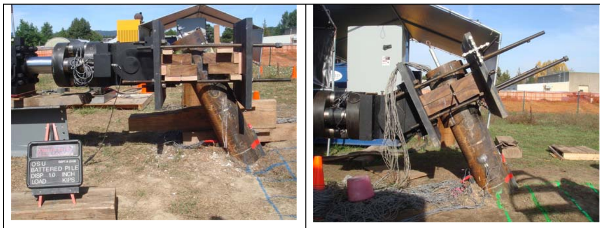
Figure 4-7 First Attempt (left) and Second Attempt (right) for the Battered Pile Test (I-3)
