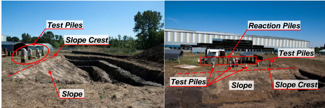
Figure 3-12 Overall View of the Completed Slope Excavation (Stage 3)
