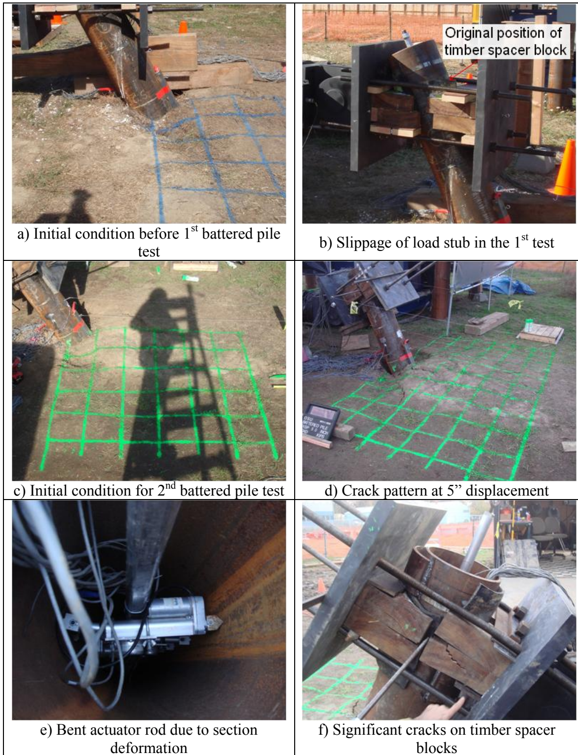
Figure 4-8 Observations during the Lateral Loading Test for the Battered Pile (I-3)
