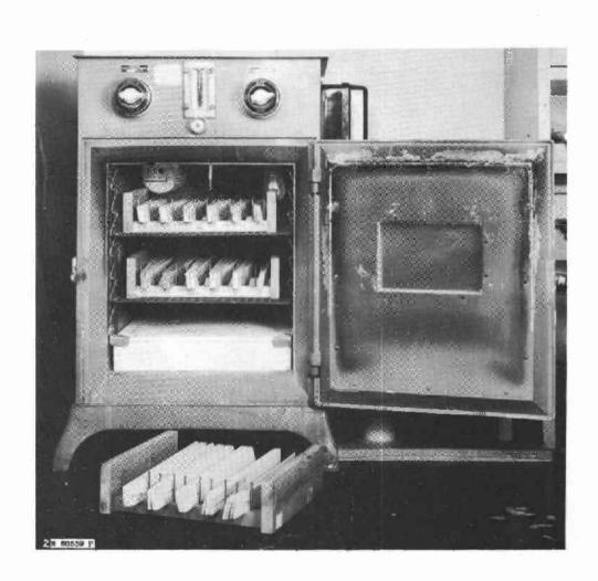
Figure 2.—Mandrels used in making bending tests on veneer to determine whether its slopes of grain from the plane of the sheet are permissible for aircraft plywood. These included most of the sizes needed for testing hardwood species of veneer.
