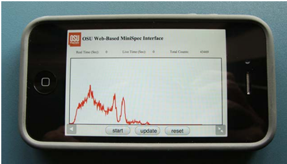
4 Figure 5. Mobile phone displaying gamma spectrum from ^{137}\text{Cs} and ^{22}\text{Na} sources as collected by 5 the MiniSpec.
