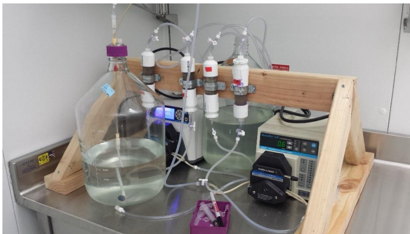
Figure 1. Experimental setup of four UFCs in parallel.
