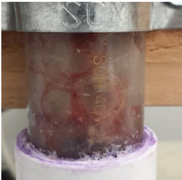
Figure 3. Anammox biofilm on swollen 10% PVA gel in UFC.
