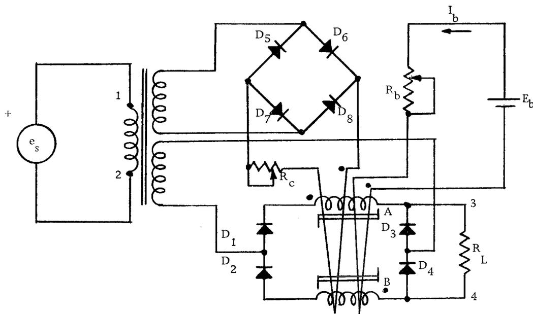
Figure 8. A Self-saturating Magnetic Amplifier
