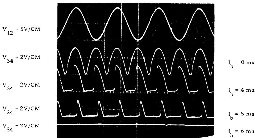
Figure 9. Magnetic Amplifier Waveforms
