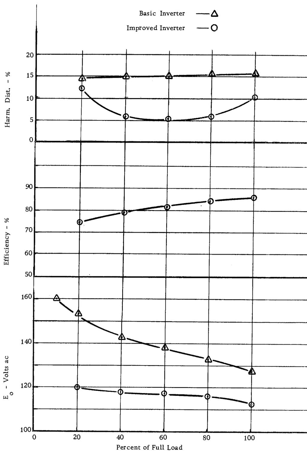
Figure 16. Output Voltage, Efficiency and Distortion
