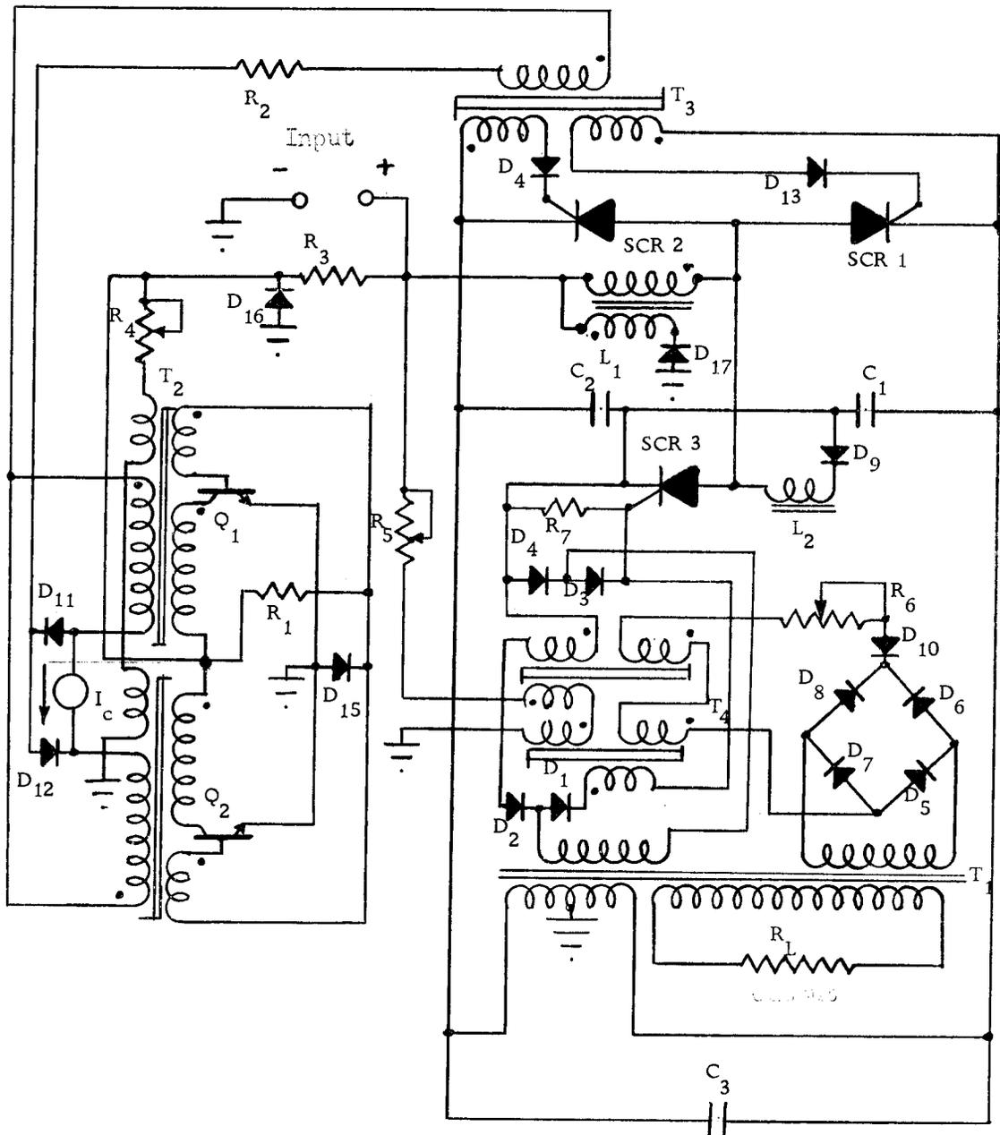
Figure 7. Voltage Regulated Inverter Circuit
