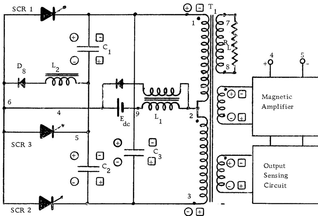
Figure 10. Simplified Inverter Schematic
