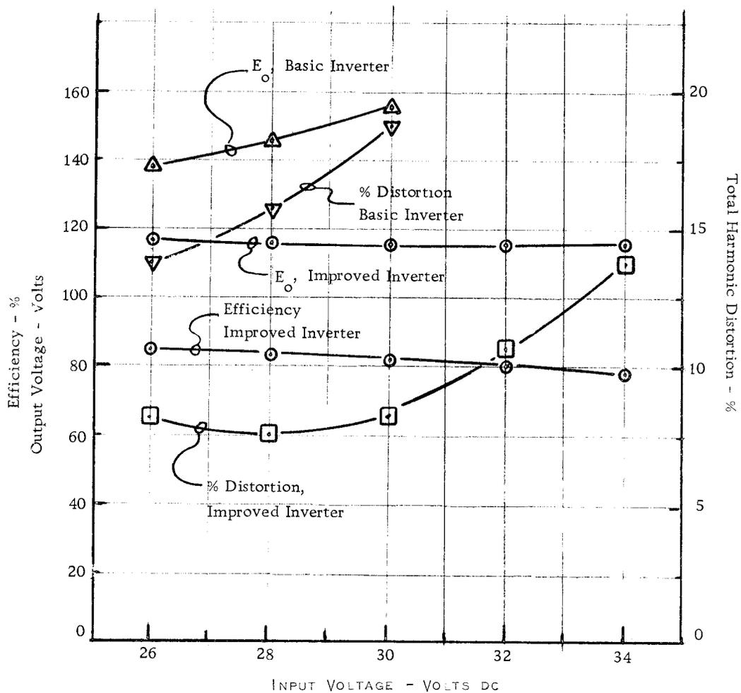
Figure 15. Regulation, Efficiency and Distortion Curves
