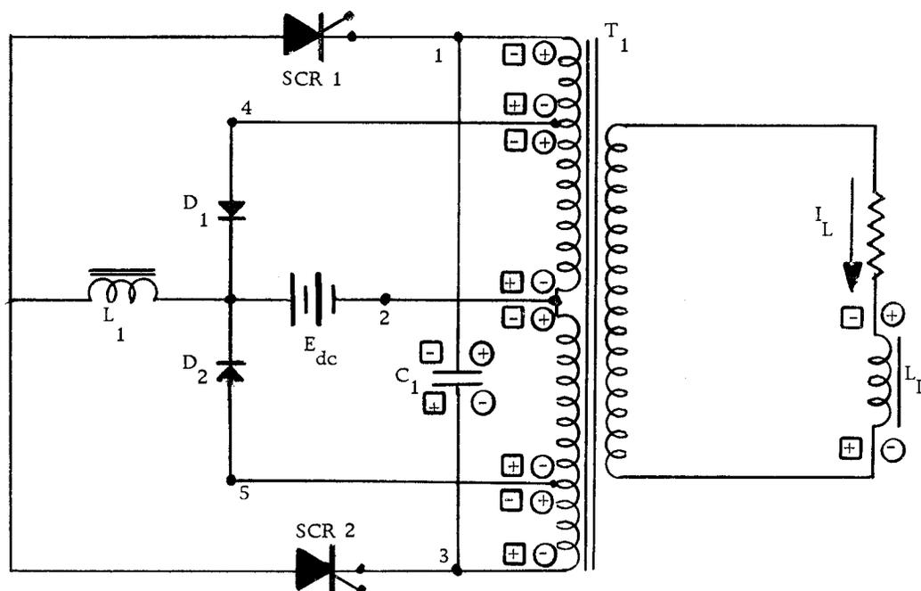
Figure 6. McMurray Parallel Inverter
