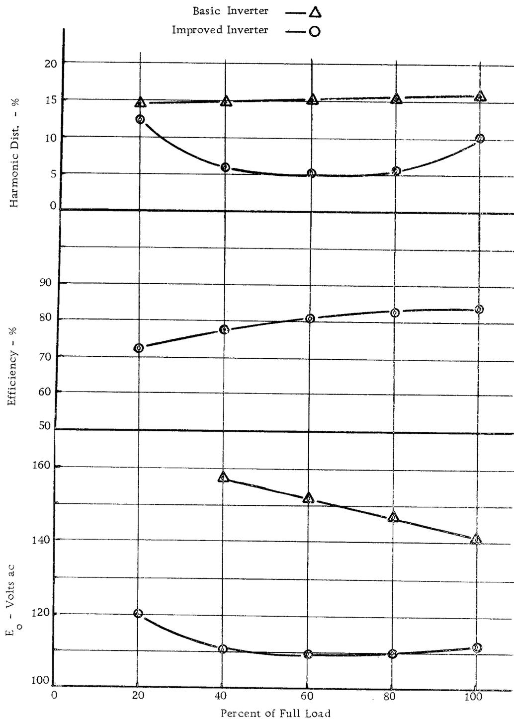
Figure 17. Output Voltage, Efficiency and Distortion
