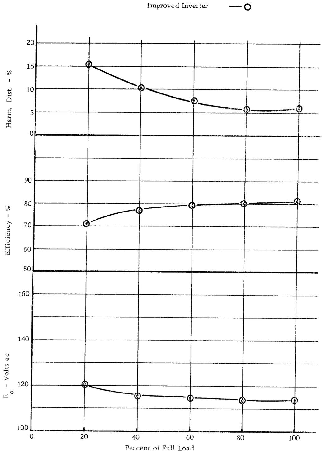
Figure 18. Output Voltage, Efficiency and Distortion
