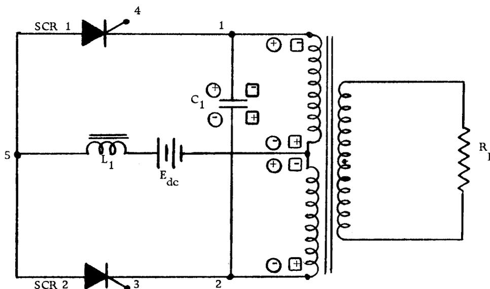
Figure 4. Basic Parallel Inverter Circuit
