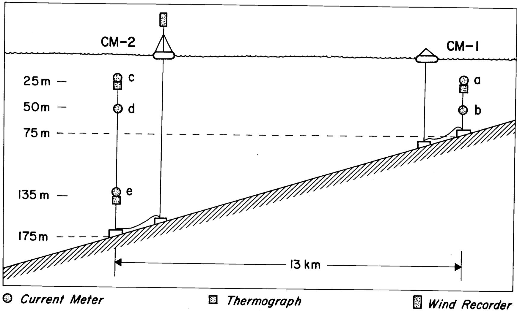
Figure 2. Configuration of the moored instrument array.
