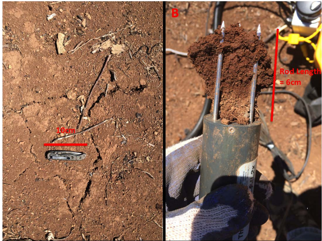
Figure 15. Peak summer soil characteristics on forest floor removal and compaction treatment at an LTSP site in Springfield, OR. (A) Cracks were visible due to shrinking of soil only on forest floor removal plots, (B) evaporation due to direct solar radiation in August of 2014 (highest soil temperatures) only reached the upper 3cm.
