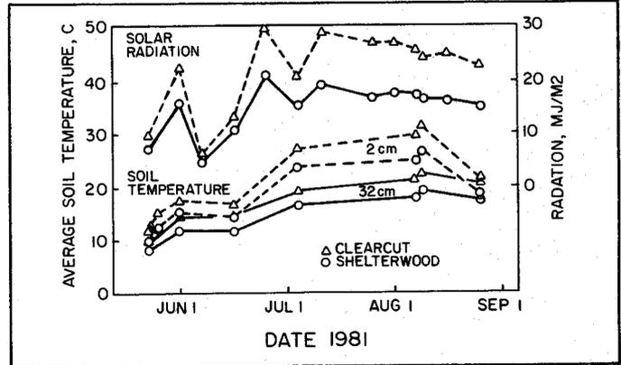
Figure 1. Shelterwood - clearcut comparison of soil temperature and radiation.
