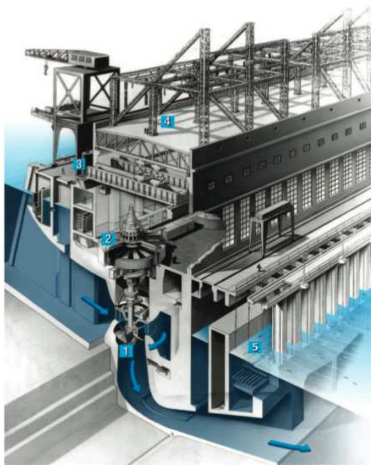
Figure 4.12. Diagram of hydropower facility, showing a single unit (from US Army Corps of Engineers).
