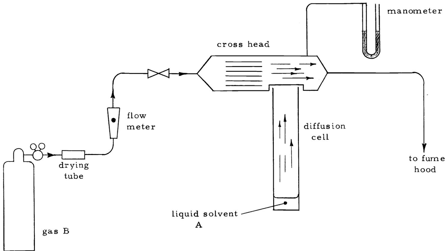
Figure 5. Schematic flow diagram of gaseous components.
