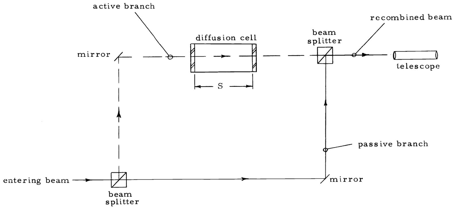
Figure 2. Schematic representation of Mach-Zender interferometer.
