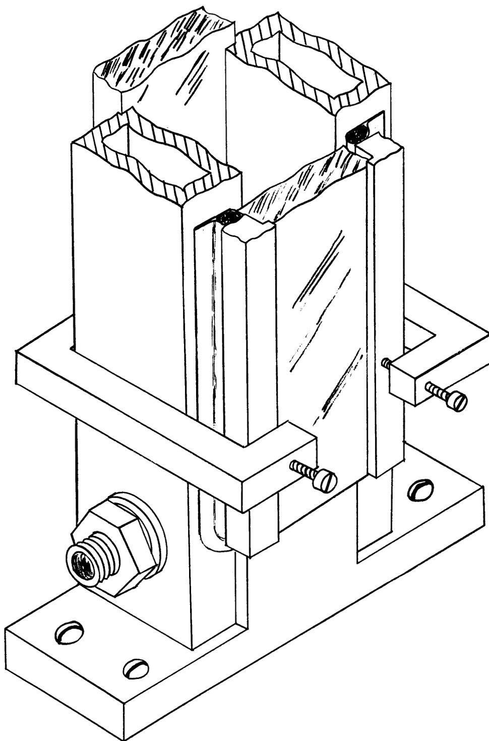
Figure 4. Detailed configuration of diffusion cell (scale 1-1/2 to 1).
