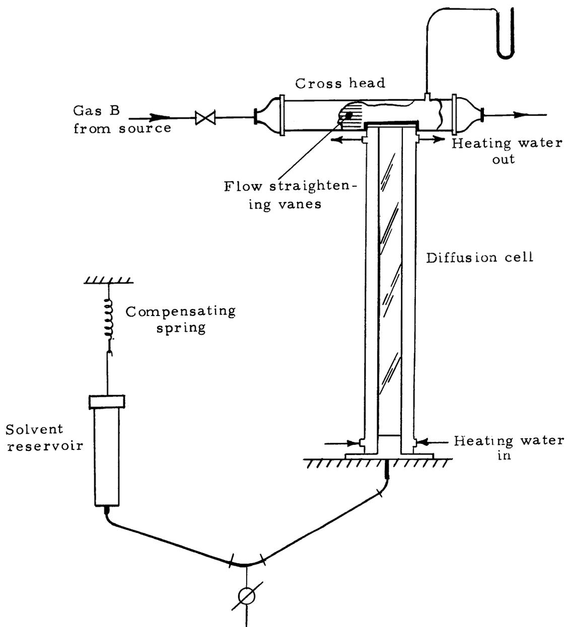
Figure 3. Representation of integrated diffusion cell subsystem.
