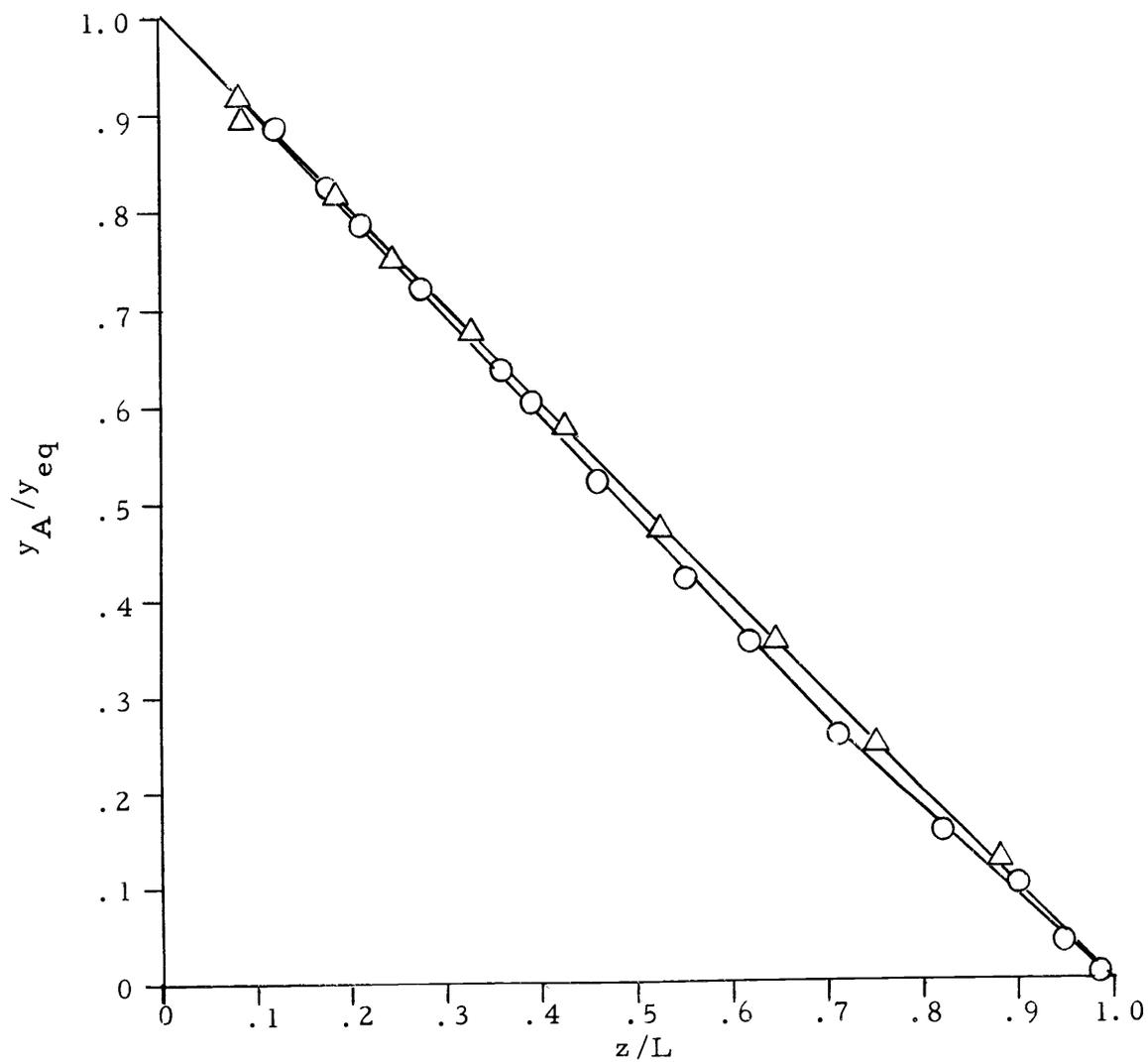
Figure 10. Composition profiles of benzene-air and benzene-nitrogen systems.
