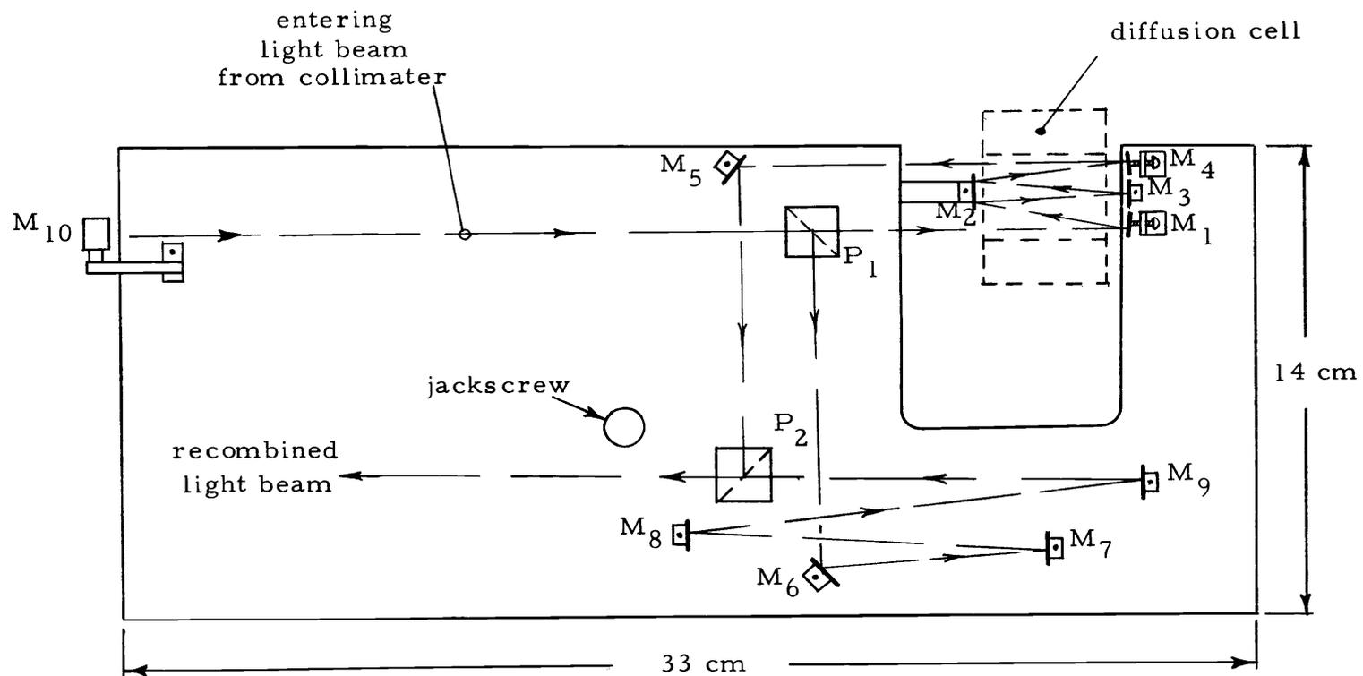
Figure 6. Layout of optical interferometer platform (scale 1/2 to 1).
