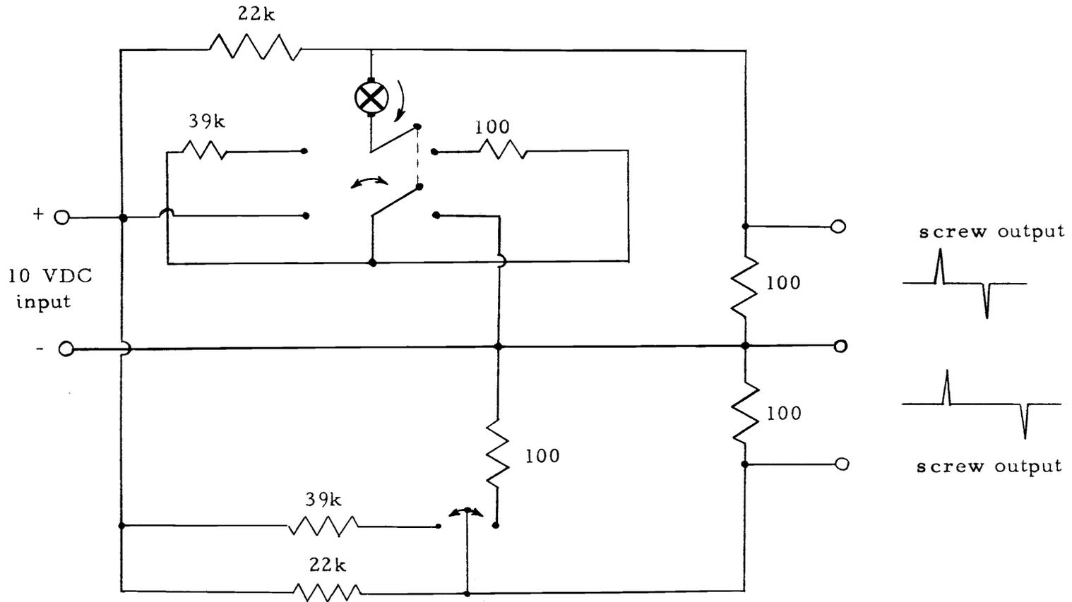
Figure 13. Counting pulse generating circuit.
