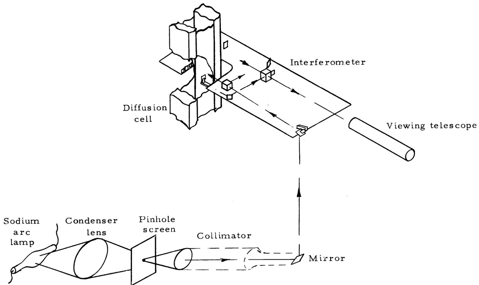
Figure 7. Layout of integrated optical subsystem.
