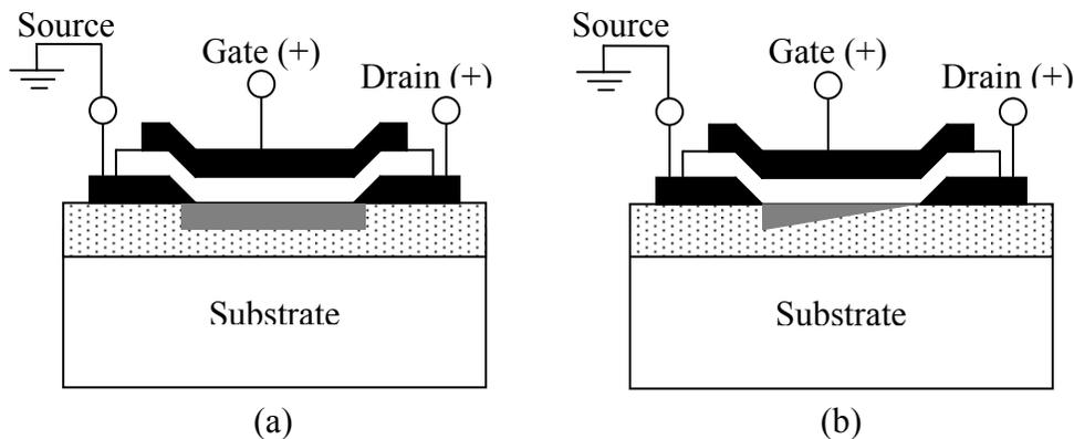
Figure 2.4: An n-channel accumulation-mode TFT operating in (a) pre-pinch-off and (b) post-pinch-off regime.
