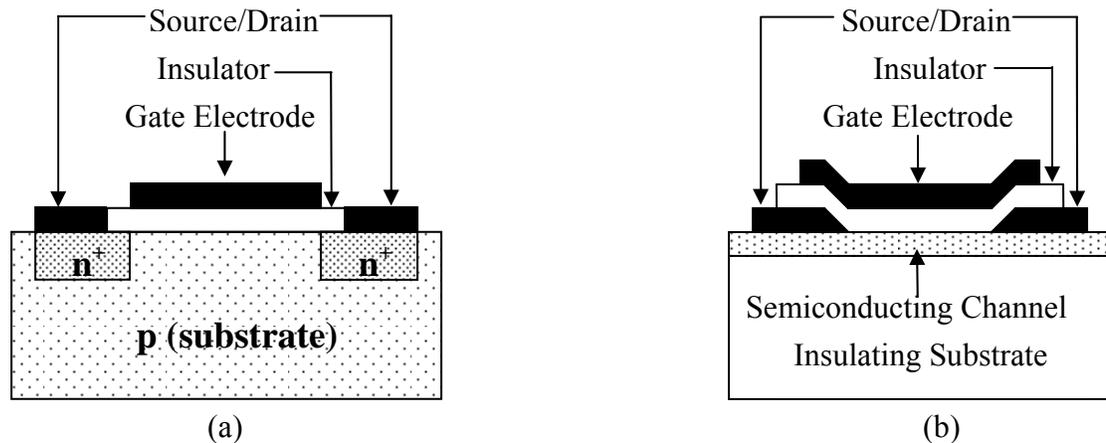
Figure 2.1: Cross-sectional schematic drawing of a (a) MOSFET and (b) TFT.
