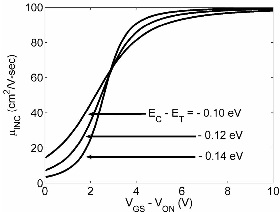
Figure 3.16: Simulated  $\mu_{INC} - (V_{GS} - V_{ON})$  as a function of trap depth,  $E_C - E_T$  for trap density of  $N_T = 5 \times 10^{17} \text{ cm}^{-3}$  and a drain voltage,  $V_{DS} = 0.2 \text{ V}$ . Model parameters used for this simulation:  $Z/L = 6:1$ ,  $h = 20 \text{ nm}$ ,  $C_G = 6.04 \times 10^{-8} \text{ F/cm}^2$ ,  $\mu_{BULK} = 100 \text{ cm}^2/\text{V-s}$ , and  $n_{co} = 1 \times 10^{15} \text{ cm}^{-3}$ .
