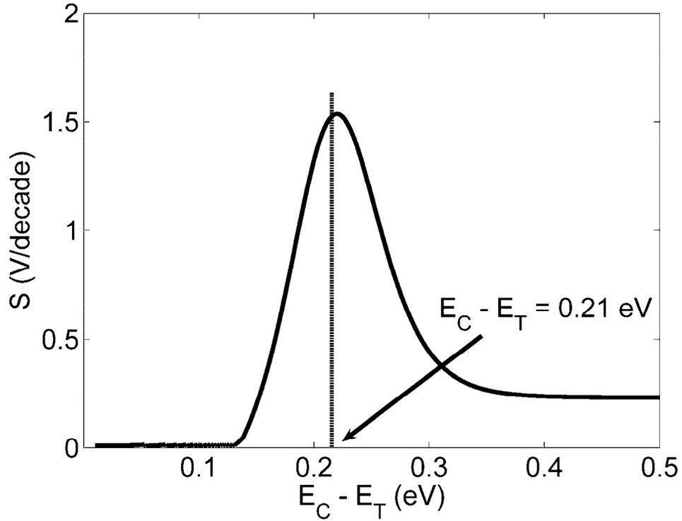
Figure 3.12: Simulated  $S$  as a function of trap depth,  $E_C - E_T$ , at a constant trap density of  $5 \times 10^{17} \text{ cm}^{-3}$ . For this simulation,  $V_{DS} = 1 \text{ V}$ ,  $Z/L = 6:1$ ,  $h = 20 \text{ nm}$ ,  $C_G = 6.04 \times 10^{-8} \text{ F/cm}^2$ ,  $\mu = 100 \text{ cm}^2/\text{V-s}$ , and  $n_{co} = 1 \times 10^{16} \text{ cm}^{-3}$ .
