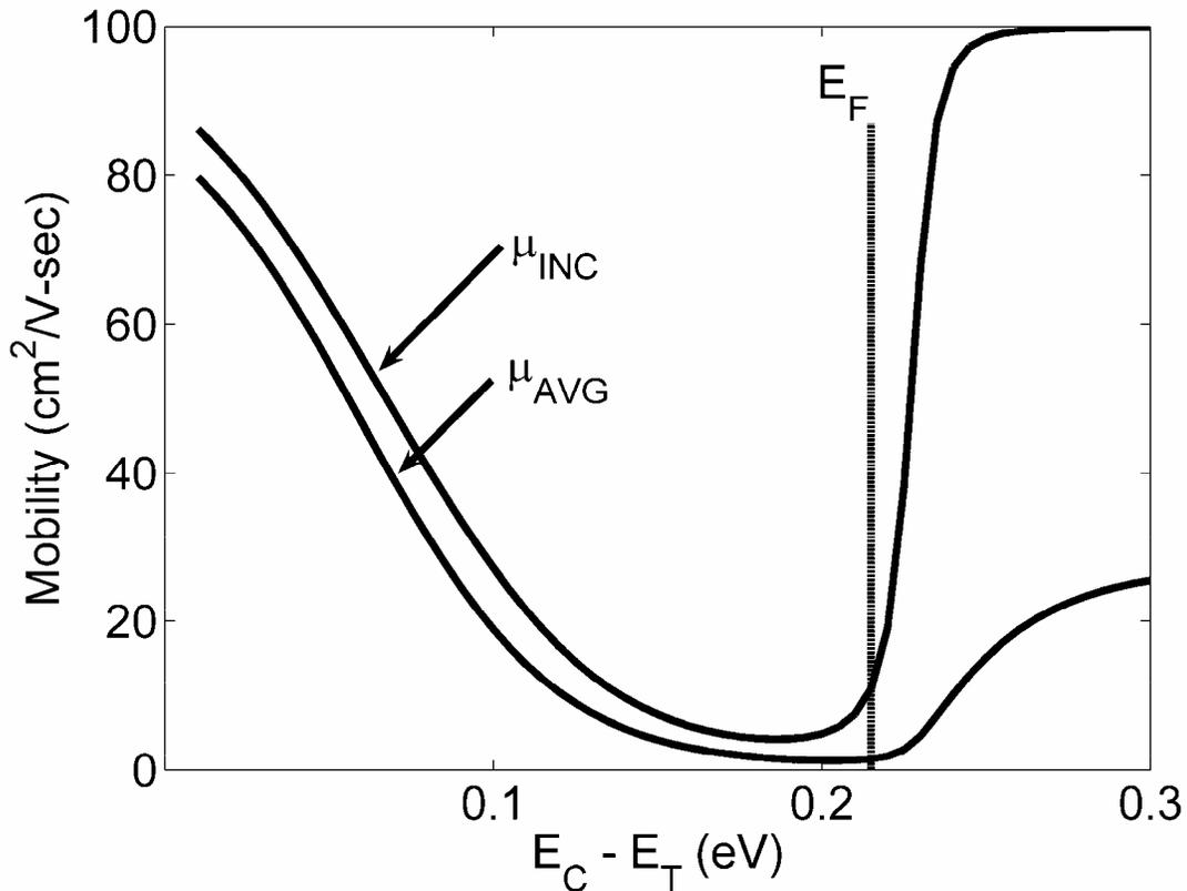
Figure 3.18: Simulated  $\mu_{INC}$  and  $\mu_{AVG}$  characteristics as a function of trap depth,  $E_C - E_T$ . The Fermi level,  $E_F$ , as established by the initial free carrier concentration is 0.21 eV below the conduction band minimum,  $E_C$ . Model parameters used for this simulation:  $Z/L = 6:1$ ,  $h = 20$  nm,  $C_G = 6.04 \times 10^{-8}$  F/cm<sup>2</sup>,  $\mu_{BULK} = 100$  cm<sup>2</sup>/V-s, and  $n_{co} = 1 \times 10^{15}$  cm<sup>-3</sup>.
