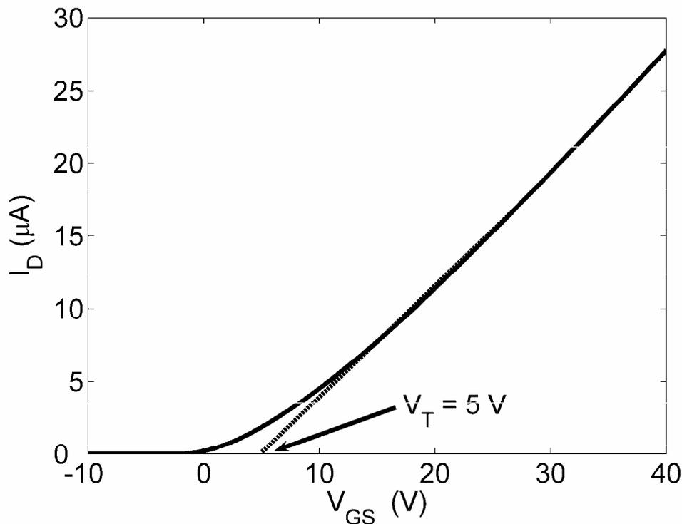
Figure 3.6: Drain current-gate voltage ( $I_D$ - $V_{GS}$ ) transfer curve for a zinc tin oxide, n-channel TFT. The threshold voltage is estimated to be  $\sim 5$  V via extrapolation of the linear portion of this curve. Geometrical parameters for this TFT are  $Z/L = 5:1$  and  $C_G = 3.45 \times 10^{-8}$  F/cm<sup>2</sup>.
