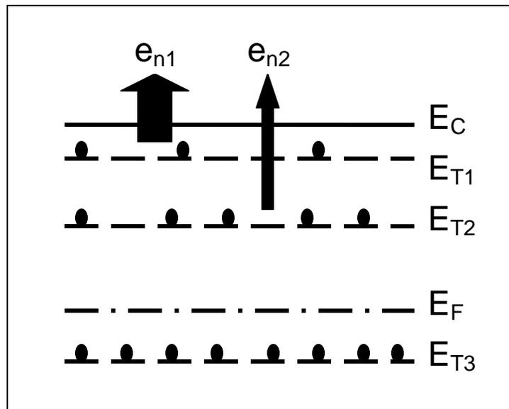
Figure. 3.3: Energy-band diagram of the upper band gap portion of the semiconductor at a flat band. Three discrete traps are present at  $E_{T1}$ ,  $E_{T2}$ , and  $E_{T3}$  with respect to the conduction band minimum,  $E_C$ .  $E_F$  determines the trap occupancy, which is qualitatively indicated by the fraction of the trap states occupied by electrons (filled circles). The widths of the arrows represent the relative rate of trap emission.
