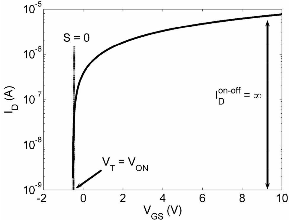
Figure 3.8: Log ( $I_D$ )- $V_{GS}$  transfer curve simulation using the square-law model. In this ideal case,  $S = 0$  V/decade,  $V_T = V_{ON}$ , and the drain current on-to-off ratio is infinite. For this simulation  $T = 300$  K,  $V_{DS} = 100$  mV,  $Z/L = 6:1$ ,  $h = 20$  nm,  $C_G = 6.04 \times 10^{-8}$  F/cm<sup>2</sup>,  $\mu = 100$  cm<sup>2</sup>/V-s, and  $n_{co} = 1 \times 10^{17}$  cm<sup>-3</sup>.
