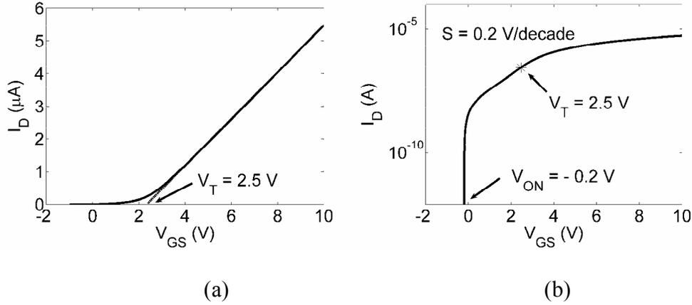
Figure 3.9:  $I_D$ - $V_{GS}$  and  $\log(I_D)$ - $V_{GS}$  transfer curves simulated using the discrete trap model. For this simulation,  $T = 300$  K,  $V_{DS} = 1$  V,  $N_T = 5 \times 10^{17}$   $\text{cm}^{-3}$ ,  $E_T = 0.15$  eV below the conduction band minimum,  $Z/L = 6:1$ ,  $h = 20$  nm,  $C_G = 6.04 \times 10^{-8}$  F/ $\text{cm}^2$ ,  $\mu = 100$   $\text{cm}^2/\text{V}\cdot\text{s}$ , and  $n_{co} = 1 \times 10^{15}$   $\text{cm}^{-3}$ .
