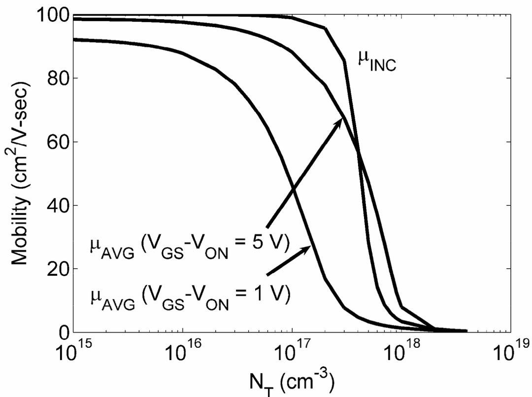
Figure 3.17: Simulated  $\mu_{INC}$  and  $\mu_{AVG}$  characteristics as a function of trap density,  $N_T$ . Model parameters used for this simulation:  $Z/L = 6:1$ ,  $h = 20$  nm,  $C_G = 6.04 \times 10^{-8}$  F/cm<sup>2</sup>,  $\mu_{MODEL} = 100$  cm<sup>2</sup>/V-s, and  $n_{co} = 1 \times 10^{15}$  cm<sup>-3</sup>.
