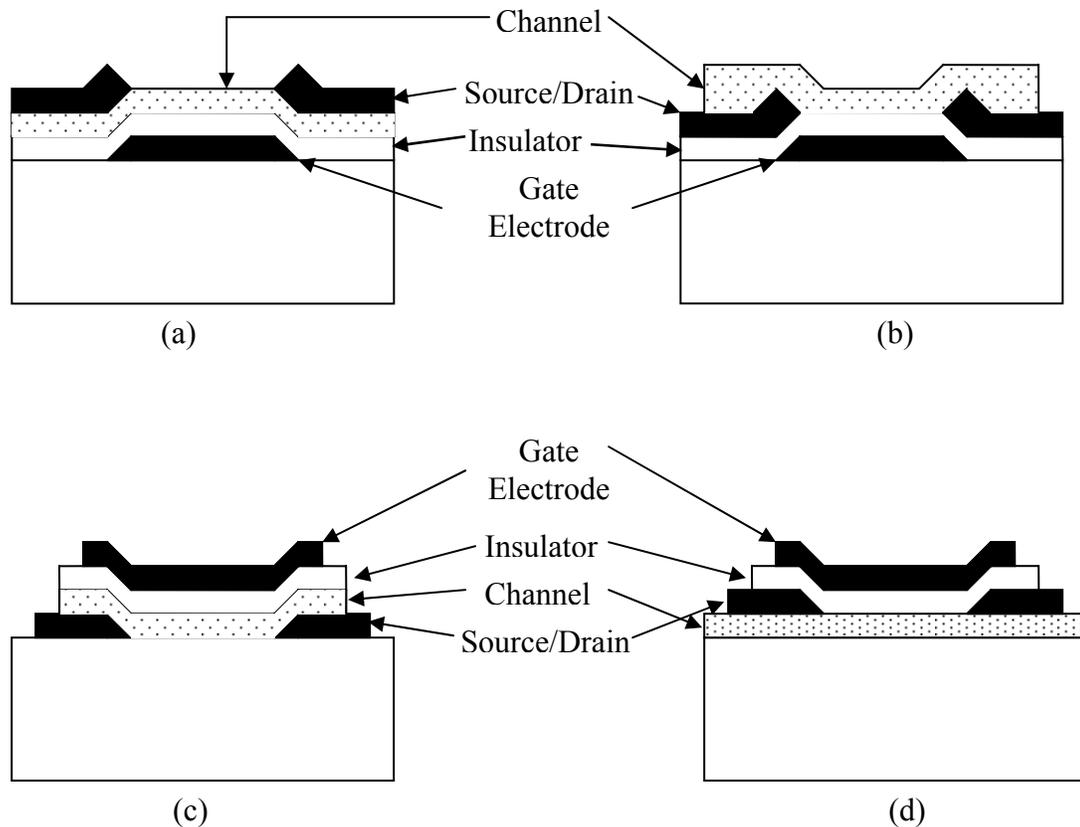
Figure 2.2: Four thin-film transistor configurations: (a) staggered bottom-gate, (b) coplanar bottom-gate, (c) staggered top-gate, and (d) coplanar top-gate.
