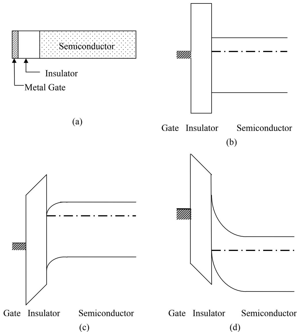
Figure 2.3: (a) The cross-section of a metal-oxide-semiconductor (MOS) capacitor and corresponding energy band diagrams for several biasing conditions: (b) equilibrium, (c) accumulation ( $V_{GS} > 0$  V), and (d) inversion ( $V_{GS} < 0$  V).
