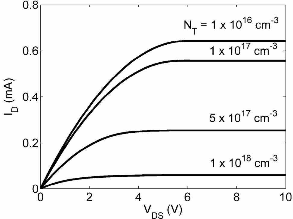
Figure 3.1: Drain current-drain voltage ( $I_D$ - $V_{DS}$ ) characteristics for an n-channel TFT corresponding to a gate voltage of 6 V and a trap depth of  $E_C - E_T = 0.15 \text{ eV}$  below the conduction band minimum. Geometrical and channel-based parameters employed for this simulation are:  $Z/L = 6:1$ ,  $h = 20 \text{ nm}$ ,  $C_G = 6.04 \times 10^{-8} \text{ F/cm}^2$ ,  $\mu = 100 \text{ cm}^2/\text{V}\cdot\text{s}$ , and  $n_{co} = 1 \times 10^{15} \text{ cm}^{-3}$ .
