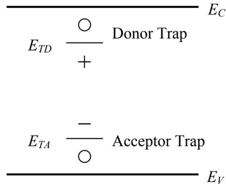
Figure 2.5: Energy band diagram of a bulk semiconductor with a donor-like trap and an acceptor-like trap with ionization energies,  $E_{TD}$  and  $E_{TA}$ , respectively.
