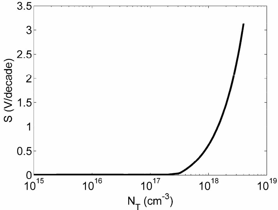
Figure 3.11: Simulated  $S$  as a function of  $N_T$  using the discrete trap model with a constant trap depth of  $E_C - E_T = 0.15$  eV. For this simulation,  $V_{DS} = 1$  V,  $Z/L = 6:1$ ,  $h = 20$  nm,  $C_G = 6.04 \times 10^{-8}$  F/cm<sup>2</sup>,  $\mu = 100$  cm<sup>2</sup>/V-s, and  $n_{co} = 1 \times 10^{15} \text{ cm}^{-3}$ .
