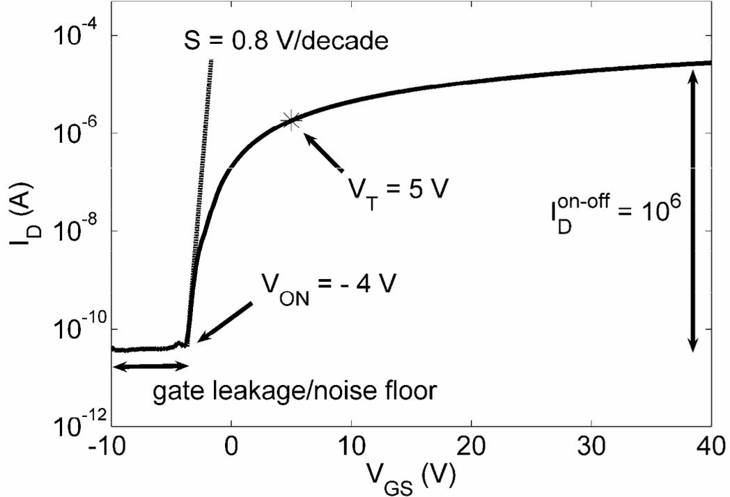
Figure 3.7:  $\text{Log}(I_D)$ - $V_{GS}$  transfer curve for a zinc tin oxide, n-channel TFT. The voltage at which the TFT turns on is  $-4$  V. The previously extracted value of the threshold voltage,  $V_T = 5$  V does not correspond to any obvious drain current onset. Geometrical parameters for this TFT are  $Z/L = 5:1$  and  $C_G = 3.45 \times 10^{-8}$  F/cm<sup>2</sup>.
