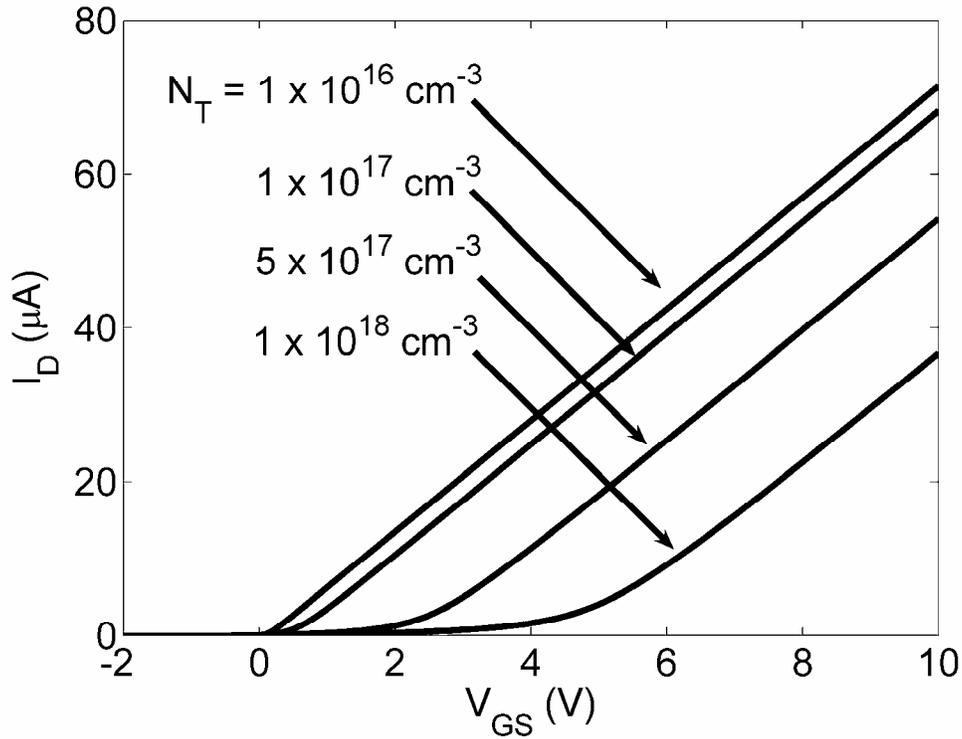
Figure 3.4: Drain current-gate voltage ( $I_D$ - $V_{GS}$ ) characteristics for an n-channel TFT corresponding to a drain voltage of 1 V and a trap depth of  $E_T - E_C = 0.15 \text{ eV}$ . Geometrical and channel-based parameters employed for this simulation are:  $Z/L = 6:1$ ,  $h = 20 \text{ nm}$ ,  $C_G = 6.04 \times 10^{-8} \text{ F/cm}^2$ ,  $\mu = 100 \text{ cm}^2/\text{V-s}$ , and  $n_{co} = 1 \times 10^{15} \text{ cm}^{-3}$ .
