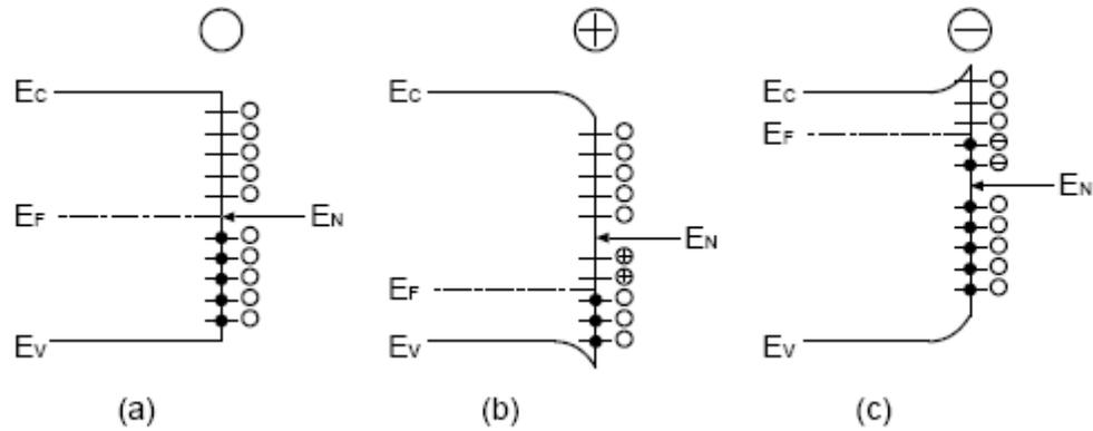
Figure 2.6: Energy band diagram considering interface states and the resultant effect of modulating the Fermi level position,  $E_F$ , with respect to the charge neutrality level,  $E_N$ . Three conditions are evaluated, (a)  $E_F = E_N$ , resulting in a flat-band condition, (b)  $E_F < E_N$ , resulting in a donor-like interface, and (c)  $E_F > E_N$ , resulting in an acceptor-like interface.
